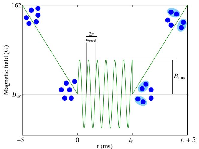
FIG. 1: (Color online) A schematic of the magnetic field sequence used in Ref. [16]. The ramps before and after the resonant pulse were shown not to create molecules. We assume a jump in  $B(t)$  at  $t_f$  when  $B(t_f) \neq B_{av}$ .
