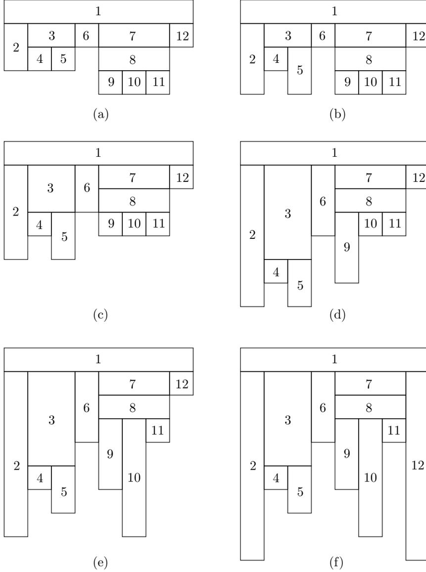
Fig. 4. Step 2: obtaining a 2-visibility drawing of  $G$  from the visibility drawing of  $T$  by ensuring the horizontal visibility between  $v_i$  and each node in  $B_2(v_i)$  for (a) nodes 3 and 4, (b) node 5, (c) nodes 6–8, (d) node 9, (e) node 10, and (f) nodes 11 and 12.
