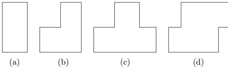
Fig. 2. Four types of modules required by He’s floor-planning algorithm [3]: (a) I-module, (b) L-module, (c) T-module, and (d) Z-module. Our algorithm does not need Z-modules.
