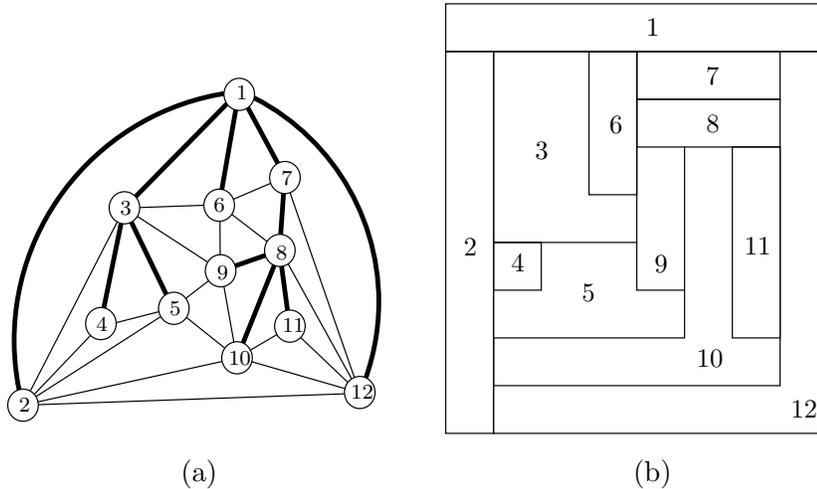
Fig. 1. (a) A plane triangulation  $G$ , where an orderly spanning tree  $T$  of  $G$  rooted at node 1 is drawn in dark. The node labels show the counterclockwise preordering of the nodes in  $T$ . (b) A floor-plan of  $G$ .
