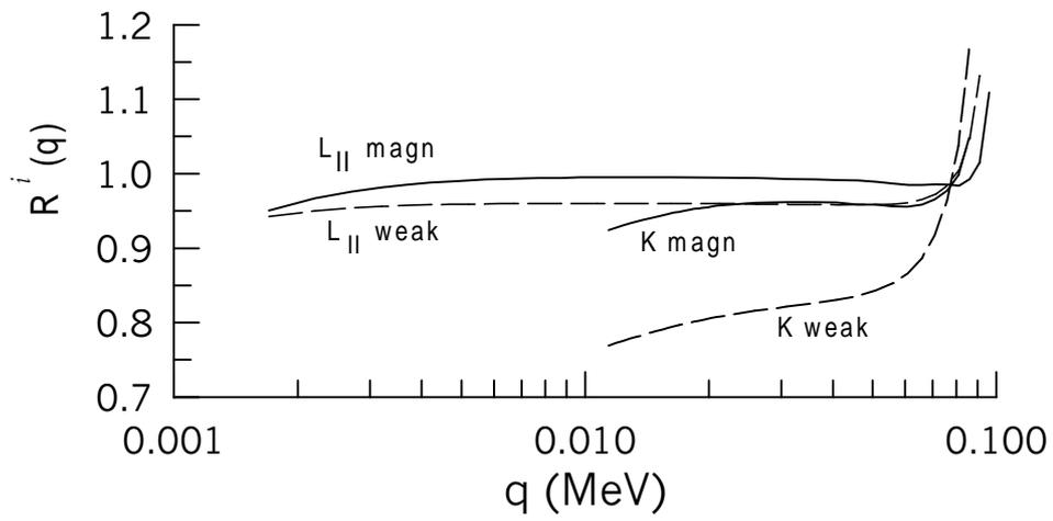
Fig. 9. "Exact" response functions for  $\bar{\nu}_e e^-$ -scattering on the germanium K- and L-shell electrons for the  $^{147}\text{Pm}$  source. The curves are marked with the corresponding subshells as in Table 1.
