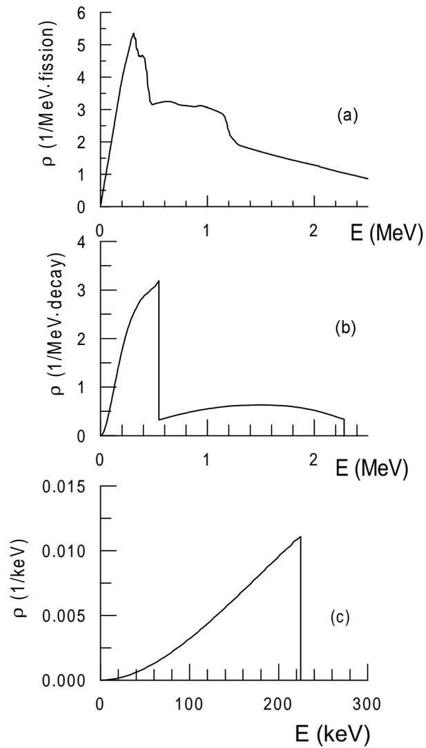
Fig. 1. Antineutrino energy spectra from three different sources: (a) reactor  $\bar{\nu}_e$  (only the low energy part is shown), (b)  $\bar{\nu}_e$ 's from the  $^{90}\text{Sr}$ - $^{90}\text{Y}$  source (two  $\bar{\nu}_e$ 's per sequential  $^{90}\text{Sr}$ - $^{90}\text{Y}$  decay), (c)  $\bar{\nu}_e$ 's from the  $^{147}\text{Pm}$  source.
