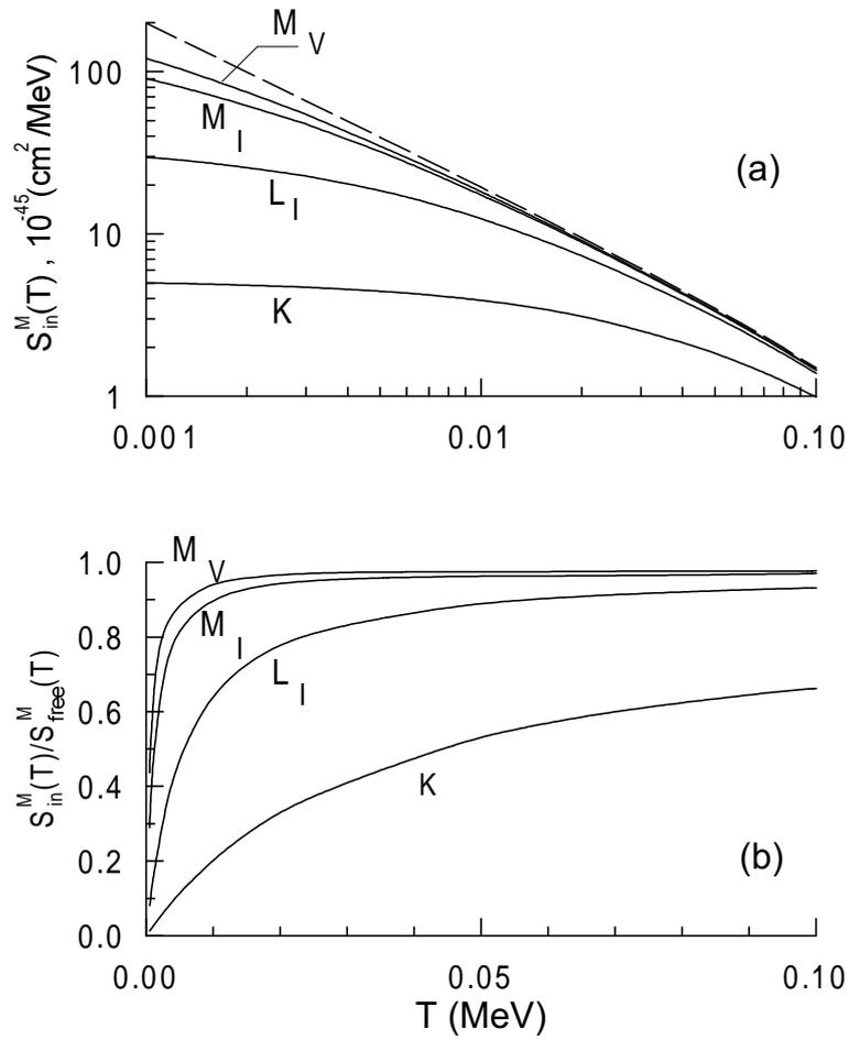
Fig. 3. Inelastic magnetic scattering of the  $^{90}\text{Sr}$ - $^{90}\text{Y}$  antineutrinos on the iodine atomic electrons vs electron kinetic energy. The curves correspond to the different subshells and are marked in the same way as in Table 1. (a) - electron kinetic energy spectra; dashed curve is for the scattering on free electrons ( $\mu = 2 \cdot 10^{-11} \mu_B$ ). (b) - ratios of the inelastic spectra to the free spectrum  $S_{\text{in}}^M(T)/S_{\text{free}}^M(T)$ .
