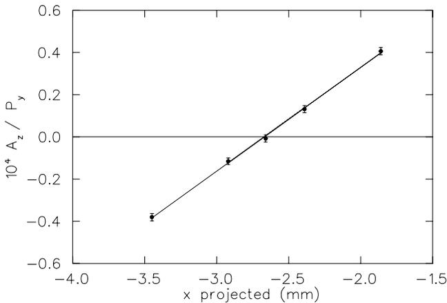
FIG. 12: A horizontal neutral axis scan. A vertically polarized beam ( $P_y = 0.76$ ) was scanned horizontally and the sensitivity to  $P_y$  plotted as a function of  $x$  projected to the “magic  $z$ ” ( $z$  location where the false  $A_z$  does not depend on angle). A beam with  $x_{proj} = -2.7$  mm was found to produce no false signal from vertical polarization components.
