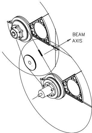
FIG. 4: Method of scanning the  $\text{CH}_2$  blades through the beam. The blades measure 5 mm x 1.6 mm in cross section and extend 85 mm beyond the holders. Each PPM has two horizontally scanning and two vertically scanning blades. This figure shows a blade at the middle of a vertical scan.
