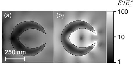
FIG. 4: Local magnitude of the electric field, calculated for a 2D geometry of silver in vacuum for light incident from the left with wavelength  $\lambda_{UV} = 250$  nm (a) and  $\lambda_l = 400$  nm (b). The gray scale bar indicates the enhancement factor of the squared field amplitude
