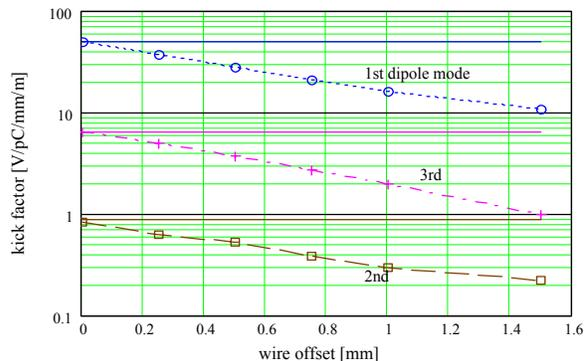
Figure 6 Kick factors of the first 3 dipole synchronous modes of cell 198 of DS2 with a wire 250  $\mu\text{m}$  in diameter placed parallel to the axis, as a function of the wire offset displacement system envisaged is straightforward, and does not cause unnecessary spurious mode excitation.
