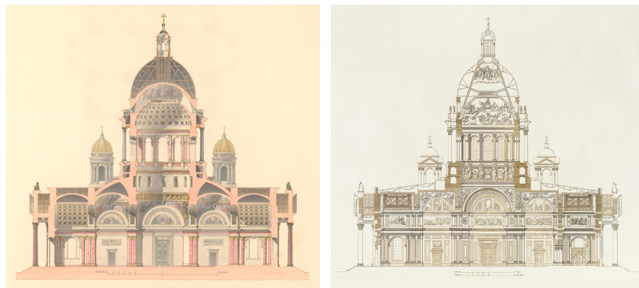
Figure 3, 4: St. Isaac’s Cathedral with masonry and wooden dome, 1818/1825/1828 (Montferrand 1828, table 4); design conversion to iron dome structure, 1838 (Montferrand 1845, table 26)
