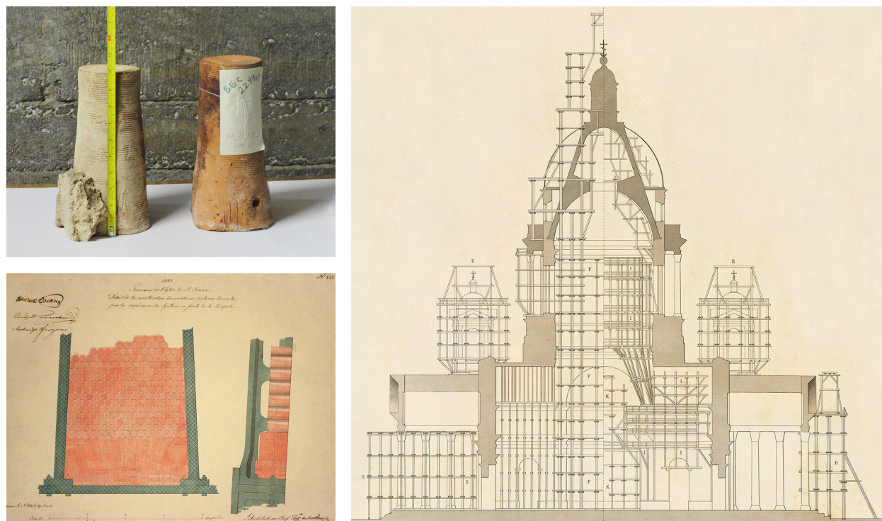
Figure 6: Scaffolding for erecting the iron dome and installing the ceramic pots (Montferrand 1845, table 32-33). Figure 7 (a, b): Ceramic pots and masonry in the ribbed dome structure: (a) placement (NTB RGUPS, FM 4-233), (b) view of the pots, 250 mm in height on bases of 100 and 135 mm, and weighing 2.20 to 2.60 kg, each (Fedorov)
