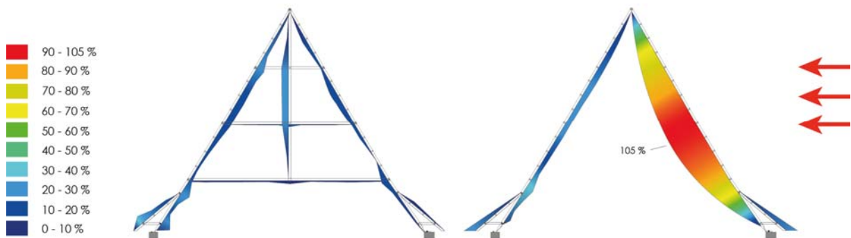
Figure 11: A pair of rafters (with and without collars) subjected to dead and wind loads: utilization in terms of effective stress (according to Batke 2015)
