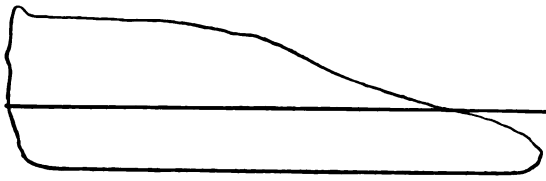
INDICATOR DIAGRAM OF FRENCH SCREW STEAMER "FAON."
