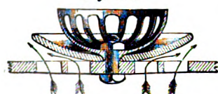
MAUDSLAY'S DISC VALVE FOR AIR PUMP.
