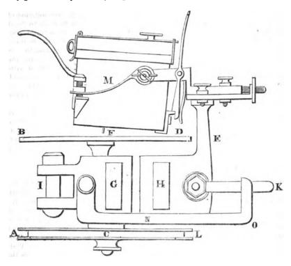
IGN O and EHK in the figure represent two separate pieces, which may be made to move upon one another in the directions HK and GI. Two springs shackled together at their extremities, and represented in a subsequent figure, are severally inserted in the apertures G and H, and fixed there by their middle points.
