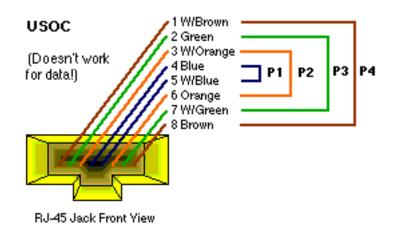
Figure 1.2 clearly shows the large difference between this and the other two standards. Note how the pairs are nested inside each other.
