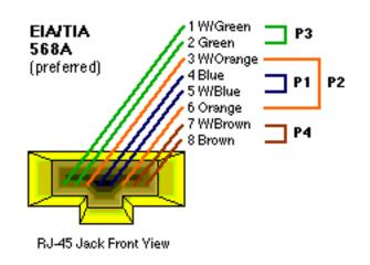
Figure 1.0 shows how the TIA/EIA 568A standard is to be terminated. Note the position of the green/white green and the orange/white orange pairs.
