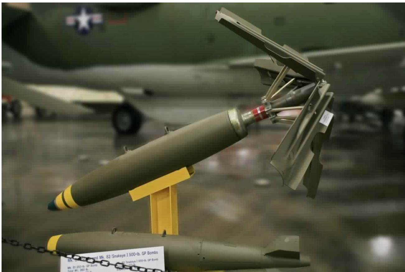
Mk. 81 bomb with Tail Retarding Device "Snakeye"
