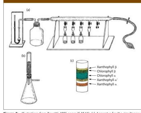
**Figure 2:** Illustrations from Tswett's 1906 paper (6,10,11). (a) Apparatus for the simultaneous use of as many as five columns. The lower part of the small funnel-like glass pieces (2–3 mm i.d. and 20–30 mm length) served as the packed column. (b) Apparatus for larger samples (1–3 cm i.d., packing length: 5–9 cm). (c) Chromatographic separation of plant pigments as drawn by Tswett. Stationary phase: calcium carbonate; eluent: carbon disulfide.
