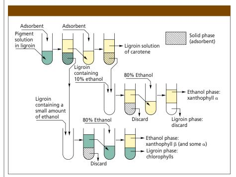
**Figure 1:** Separation scheme of the stepwise differential adsorptive precipitation and extraction method, used by Tswett in his early work. Drawn after the description in (4).
