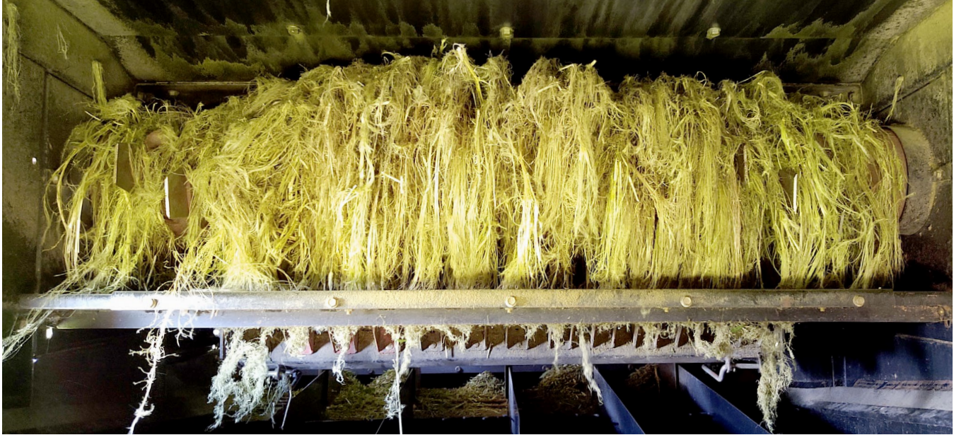
FIGURE 5. Fibers wrapped around the straw chopper rotor at the exit of the threshing rotor when operated at the low speed setting. Increasing the speed from low to high eliminated this issue.
