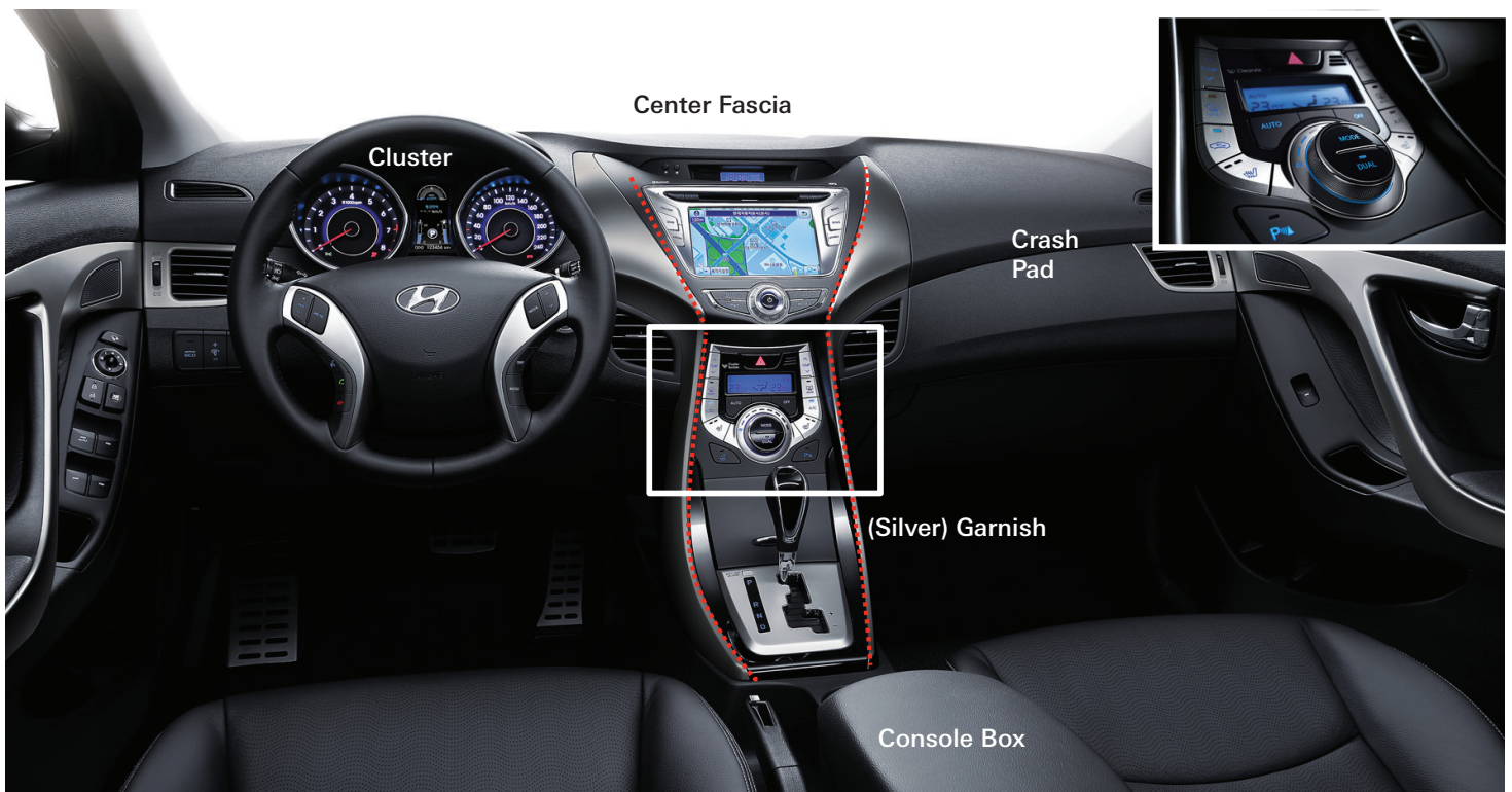
FIGURE 7. The interior design of the 2010 Elantra, featuring a center fascia with a silver garnish. Inset: the control knob for fan and temperature.
