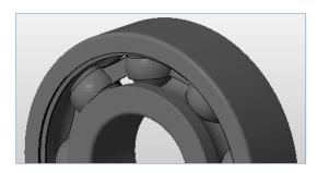
Example model design of an all-inone assembly with moving parts
