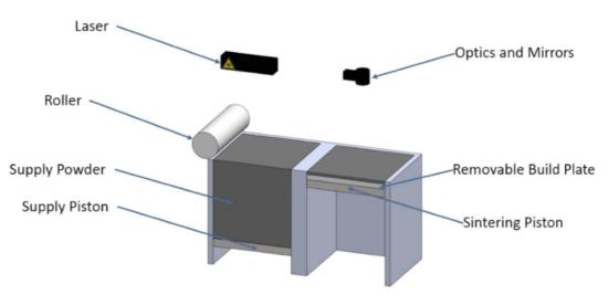
Typical components of a DMLS machine
