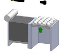
**Part Removal**: Sinter piston raises up, allowing the build plate to be removed.
