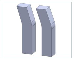
*Example of warping on a tall, thin part without support structures*
