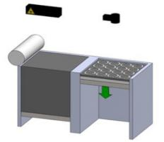
**Piston Movement**: Sinter piston moves down the thickness of one layer.
