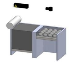
**Layering**: The process is repeated until the parts are fully sintered.
