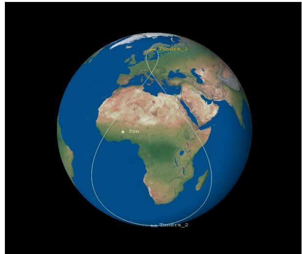
Figure 2. Two-satellite Tundra constellation: ground trace of the orbits.
