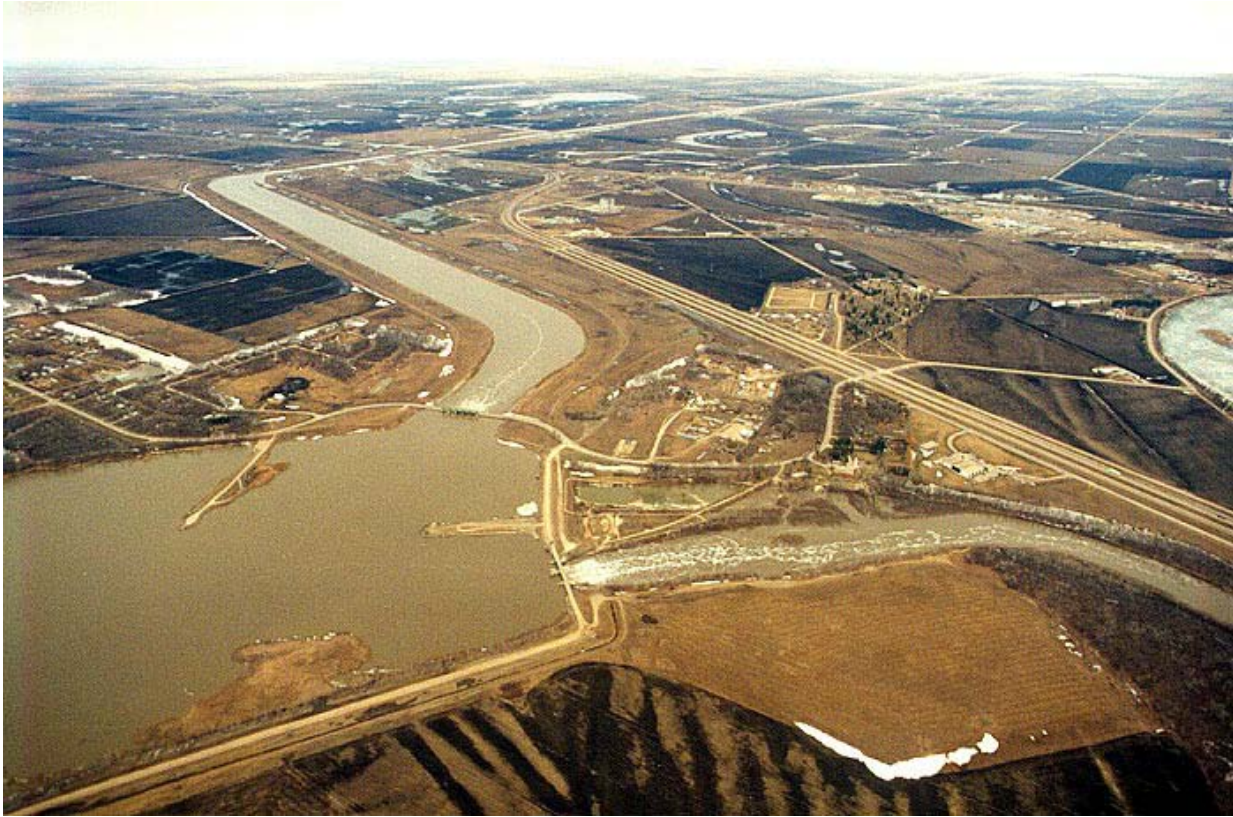
Figure 29: An aerial photograph of the Portage Diversion during a flood event; the year is unknown. The Portage Reservoir is visible on the left edge of the photo, the diversion channel continues northward into the background of the photo, and the Assiniboine River flows off the right hand edge of the photo. Of note, a portion of the Blind (or Fort la Reine) paleochannel is visible downstream of the control structure on the river, running north from the highway into the background.
