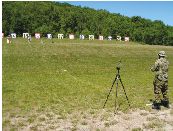
Figure 2: Measurement positions of the C7 rifle noise at CFB Meaford (top), and photo of the range environment (bottom). Microphones were placed close to the shooter and on tripods at 4 m increments. The grass-covered ground surface is partially sound-absorbent, and there are no reflective surfaces near the weapon.
