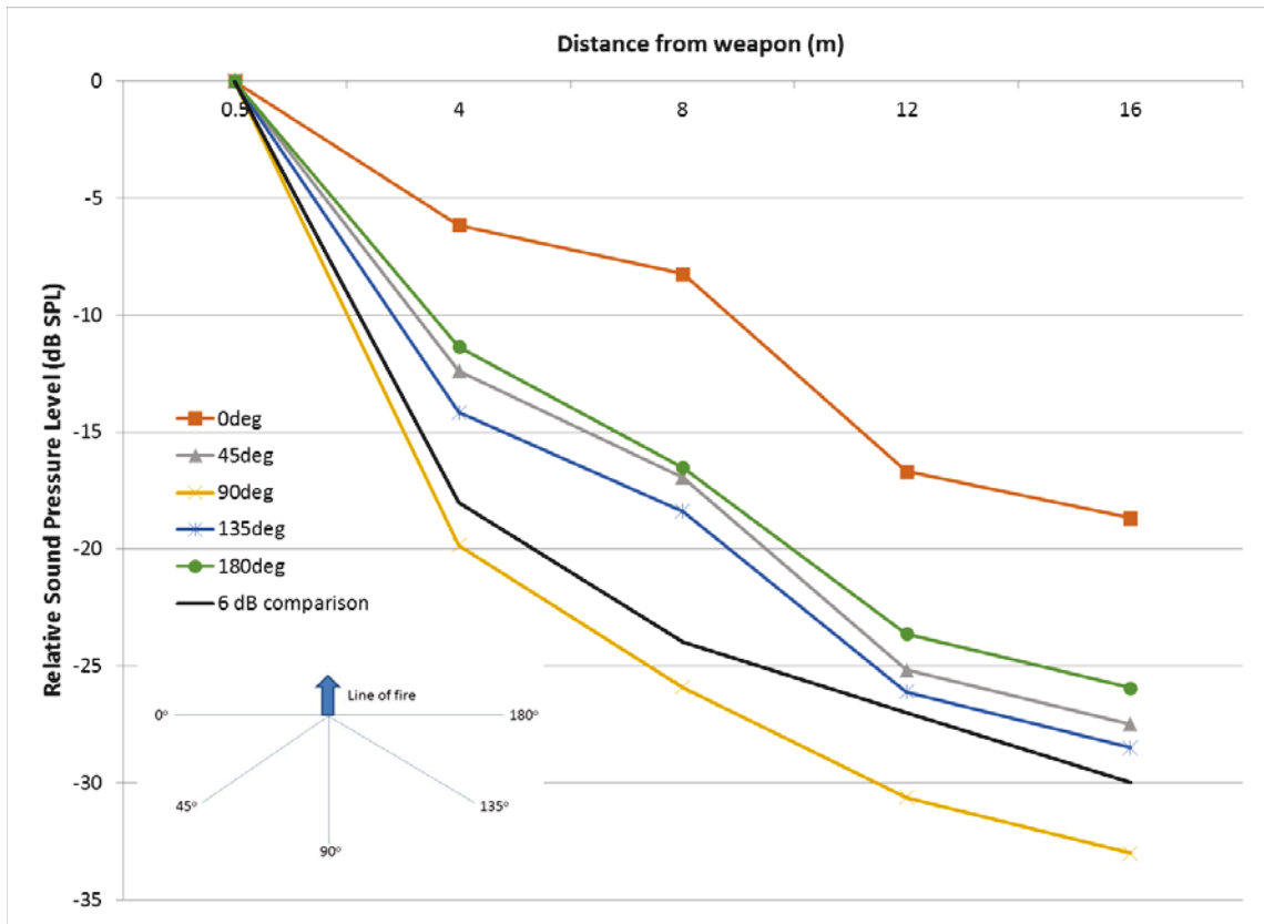
Figure 5: Unweighted peak sound pressure levels behind the weapon, relative to the closest point of measurement (shown as 0.5m). The data shown are the averages for C8 suppressed and unsuppressed, C14 suppressed, C15 suppressed and C16. The 6 dB reduction with doubling of distance is shown for reference (black line).
