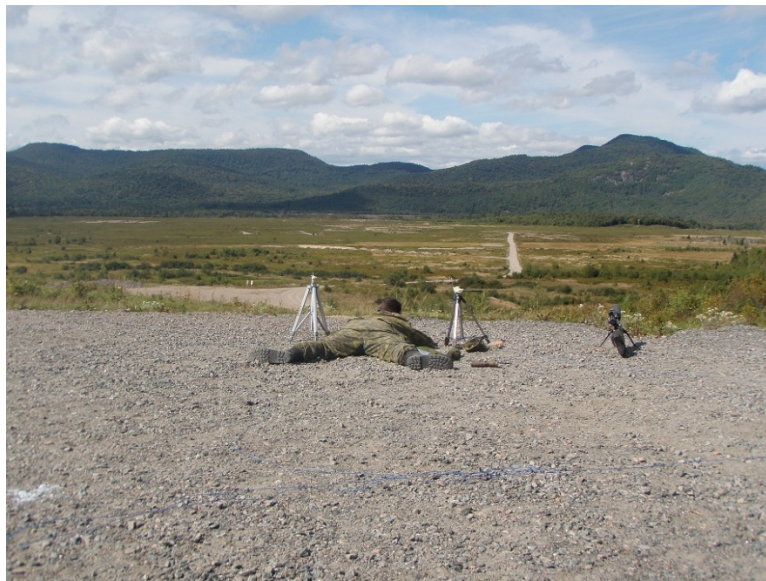
Figure 3: Measurement positions of the C8, C14, C15 and C16 weapon noise at CFB Valcartier (top), and photo of the range environment (bottom). Microphones were placed close to the shooter and on tripods at 4 m increments. The gravel-covered ground surface is partially sound-absorbent, and there are no reflective surfaces near the weapon.
