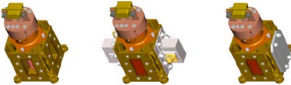
Figure 2-6. Waveguide transfer switches used on Dawn.
