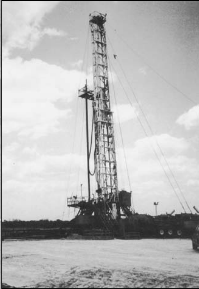
A drilling rig with several stands of drill pipe in the derrick
