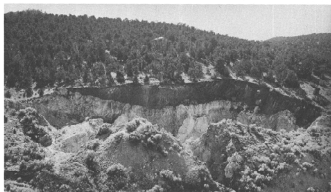
Figure 2. Southwestward view of Harding quarry from North Knob, showing the sharp, irregular hanging wall of the main pegmatite body as exposed by open-cut mining prior to 1943. The body dips gently away from the observer, and its footwall is exposed near portal of main entry in right foreground. Active workings for microlite ore are at left in quarry, beyond the northeast entry. Temporary structure of U.S. Bureau of Mines camp appears on the wooded slope in center distance.
