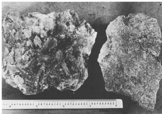
Figure 7. Specimens of lithium-tantalum ore from main quarry. At left is a variety of "spotted rock" in which patches of coarse microcline are outlined by small, dark-colored crystals of lepidolite, tantalite-columbite, and uranian microlite-pyrochlore. The microcline is partly replaced by minute scales of lepidolite, which also are abundant in remainder of the rock. At right is an aggregate of spodumene laths and plates, most of them much corroded, in a matrix of purple lepidolite (dark), albite, and quartz with scattered small crystals of tantalum-niobium minerals.
