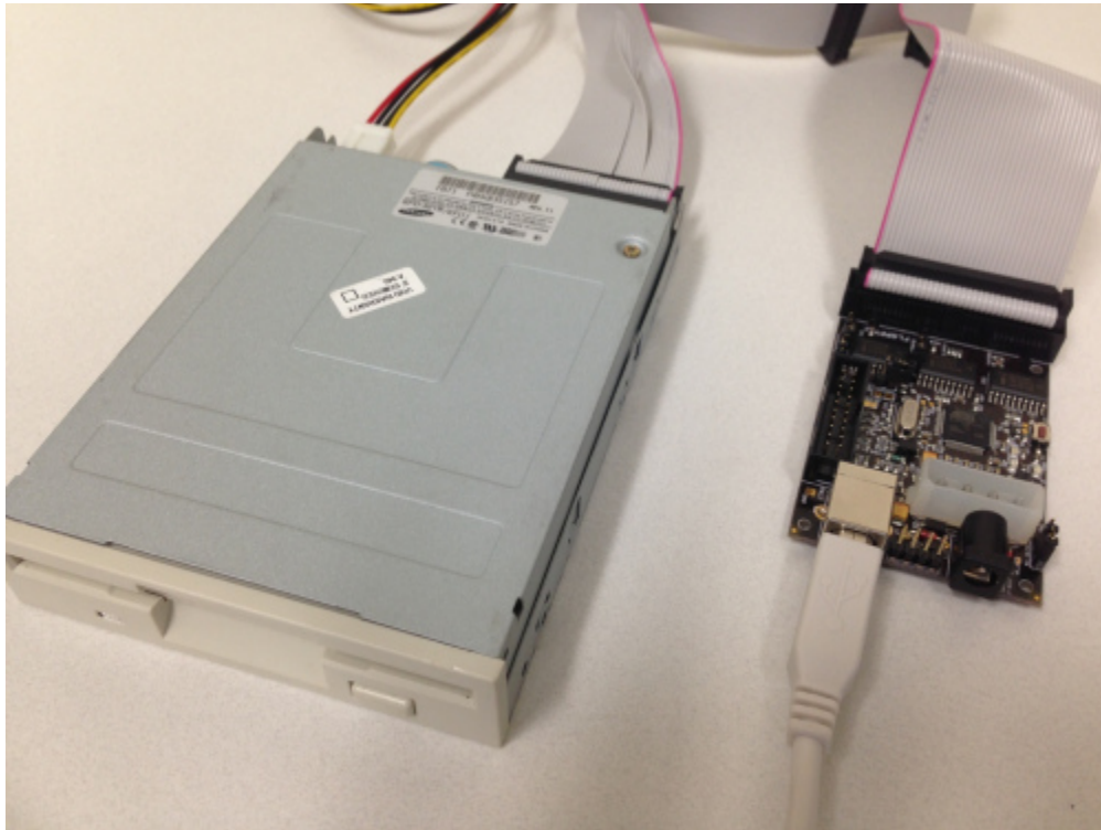
Figure 4: The KryoFlux connects to a 3.5" floppy disk drive and captures forensic images of disks in a variety of formats.
