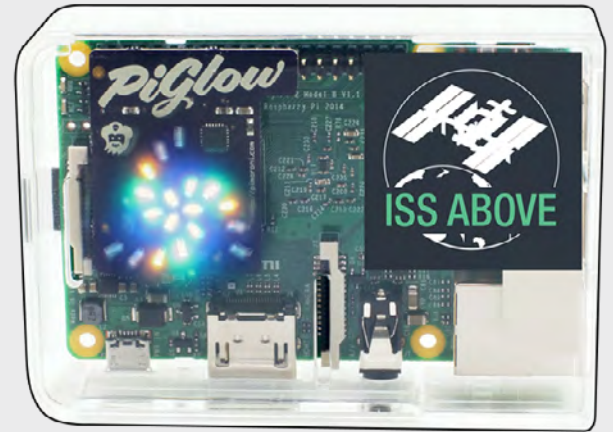
Figure 16 An ISS-Above unit, with lights indicating when the space station passes overhead. (Photo courtesy of ISS-Above)
