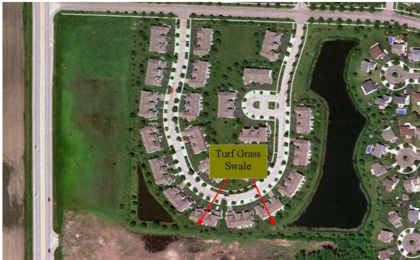
Figure 4-12. Kimball Farms Detention Basin # 1 contains a large east basin and a small west basin that are separated by an overland flow swale to the south. The east basin also contains a substantial area of shoreline that is eroding.
