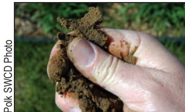
A ribbon test used to estimate clay content.
