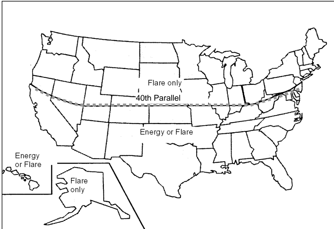
Figure 3. Covered lagoons - locations suitable for biogas to energy conversion generally fall below the 40th parallel.
