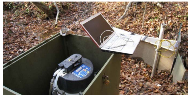
ISCO sampler collecting water quality data. A sampler like is currently being used for water quality monitoring by NGRREC in the Upper Silver Creek watershed. Photo: University of Delaware.
