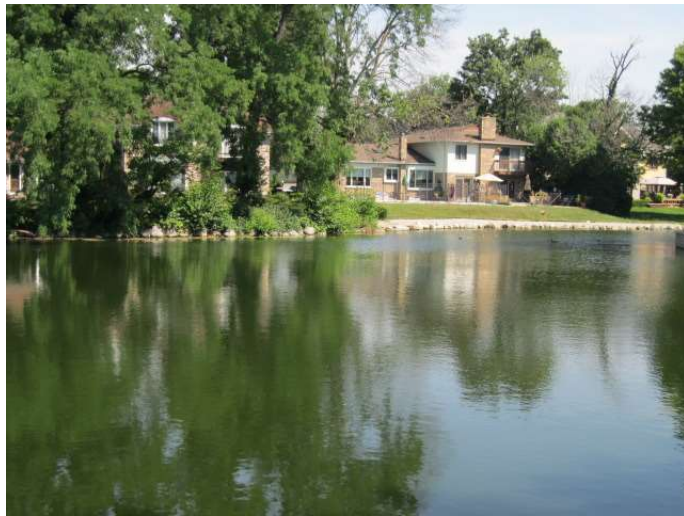
Photos 83 and 84: An unnamed lake (Basin 1-B) with residential areas along the shoreline contains extensive turf grasses at the shoreline with a variety of shoreline stabilization treatments ranging from retaining wall, to rip-rap, to re-shaped turf slopes. It is likely that turf grass pollutant runoff contributed to algae blooms that appear to be present.
