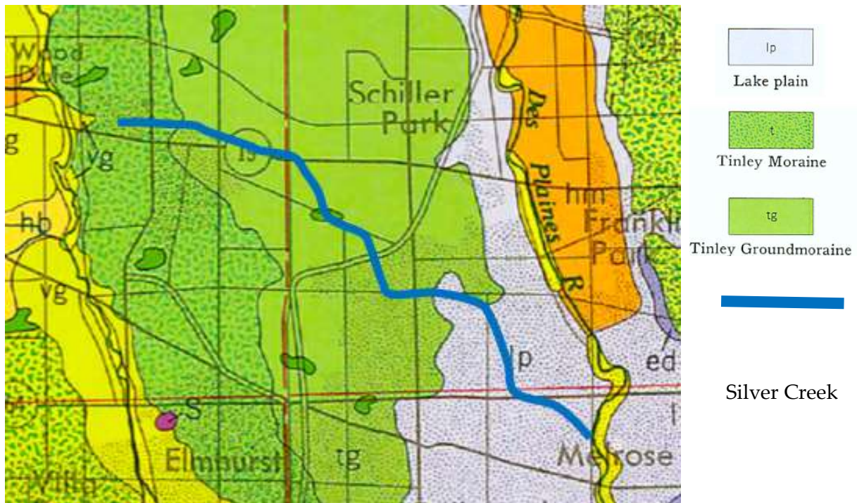
Fig. 4: Surface Geology includes lake plain (lp) to the east, and Tinley Moraine (t) / Tinley Groundmoraine (tg) to the central and west watershed areas (Willman, 1971).
