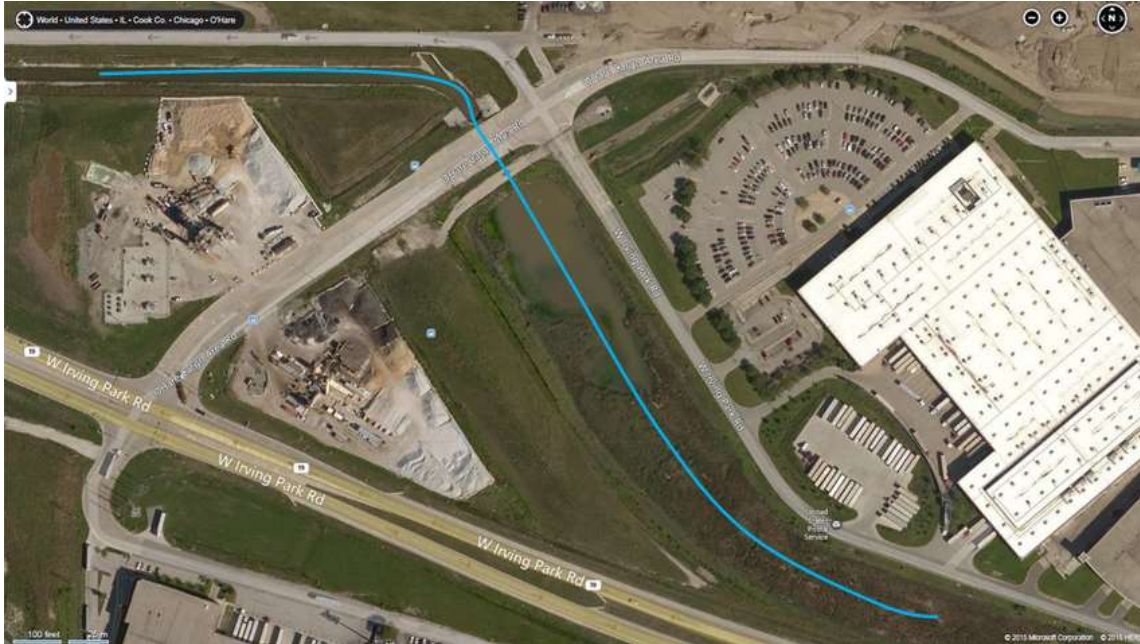
Exhibit 2: Silver Creek in Reach # 6 was converted into a broad, shallow detention area with extensive adjacent emergent wetland dominated by cattails. It is assumed that maximized flood storage capacity is a primary purpose for the broad configuration of this detention area.
