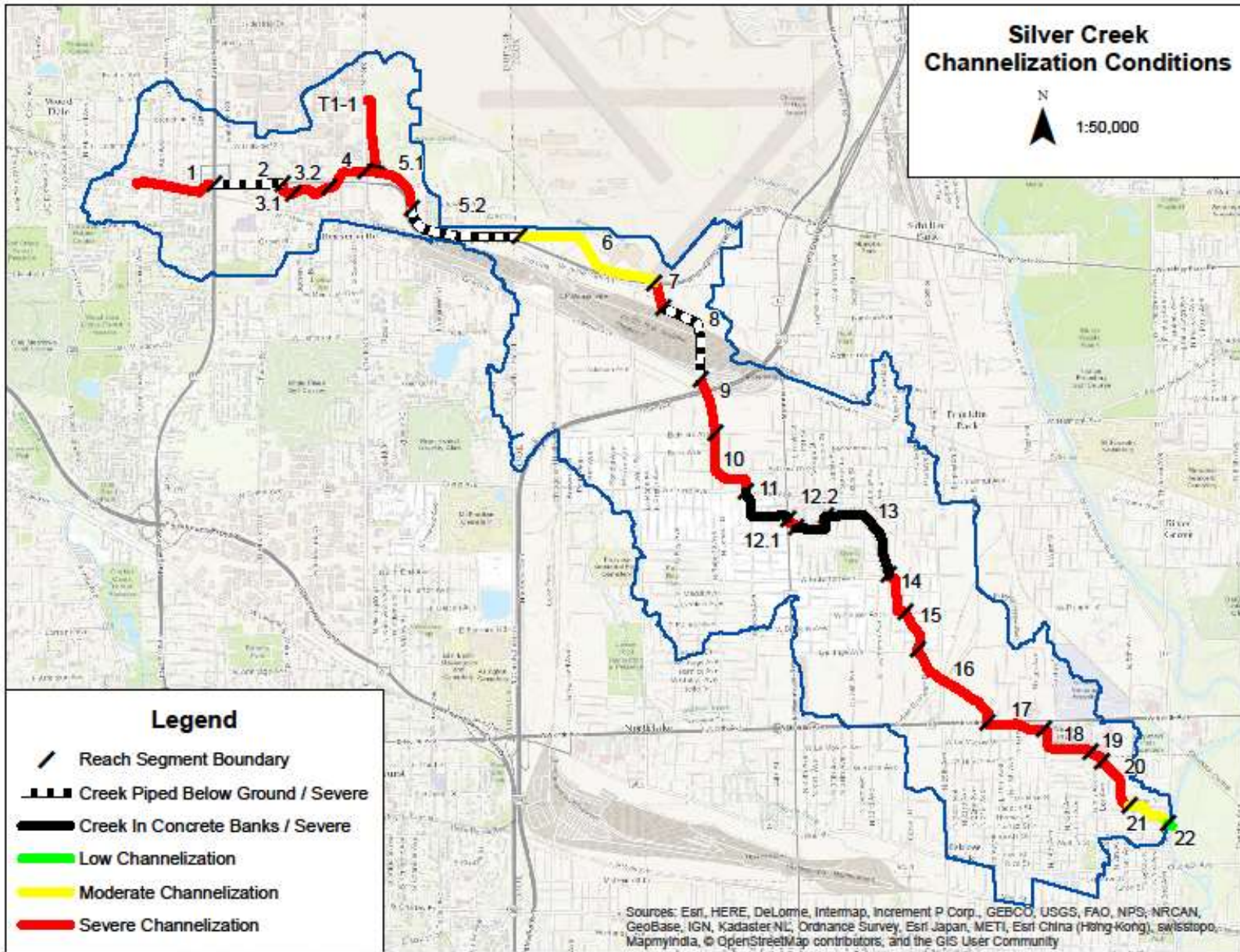
Fig. 22: Silver Creek Stream Reach Channelization Conditions.
