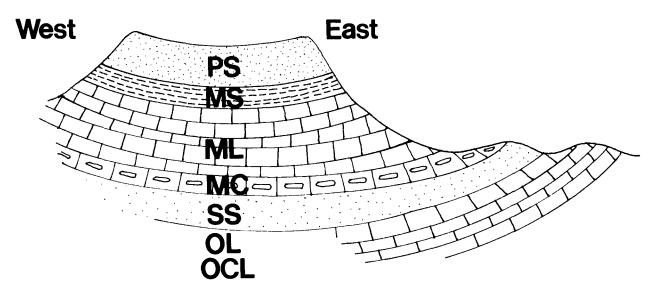
Fig. 22. Diagrammatic cross section of Lookout Mountain and associated ridges (looking north). Adjacent low hills are in Red Mountain Sandstone (SS) and Knox Dolomite (OCL). PS Pennsylvanian sandstones, MS Mississippian shales, ML Mississippian limestones, MC Mississippian chert (Fort Payne chert), SS Silurian sandstones, OL Ordovician limestones, OCL Ordovician - Cambrian limestones. After Cressler (1964) and S. Pickering (pers. comm.).
