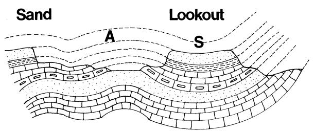
Fig. 23. Diagrammatic cross section of Sand and Lookout mountains depicting the eroded anticlines (A) as valleys and the former synclinal valleys (S) as ridges (looking north). After Sullivan (1942).
