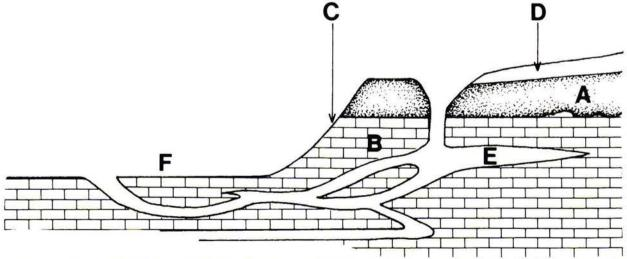
Fig. 29. Solution ravine and limesink on the Pelham Escarpment, SW Georgia. (A) Miocene Hawthorne clastics on the western edge of the Tifton Upland; (B) Miocene and Oligocene limestones; (C) Pelham scarp face; (D) ravine emptying into sink; (E) underground cavern such as Climax Cave; (F) Dougherty Plain (Limesink Region) surface. Steepness of scarp face is greatly exaggerated.
