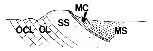
Fig. 20. Diagrammatic cross section of Taylor's Ridge at Summerville (looking north), Bulk of ridge is formed by Silurian sandstone (Red Mountain Formation). Cliffs of the eastern side are formed in chert beds of Silurian (Armuchee Chert) and Mississippian (Fort Payne Chert) age. MS Mississippian Shale (Floyd Shale), MC Mississippian chert, SS Silurian sandstone, OL Ordovician limestones, OCL Ordovician-Cambrian limestones. After Cressler (1974).
