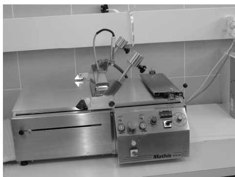
Figure 2. Coating equipment used in the production of the surface sized samples.
