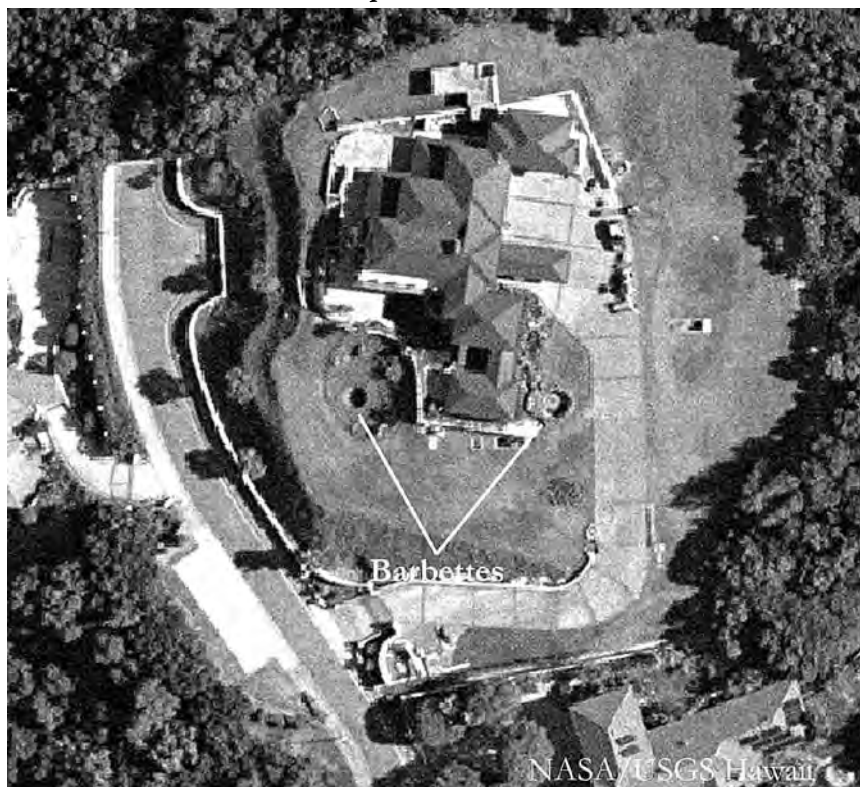
Large mansion constructed over the remains of Battery Wilridge (Kirkpatrick). Arrows point to existing steel barbettes of both turrets. USGS
