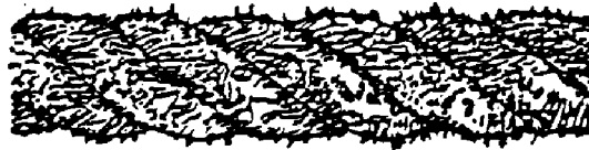
Figure 613-2-33. Synthetic Rope Showing Fuzzy Nap as a Result of Normal Wear
