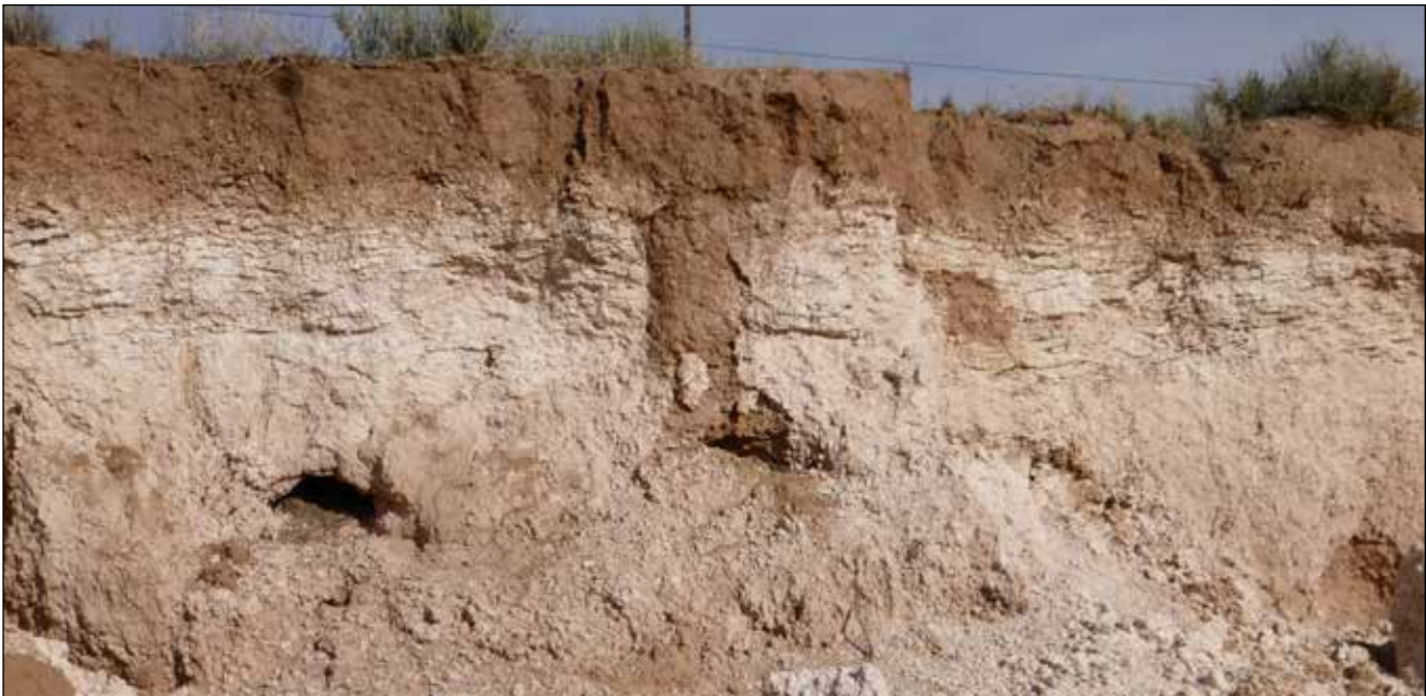
Figure 19. Borrow pit near Engle showing well developed horizontally fractured white carbonate horizons just below the reddish brown eolian deposits at the surface.
