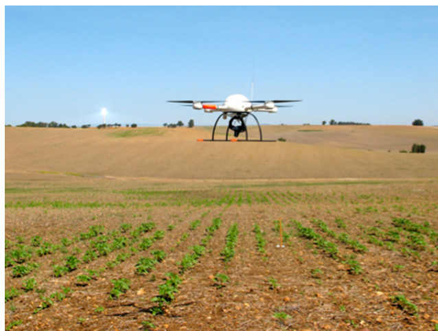
Fig. 5 Cost and availability of imaging spectroscopy data could be improved using an Unmanned Aerial Vehicle (UAV) remote sensing system. The md4-1000 UAV used by Torres-Sánchez et al. (2013) can carry any sensor weighing less than 1.25 kg. For evaluation of weed infestation, it was equipped with a still point-and-shoot camera and a six-band multispectral camera (courtesy of Public Library of Science)
