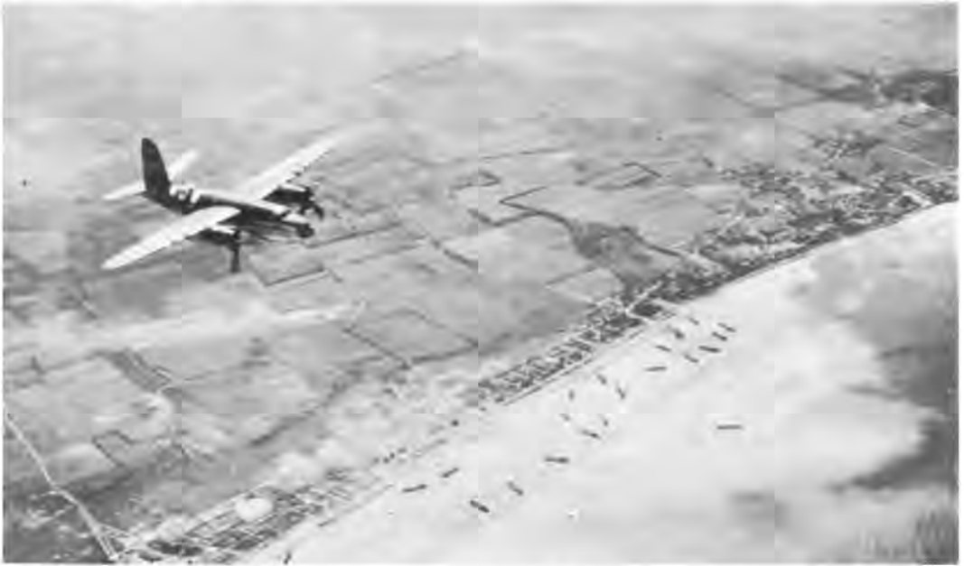
NINTH AIR FORCE B-26 OVER BRITISH BEACHHEAD at Lion-sur-Mer. Note markings on plane. All Allied aircraft, except 4-engine bombers, in support of the invasion were painted thus for purposes of identification. Two black and three white stripes were painted on wings and around the fuselages.
