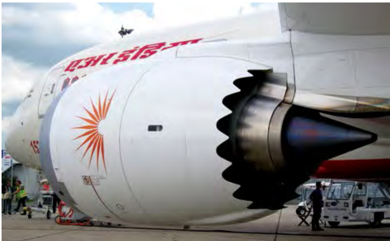
Image 345: GENx engine with a chevron nozzle on an Air India Boeing 787 Dreamliner. By Oliver Cleynen (own work) [cc BY-SA 3.0 ( http://creativecommons.org/licenses/by-sa/3.0 )], via Wikimedia Commons.
