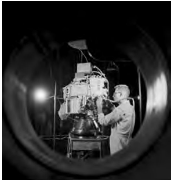
Image 194: Space Electric Rocket Test I ( SERT-I ) spacecraft and thrusters tested in EPL's Tank No. 3 in June 1964 (GRC-1964-C-70258).
