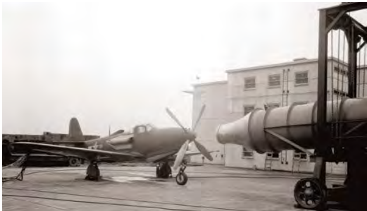
Image 70: A P-38J Lightning in front of the blower on the hangar apron that was utilized as a crude rain-simulating device. The blower was used extensively during the 1940s to supplement wind tunnel and flight research data (GRC-1945-C-09650).
