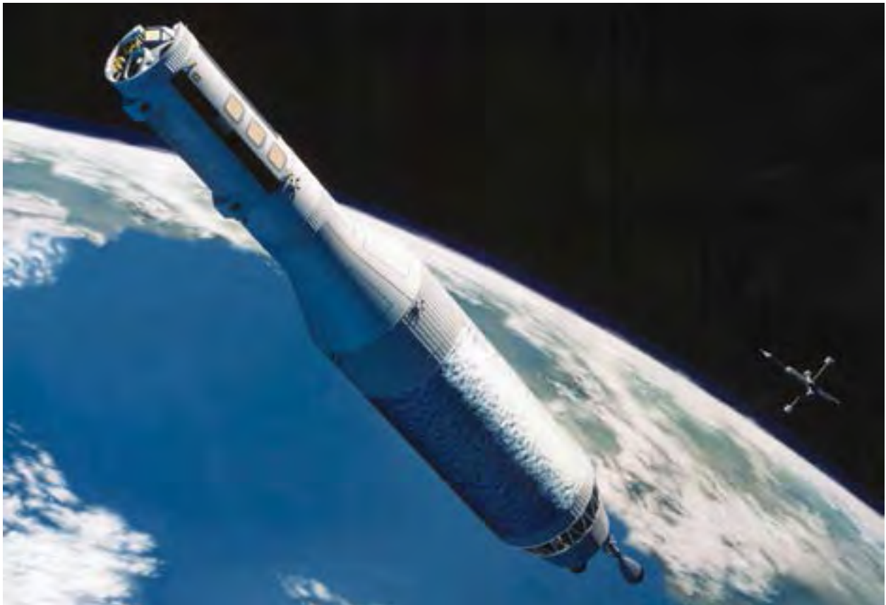
Image 317: Conceptual drawing of a lunar-oxygen-augmented nuclear thermal rocket (NTR) (GRC-1997-C-00827).
