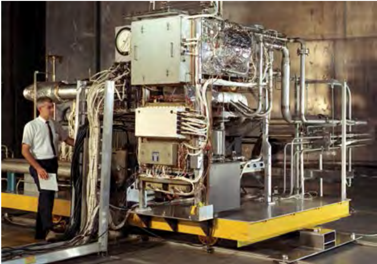
Image 238: Brayton system setup in the SPF prior to the installation of the space radiator. The tests, which began in September 1969, were the first ever conducted in the new vacuum tank at Plum Brook Station (GRC-1970-C-01966).
