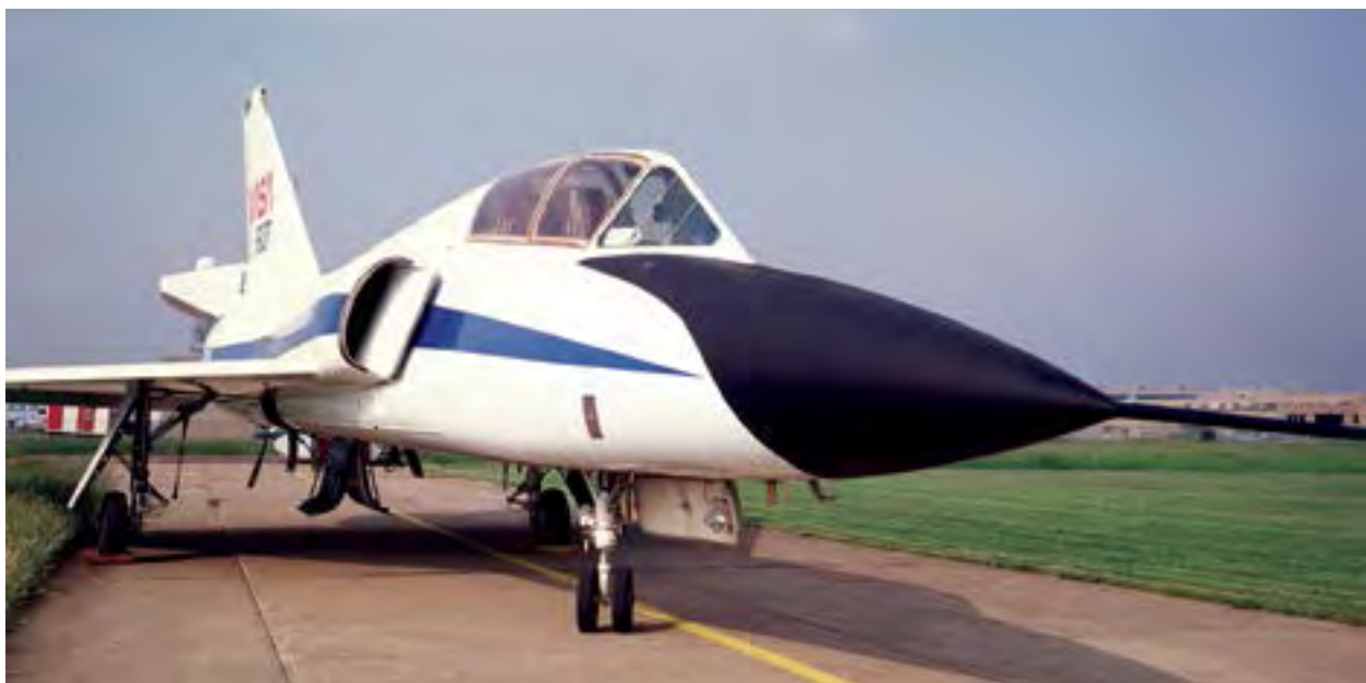
Image 253: NASA's F-106B Delta Dart was acquired as the chase plane for the center's first F-106B. After that program ended, the chase plane was equipped with air-sampling and ocean-scanning equipment and performed remote sensing throughout the 1970s. The ocean-scanning equipment was stored in the nose section of the F-106B (GRC-1979-C-02423).
