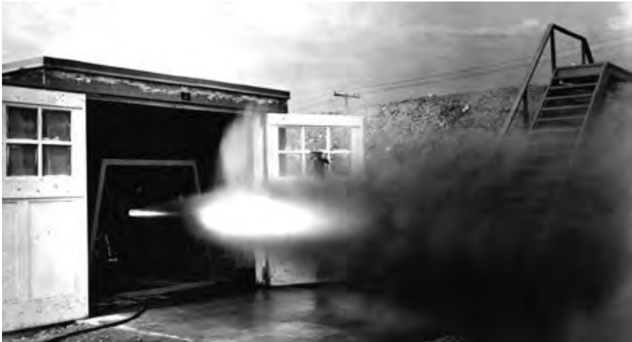
Image 120: Firing of a nitric acid aniline JATO rocket at the Rocket Lab in March 1946. The Rocket Lab was expanded over the next 10 years and eventually included its own hydrogen liquefier (GRC-1946-C-14478).
