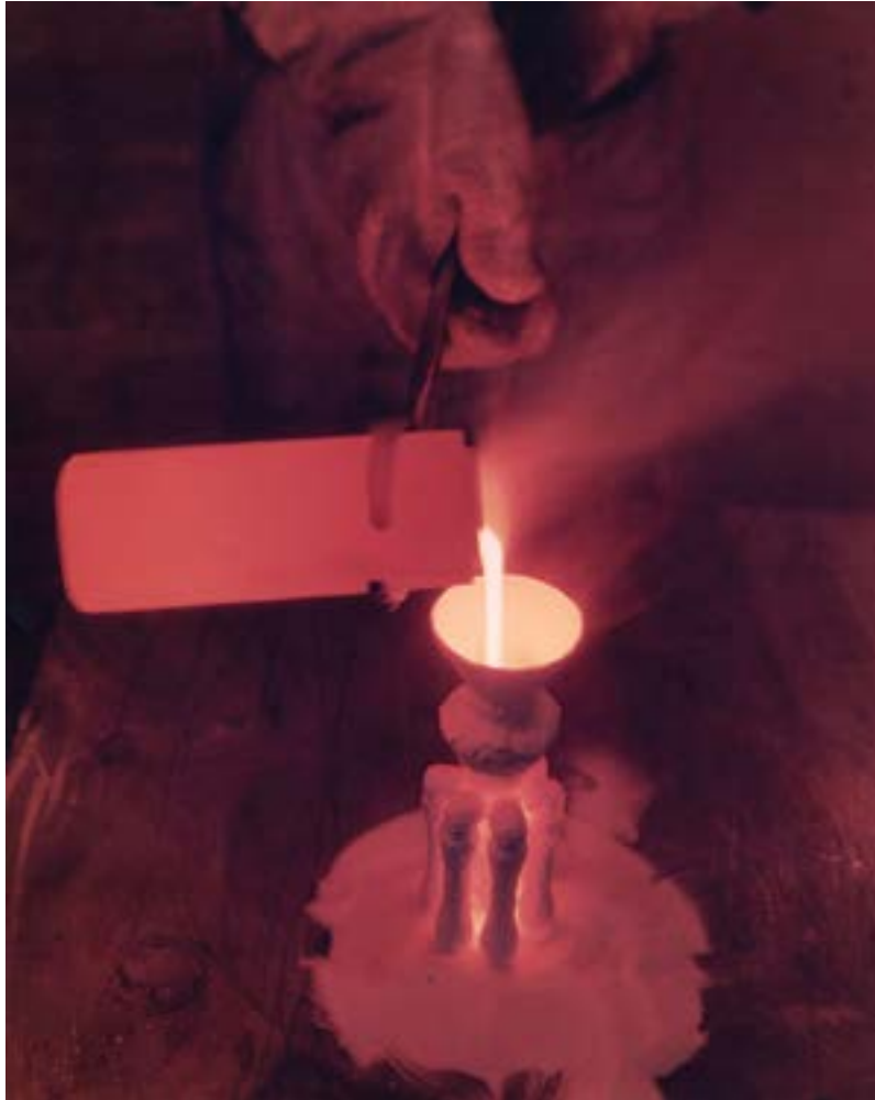
Image 220: Pouring of a nickel alloy at Lewis's Technical Services Building in April 1966 (GRC-1966-C-01563).
