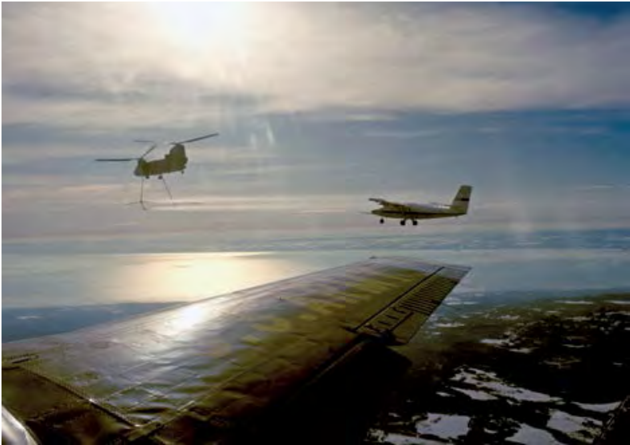
Image 301: The Twin Otter performs an inflight icing test in Duluth, Minnesota, while a Sikorsky helicopter trails water vapor to simulate icing clouds (GRC-1988-C-01727).
