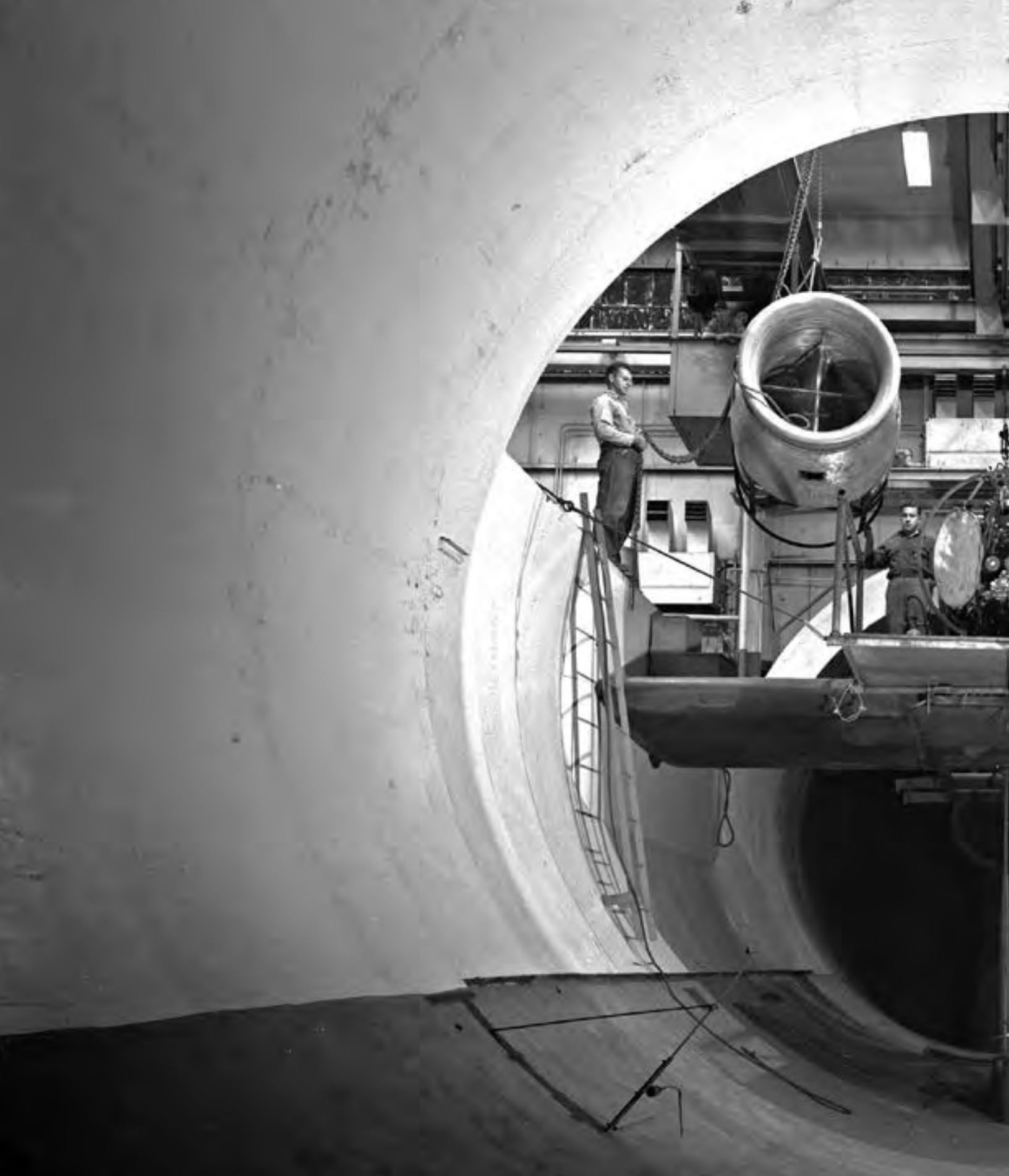
Image 79: Mechanics lower an inlet duct for a Westinghouse J40 engine into the Altitude Wind Tunnel's 20-foot-diameter test section (GRC-1951-C-28463).
