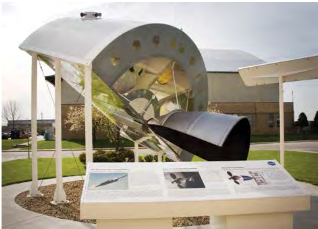
Image 376: While NASA was still defining the Constellation mission and parameters, Glenn sought ways to participate in the program. In 2005 Glenn teamed with Marshall to design the Orion service module mock-up. The Glenn Fabrication Shop then created an 18-foot-diameter full-scale model with a 180° cutaway highlighting the module's internal components. 1160,1161 Ever since, it has been on display next to the Administration Building (GRC-2007-C-00566).
