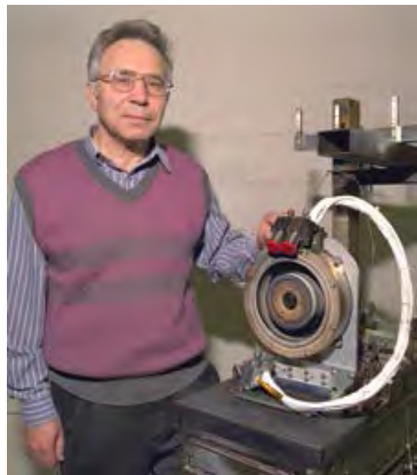
Image 372: Ivanovich Anatoli Vassine poses with a Russian T-160E Hall thruster being tested at the center in November 1997 (GRC-1997-C-04095).
