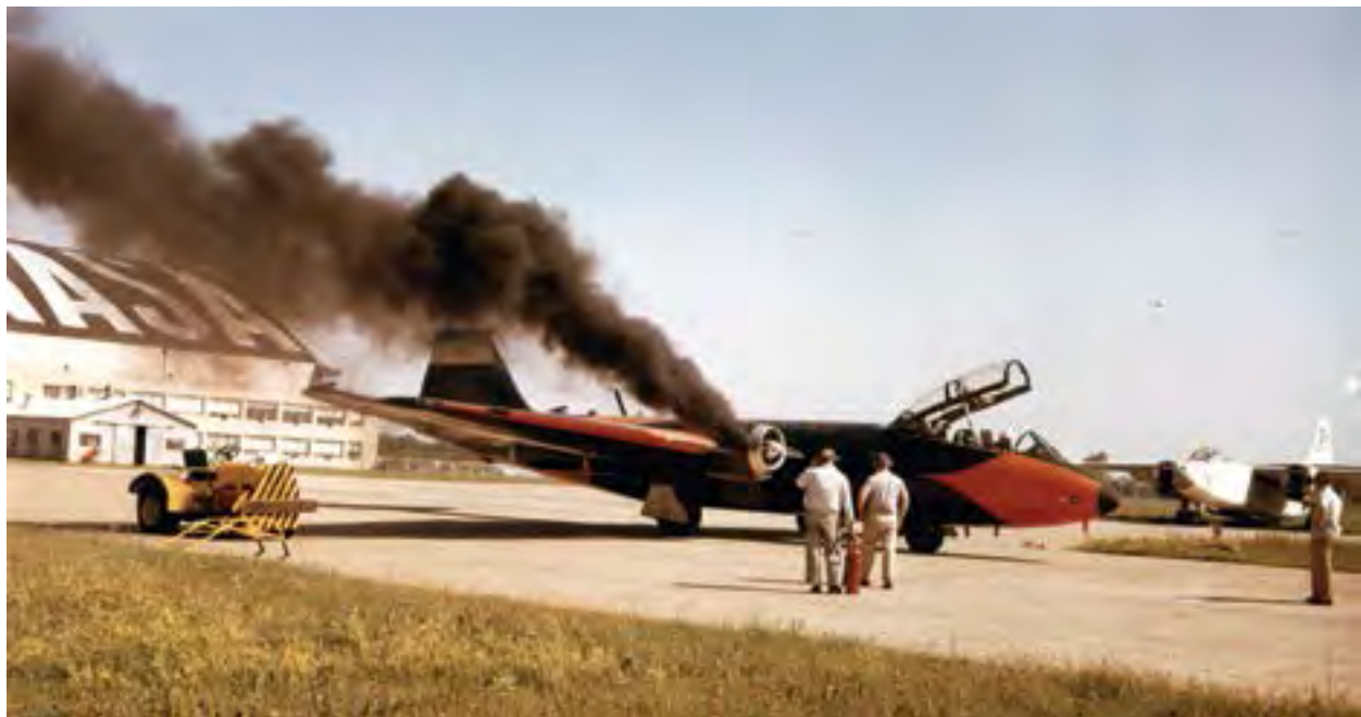
Image 158: As a converted B-57B prepares for a liquid-hydrogen flight over Lake Erie, black smoke emanates from the jet-fuel-powered engine. The hydrogen engine left a pronounced white contrail (GRC-1993-C-05546).
