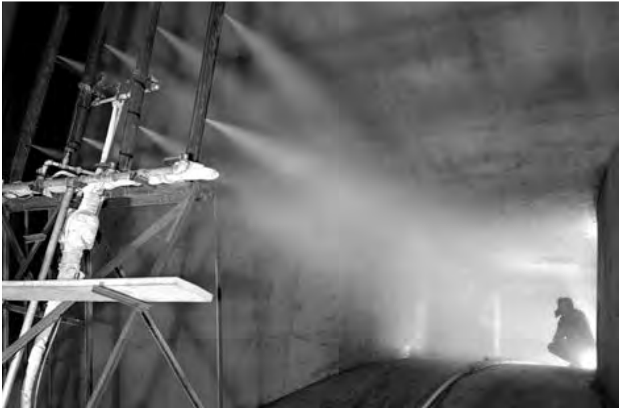
Image 137: After years of experimentation, Lewis engineers finally perfected the IRT's spray bar system in 1949 (GRC-1949-C-24017).
