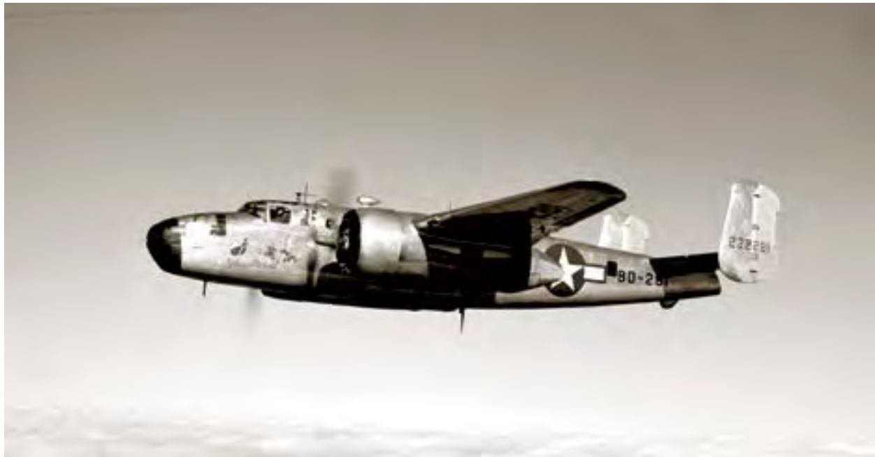
Image 104: The XB-25E Mitchell searches for icing clouds in January 1947. The aircraft, dubbed "Flamin' Mamie," includes nose artwork depicting a fiery woman chasing off icing researchers (GRC-1947-C-17763).
