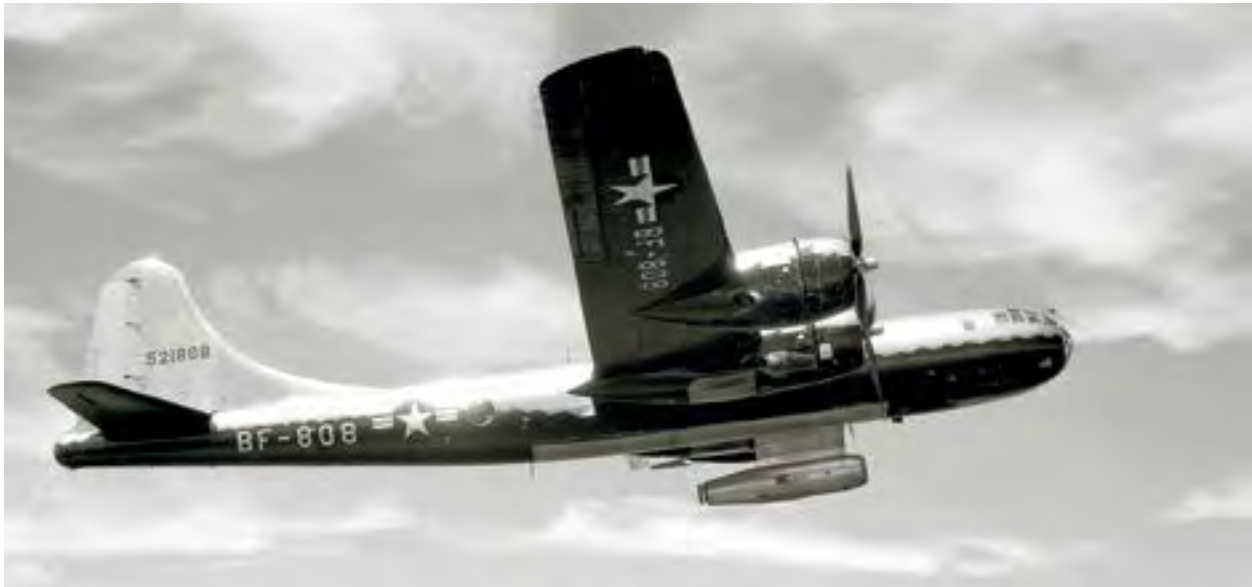
Image 115: A B-29 bomber that was modified to serve as a ramjet testbed for Lewis researchers. The experimental ramjet was lowered from the bomb bay and fired (GRC-1948-C-21990).
