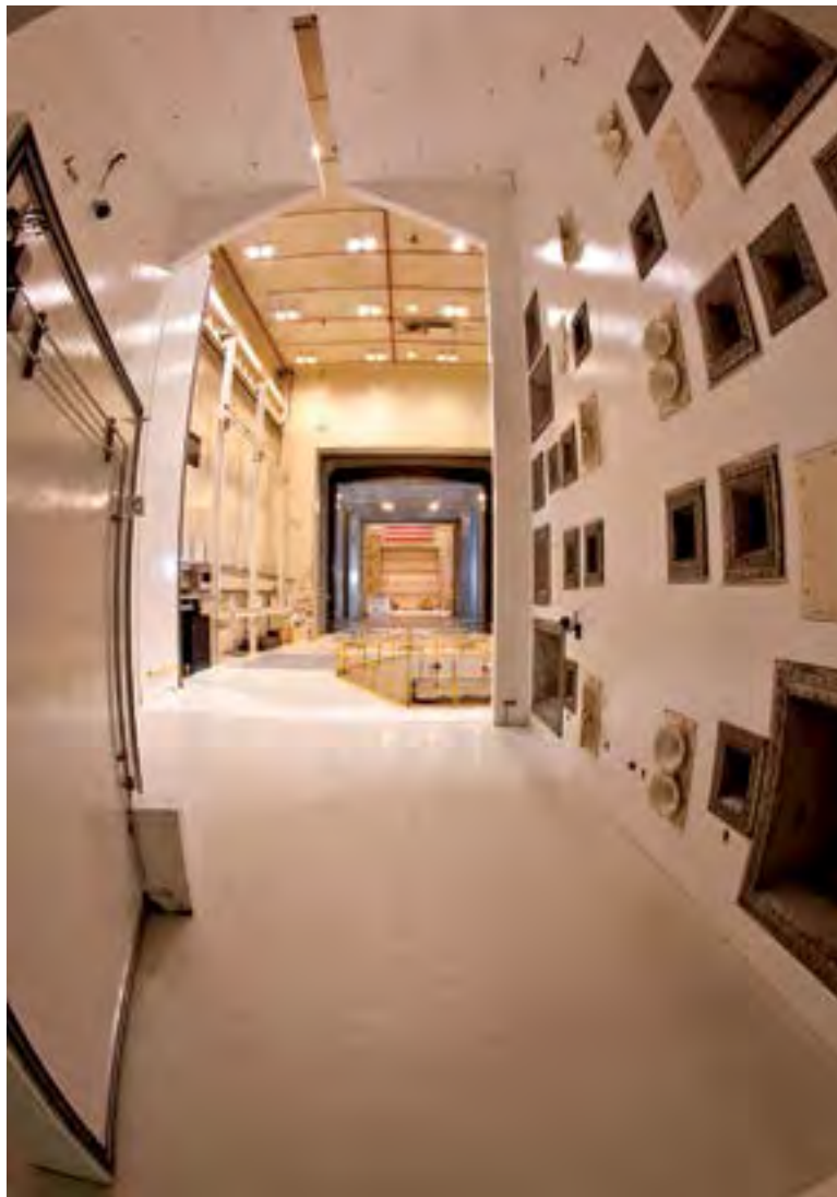
Image 387: The acoustics chamber in the SPF facility to be used for vehicle vibrational and structural dynamics testing (GRC-2011-C-04392).
