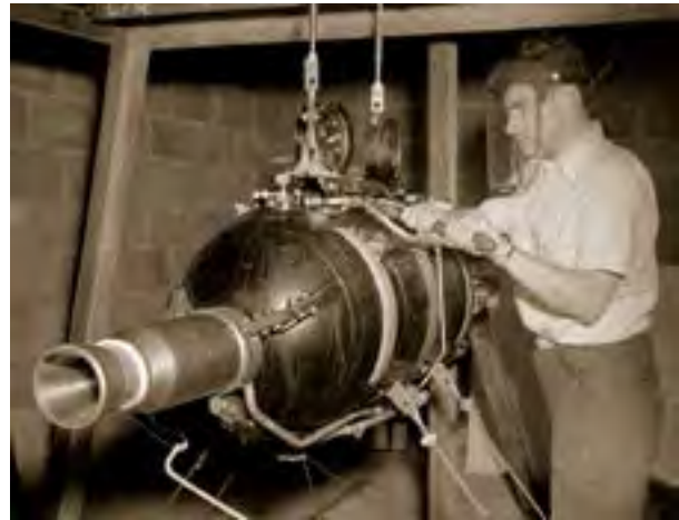
Image 119: A researcher prepares a jet-assisted take off (JATO) rocket for a combustion study at the Rocket Lab (GRC-1945-C-10724).
