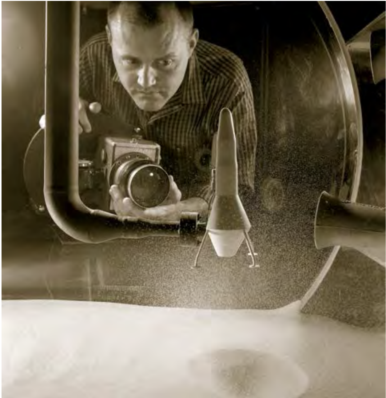
Image 212: Bill Harrison films a test analyzing the effect of a lander's jets on simulated Moon dust. This experimental tank was located in the 8×6 complex (GRC-1960-C-53768).
