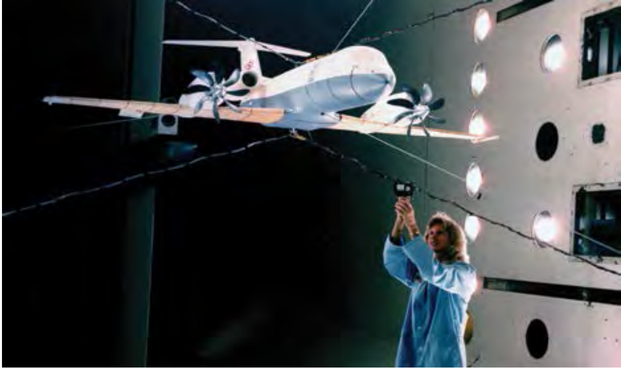
Image 297: A Propfan Test Assessment model is tested for flutter in the 9×15 wind tunnel during October 1985 (GRC-1985-C-07896).
