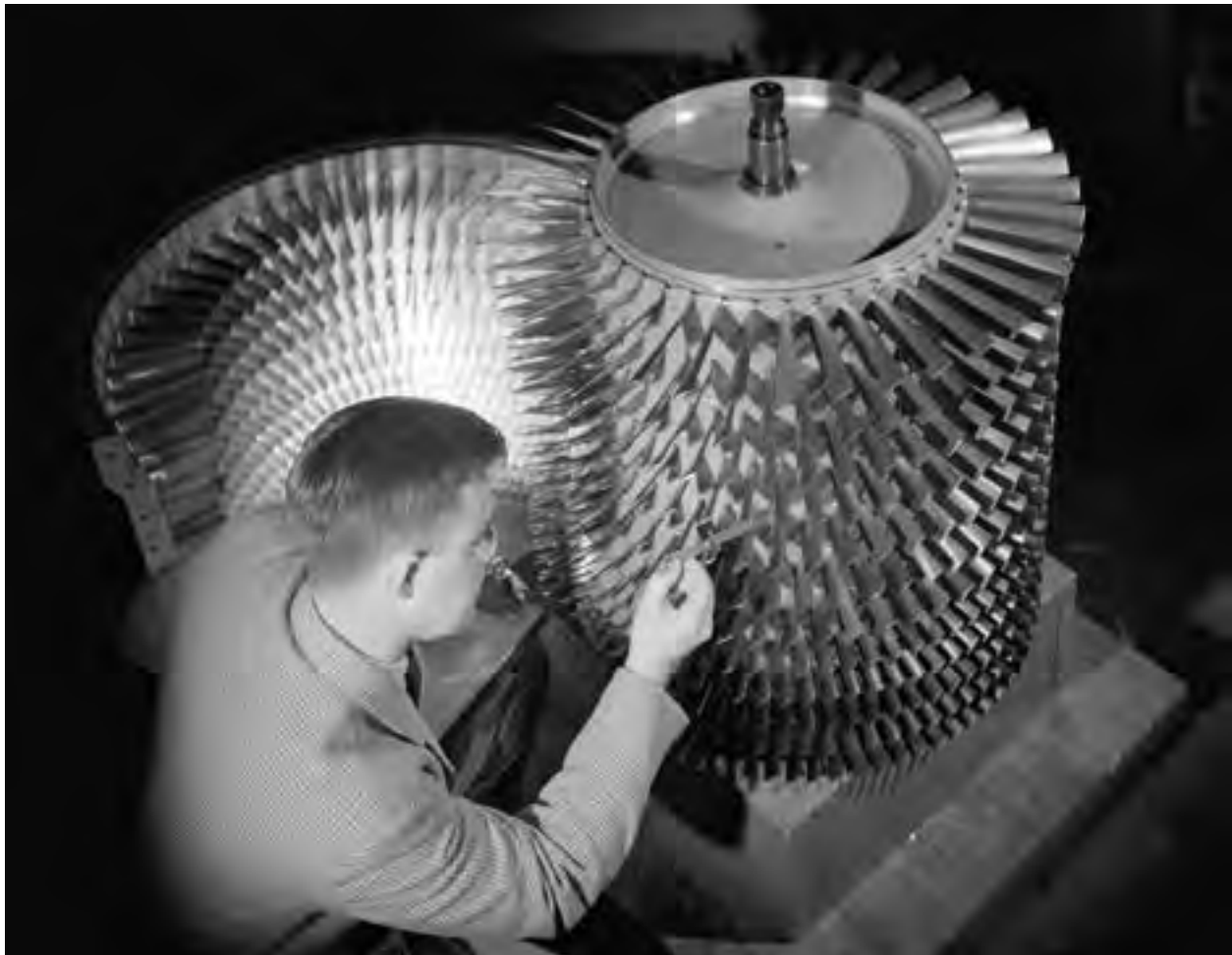
Image 146: A researcher measures the turbine blades on a 12-stage axial-flow compressor in February 1955 (GRC-1955-C-37659).
