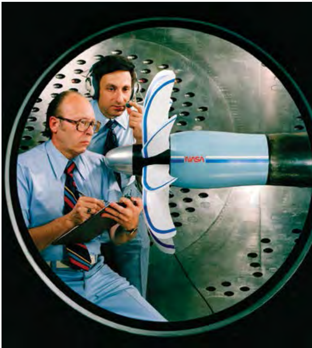
Image 273: Salvatore Grisaffe (left) and Oral Mehmed with a Hamilton Standard SR–6 propfan in the 8×6 test section (GRC–1980–C–04620).
