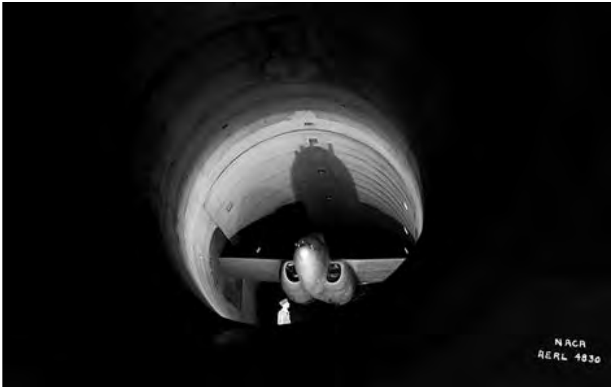
Image 72: The secret test of the Bell YP-59A Airacomet in the spring of 1944 was the first investigation in the new AWT. The Airacomet, which was powered by two General Electric I-A centrifugal turbojets, was the first U.S. jet aircraft (GRC-1944-C-04830).
