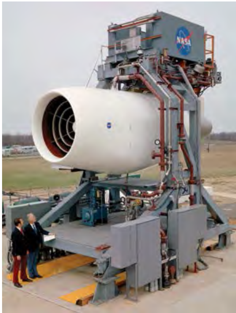
Image 219: A General Electric Quiet Engine tested with Lewis's acoustically treated nacelle on the hangar apron (GRC-1972-C-01486).
