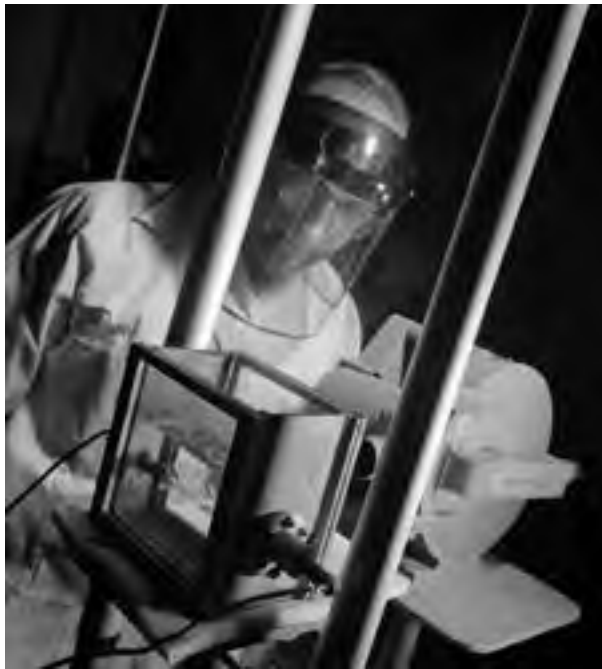
Image 200: Bob Siegel with a test rig for high-speed filming of liquid behavior in microgravity in the 8×6 wind tunnel (GRC-1960-C-54149).
