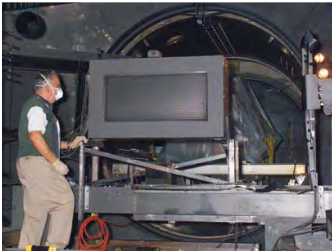
Image 370: A rectangular HiPEP thruster being removed from the EPL vacuum tank in June 2005 after the duration test (GRC-2005-C-01061).
