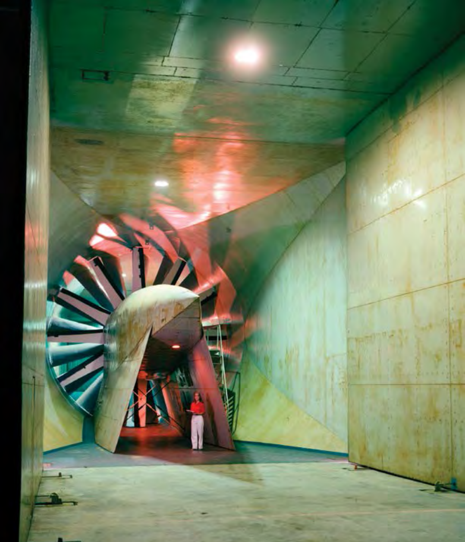
Image 291: The Icing Research Tunnel's drive fan as it appeared in July 1982. The IRT had been recently restored to support Lewis's reinstated icing research program (GRC -1982-C-04302).
