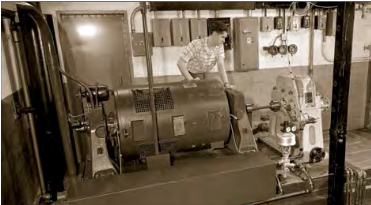
Image 148: The high-speed, high-temperature test rig in the Fuels and Lubrication Building (GRC-1953-C-32722).
