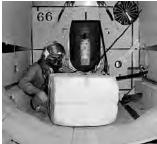
Image 201: Fred Haise, Lewis pilot and future Apollo astronaut, monitors the cameras and instrumentation for the experimental liquid-hydrogen container in the bomb bay of the AJ-2 aircraft (GRC-1961-C-56862).
