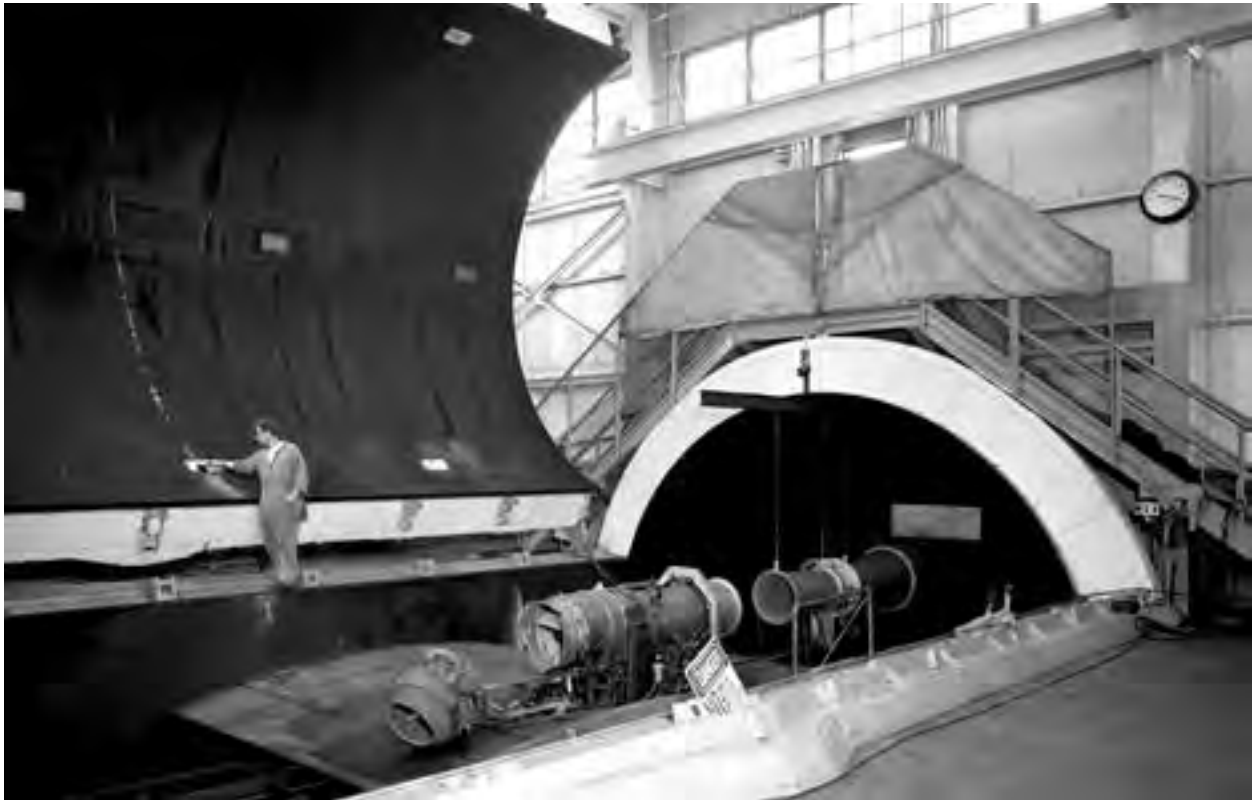
Image 92: A failure of a Westinghouse J34 engine in the AWT test section (GRC-1950-C-26294).
