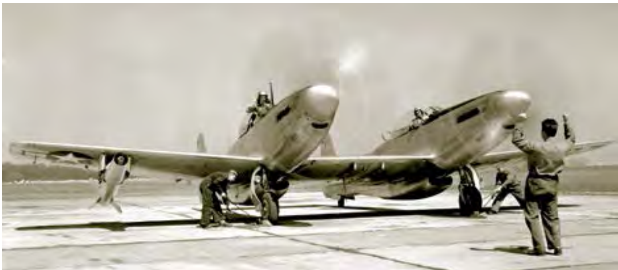
Image 116: A North American XF-82 Twin Mustang prepares for flight with a ramjet missile under its right wing (GRC-1949-C-23330).
