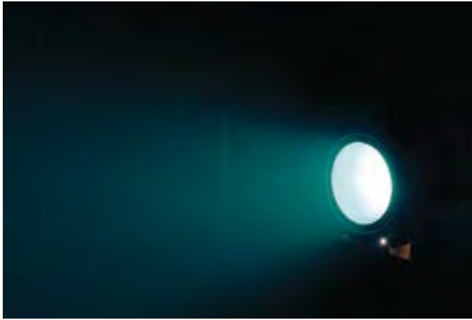
Image 371: Testing of a prototype NEXT thruster in the EPL during May 2006 (GRC-2006-C-01260).
