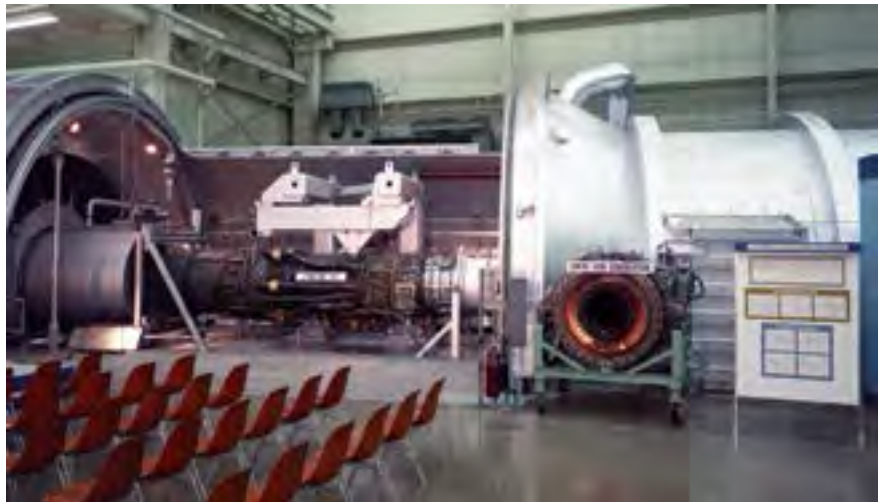
Image 256: A J-58 engine in a new test chamber in the Propulsion Systems Laboratory (PSL) with a swirl-can combustor on display (GRC-1973-C-03376).
