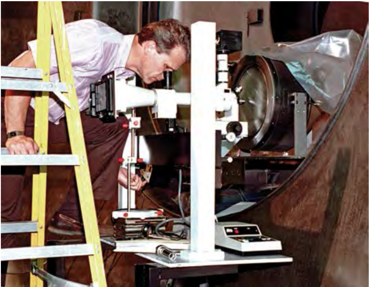
Image 336: A researcher prepares the NSTAR thruster for a 2000-hour wear test in the EPL during November 1994 (GRC-1994-C-05234).
