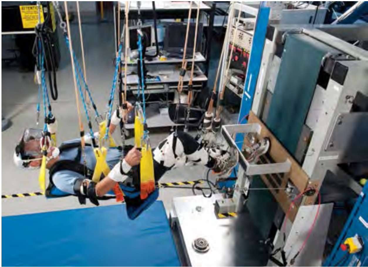
Image 399: The vertical treadmill is demonstrated in Glenn's Exercise Countermeasures Lab. The treadmill, referred to as the "Standalone Zero Gravity Locomotion Simulator," allows researchers to study the effects of low gravity on astronaut exercise (GRC-2010-C-03733).
