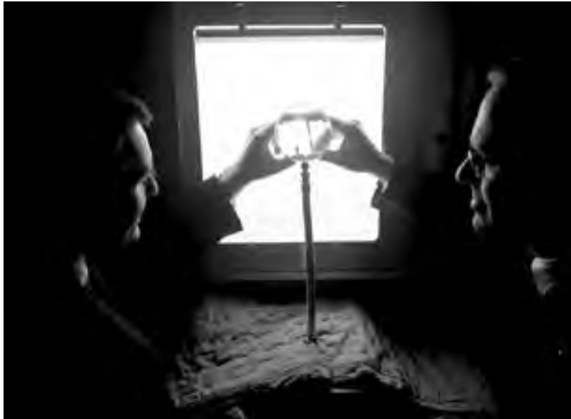
Image 221: Plum Brook Station manager Alan “Hap” Johnson and reactor chief Brock Barkley examine Moon dust that had been irradiated in the PBRF to identify its composition. The 25 milligrams of lunar soil had been retrieved by the Soviet Luna XVI spacecraft in September 1970 (GRC-1970-C-00950). 549
