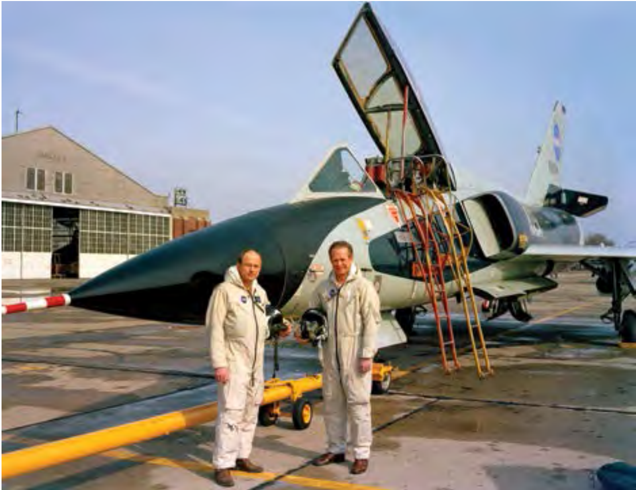
Image 217: Pilots Clifford Crabs and Byron Batthaer with Lewis's F-106B Delta Dart. The modified fighter aircraft could record 480 pressure measurements and nearly 100 other flight characteristics every 11 seconds (GRC-1971-C-00847).
