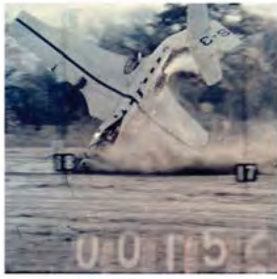
Image 140: A 1955 example of Bill Wynn's innovative visual timekeeping method for the Crash Fire Program (GRC-C-1955-38196).
