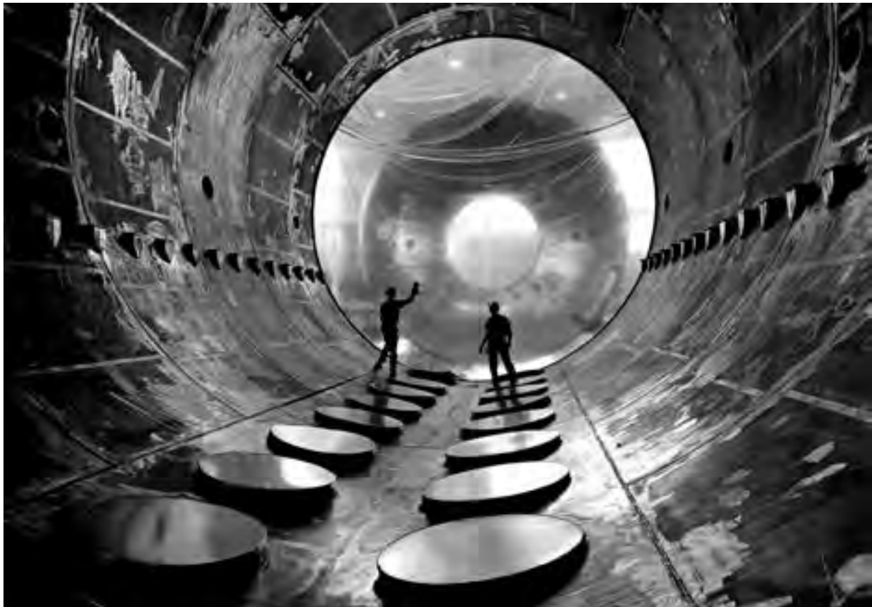
Image 186: Interior of the 20-foot-diameter vacuum tank in the Electric Propulsion Laboratory. The circular covers on the floor sealed the displacement pumps located beneath the chamber (GRC-1961-C-57748).
