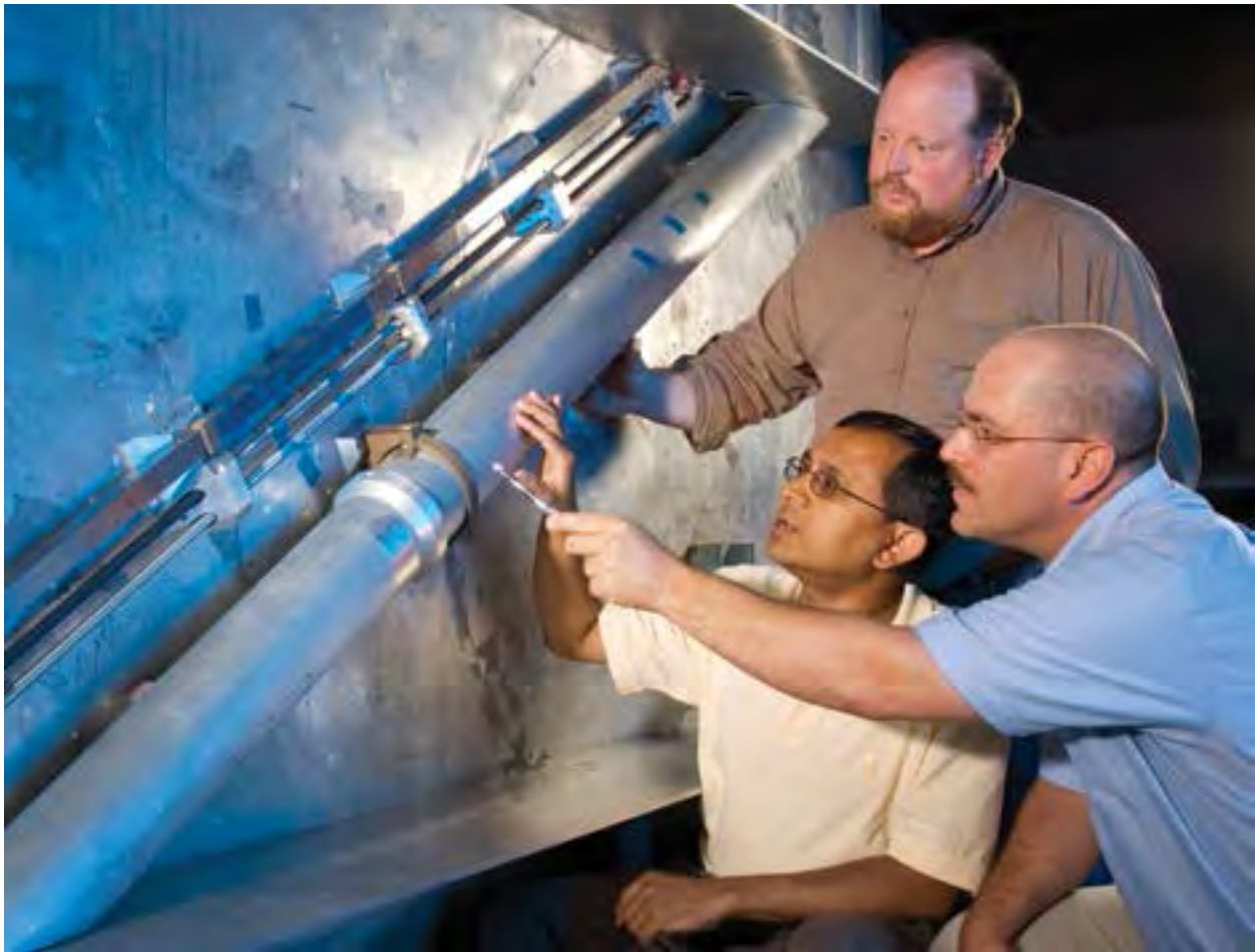
Image 363: Jayanta Panda, Scott Williamson, and Daniel Suliff examine the shuttle ramp protuberance test setup in the 8- by 6-Foot Supersonic Wind Tunnel (8×6) (GRC-2007-C-01848).
