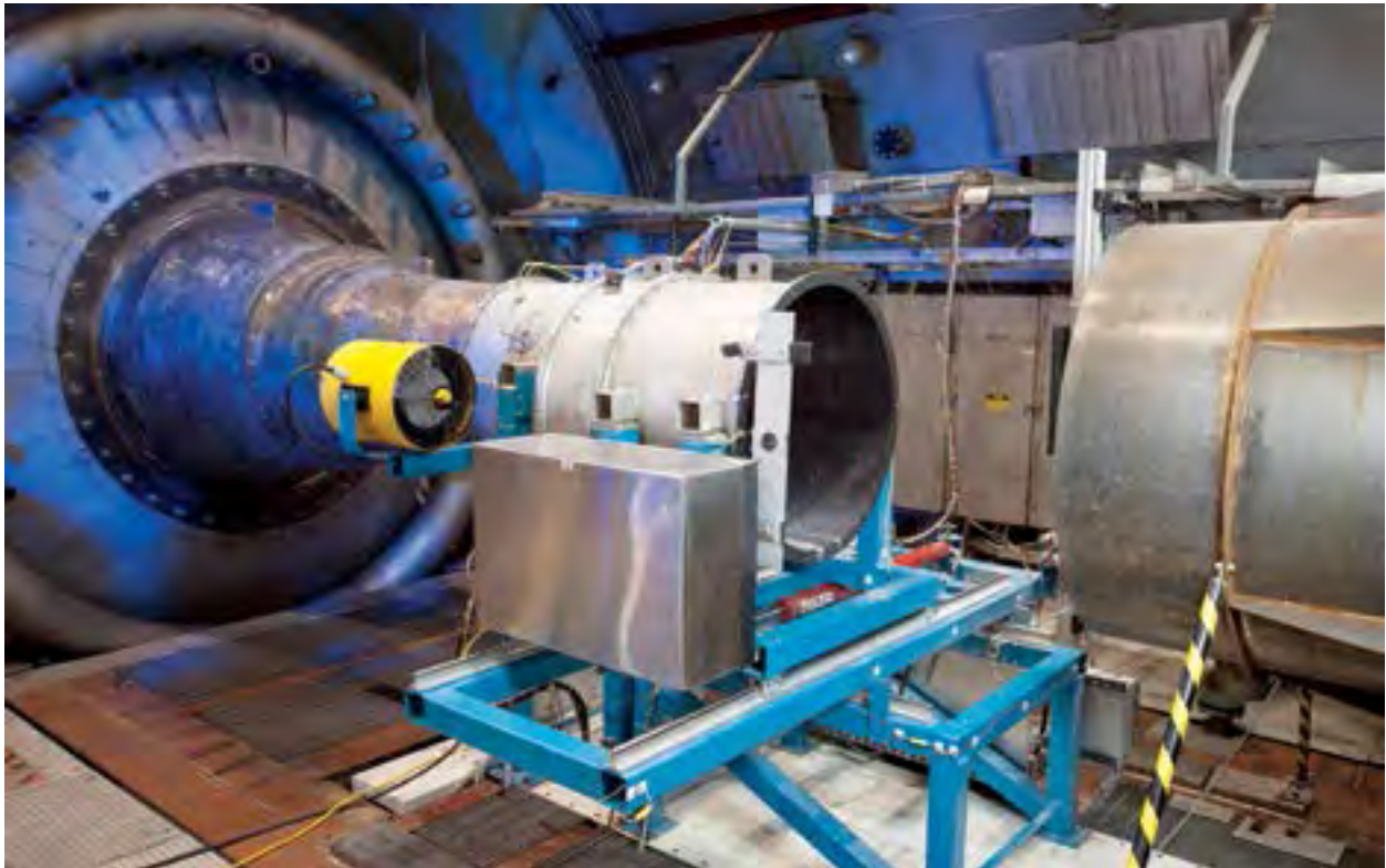
Image 392: PSLs No. 3 test chamber was modified for high-altitude engine icing tests (GRC-2012-C-04153).
