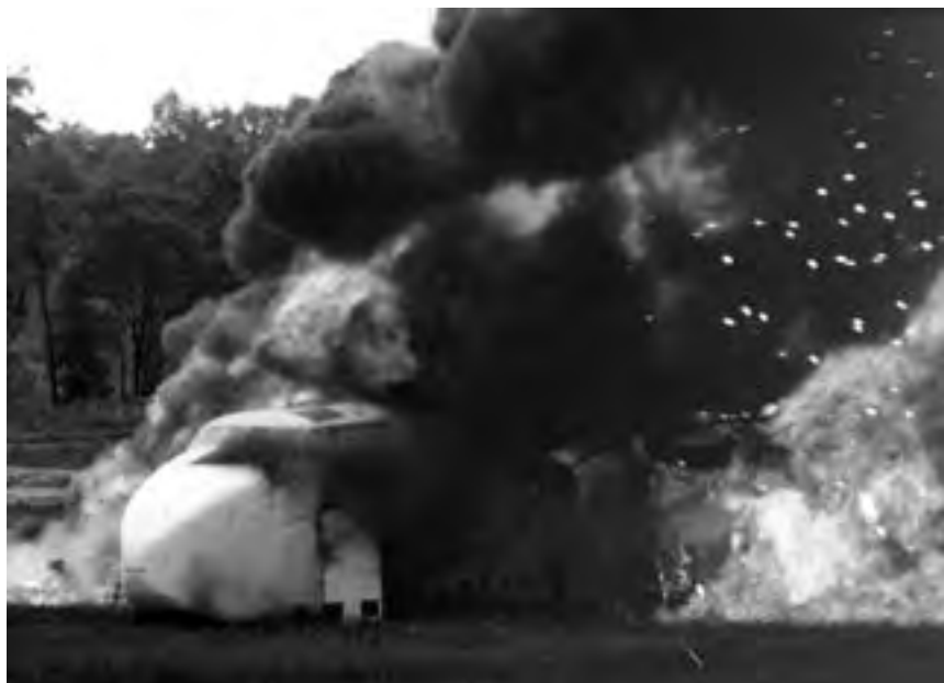
Image 139: Lewis researchers crash a transport aircraft through barriers at the Ravenna Arsenal. Incandescent particles are visible from the explosion (GRC-1957-C-43929).
