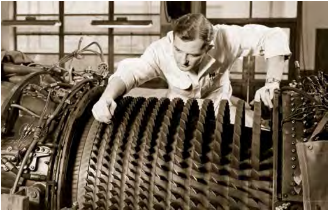
Image 91: A mechanic examines compressor blades on a General Electric J47 engine (GRC-1949-C-22850).
