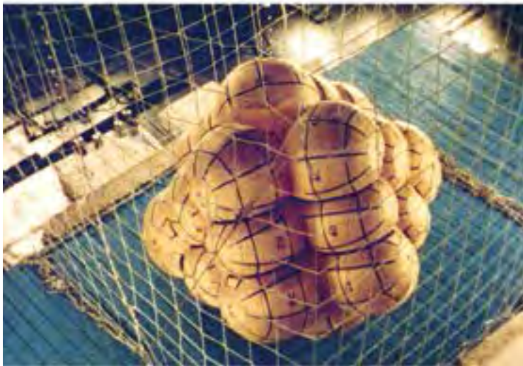
Image 333: Pathfinder airbag drop in the SPF (GRC-1995-C-01614).
