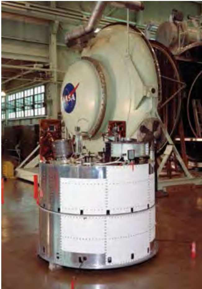
Image 234: SERT-II spacecraft in the foreground after testing in the EPL in December 1969 (GRC-1970-C-00112).
