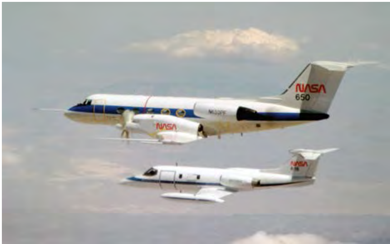
Image 296: The Gulfstream II and Learjet, both flown by Lewis pilots, conduct inflight noise measurements (GRC-1987-C-10756).
