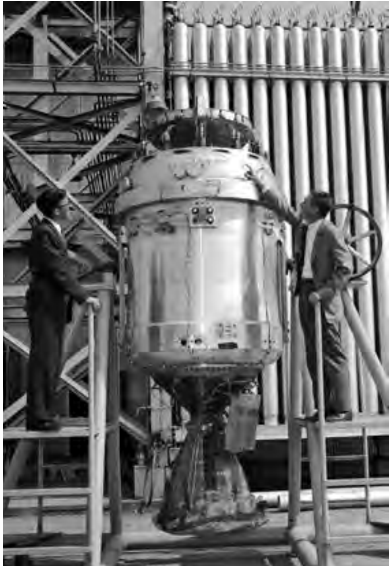
Image 197: An unfueled Kiwi B-1-B reactor and its Aerojet Mark IX turbopump being prepared for installation in the B-3 test stand (GRC-1967-P-01289).
