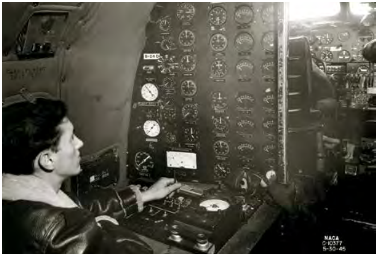
Image 101: A flight research member examines instrumentation in the B-24D during a 1945 icing flight (GRC-1945-C-10377).
