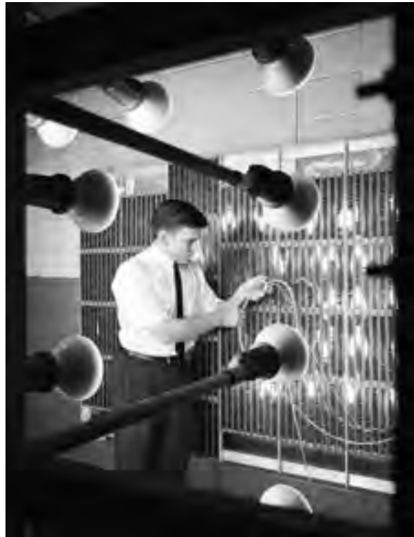
Image 236: High-voltage solar array test in the Engine Research Building during July 1965 (GRC-1965-C-01839).
