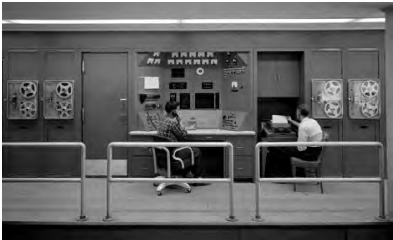
Image 153: Lewis engineers operate the CADDE system in the 10×10 (GRC-1956-C-42021).
