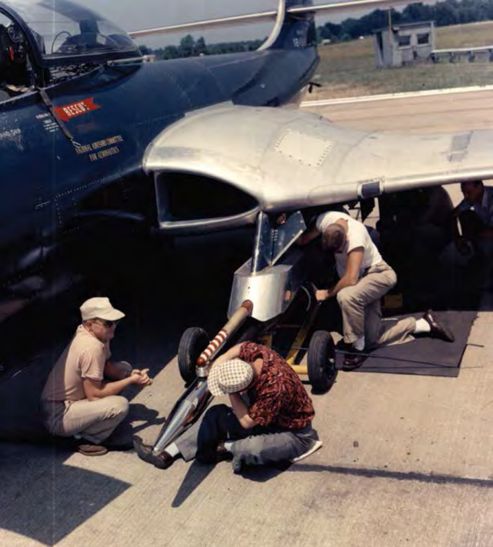
Image 125: Technicians install an experimental hypersonic test missile on the NACA's McDonnell F2H-2B Banshee in August 1957. Lewis pilots launched the missiles over the Atlantic Ocean at Wallops Island (GRC-2015-C-06812).
