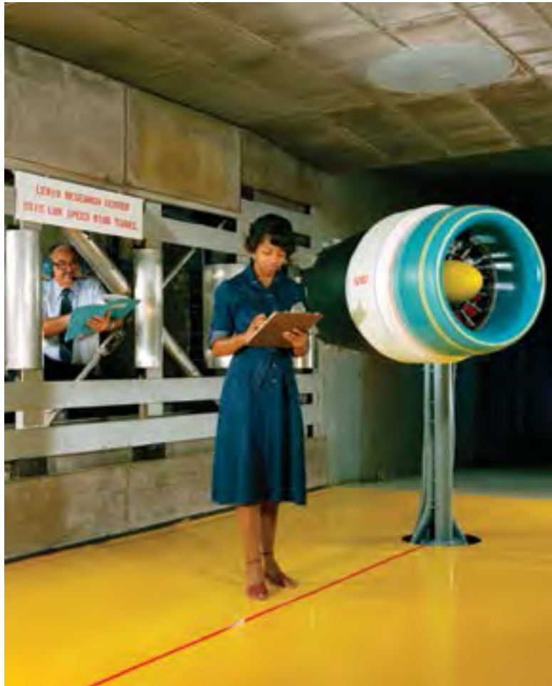
Image 269: A V/STOL engine with a zero-length inlet installed in the 9×15 (GRC-1980-C-04513).
