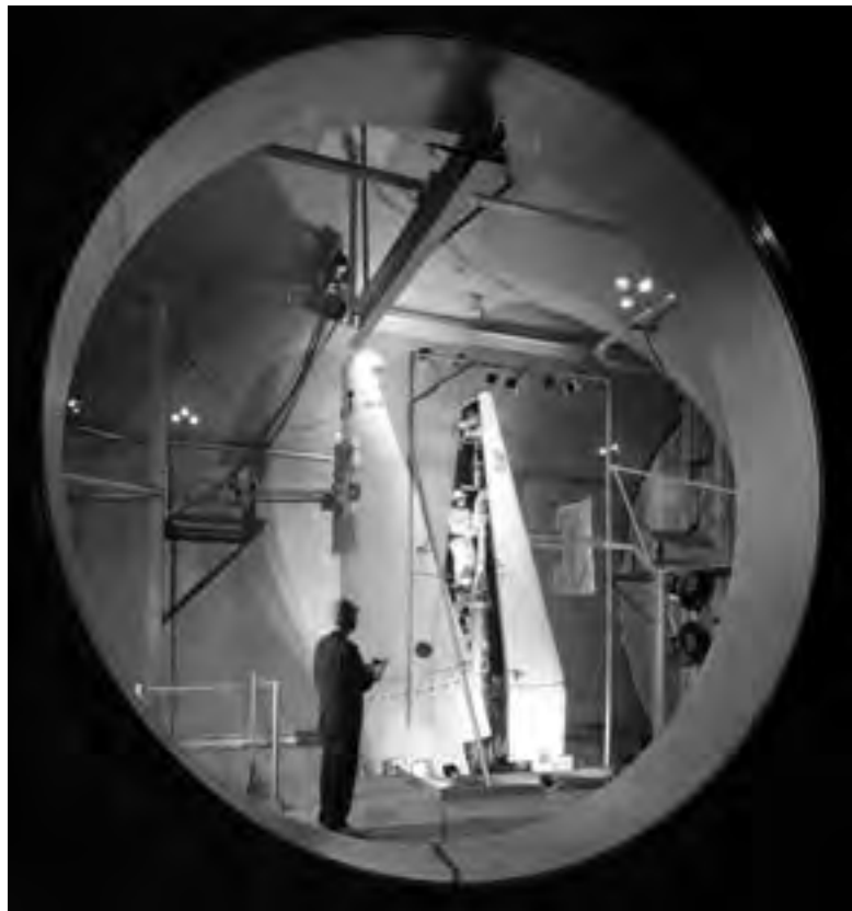
Image 209: Researchers prepare a Centaur-Surveyor nose cone shroud for a separation test in the SPC vacuum tank (GRC-1964-C-71091).
