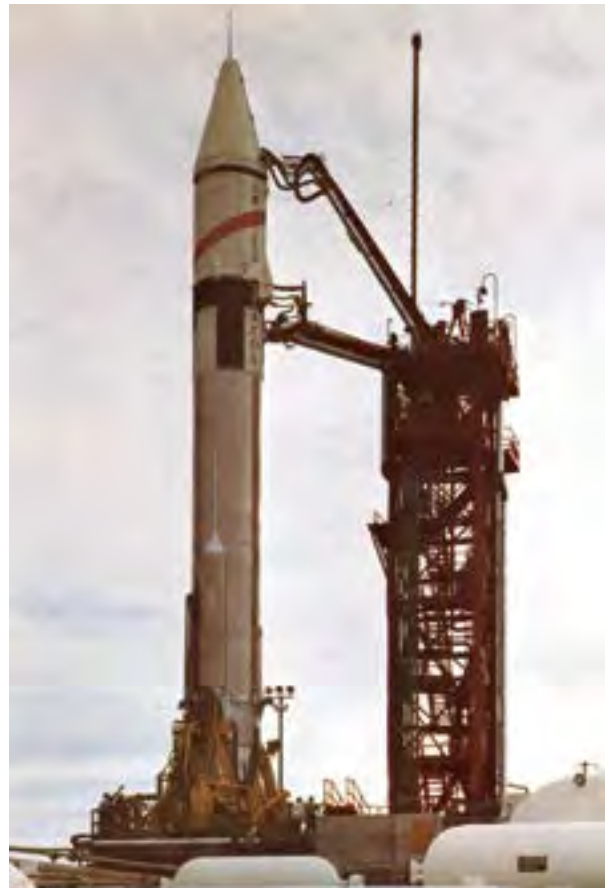
Image 208: AC-2 on a launch pad at Cape Canaveral in November 1963. It was the first successful launch of a liquid-hydrogen rocket. The Centaur upper stage from the AC-2 launch remains in orbit today (GRC-2015-C-06539).
