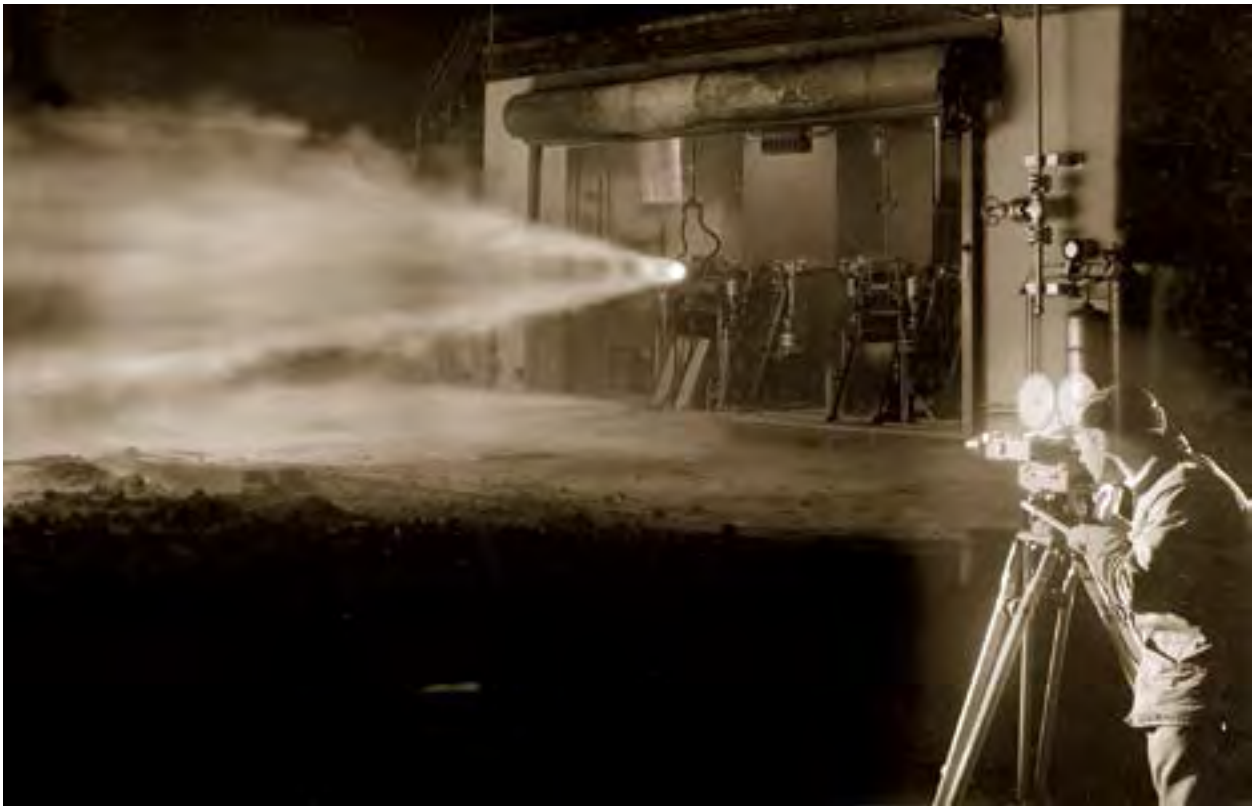
Image 156: A photographer films the operation of a liquid-hydrogen/liquid-oxygen rocket engine in Cell 22 of the Rocket Lab. Tests were run in the evening when most of the lab was relatively vacant (GRC-1955-C-37427).
