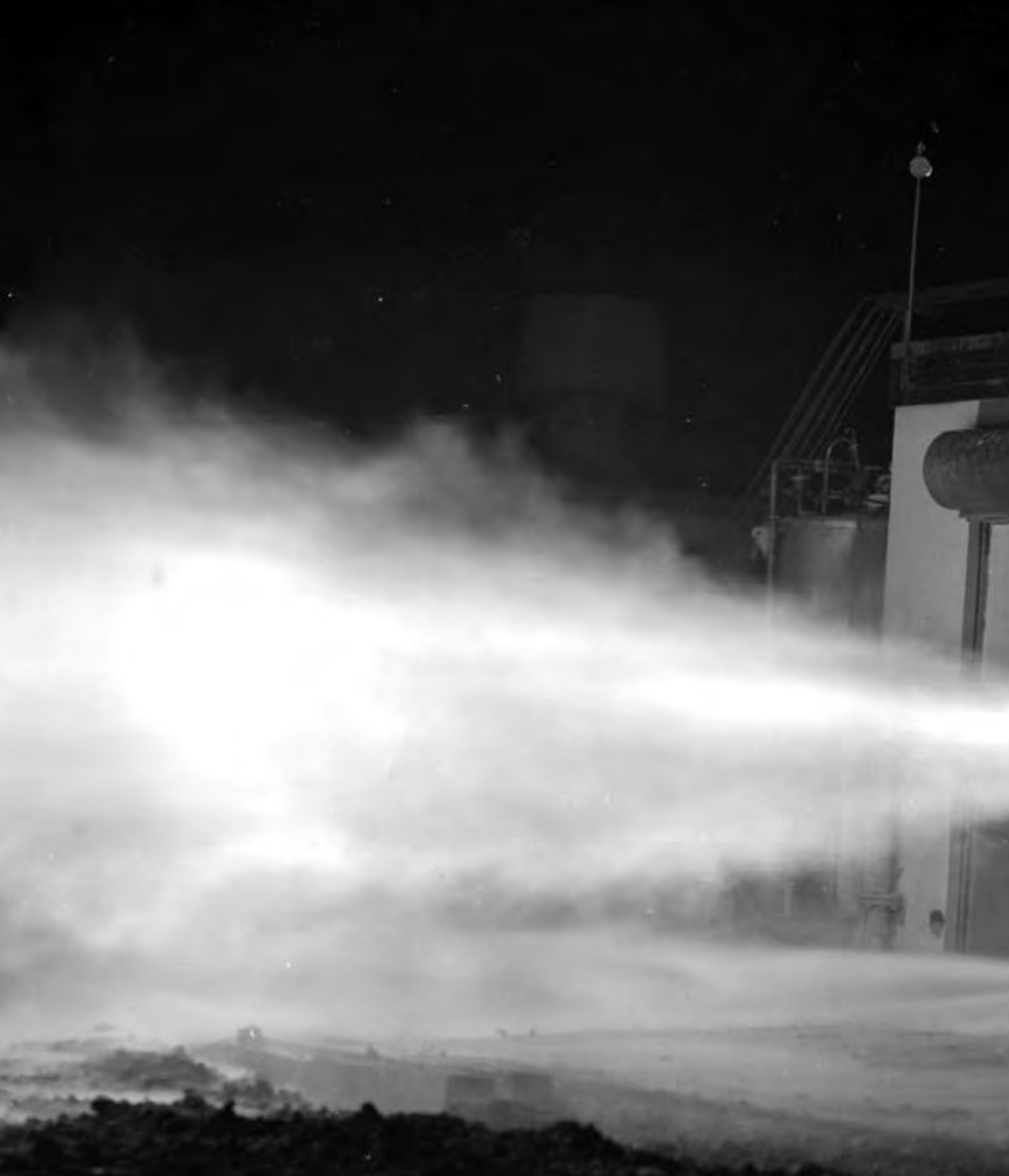
Image 124: A 5,000-pound-thrust rocket engine is fired from the Rocket Lab's Cell 22 in January 1955. The series of tests proved to be Lewis's first successful liquid-hydrogen/liquid-oxygen runs (GRC-1955-C-37428).
