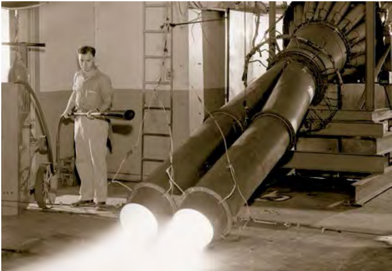
Image 93: A mechanic with a fire extinguisher watches the firing of twin afterburners (GRC-1949-C-23744).
