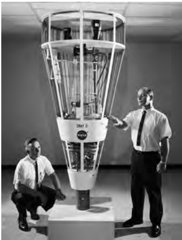
Image 237: A model of the SNAP-8 power system created by the Lewis Fabrication Shop prior to a September 1966 Space Power Conference at the center (GRC-1966-C-03304). 586
