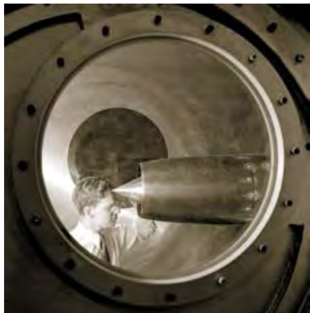
Image 118: A researcher inspects a 16-inch-diameter ramjet engine in the 8×6 test section. Researchers studied the ramjet's performance at different speeds and varying angles of attack. The engine performed well, and the findings correlated with nonfueled studies in the smaller wind tunnels (GRC-1950-C-25776).
