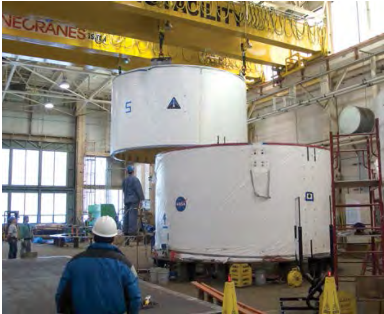
Image 383: Stacking of two Ares I-X segments in the Fabrication Shop, which was renamed the “Ares Manufacturing Facility” (GRC-2008-C-00421).
