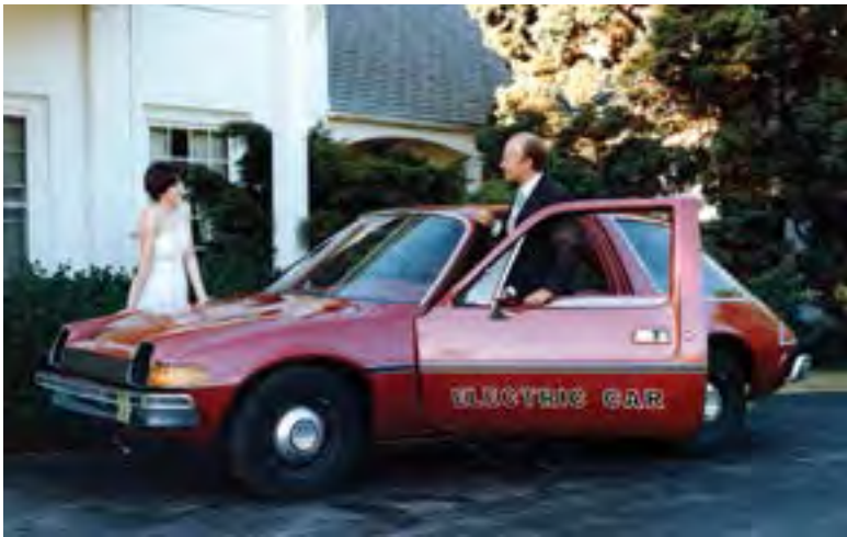
Image 268: American Motors Pacer vehicle modified to run on twenty 6-volt batteries (GRC-1977-C-02096).
