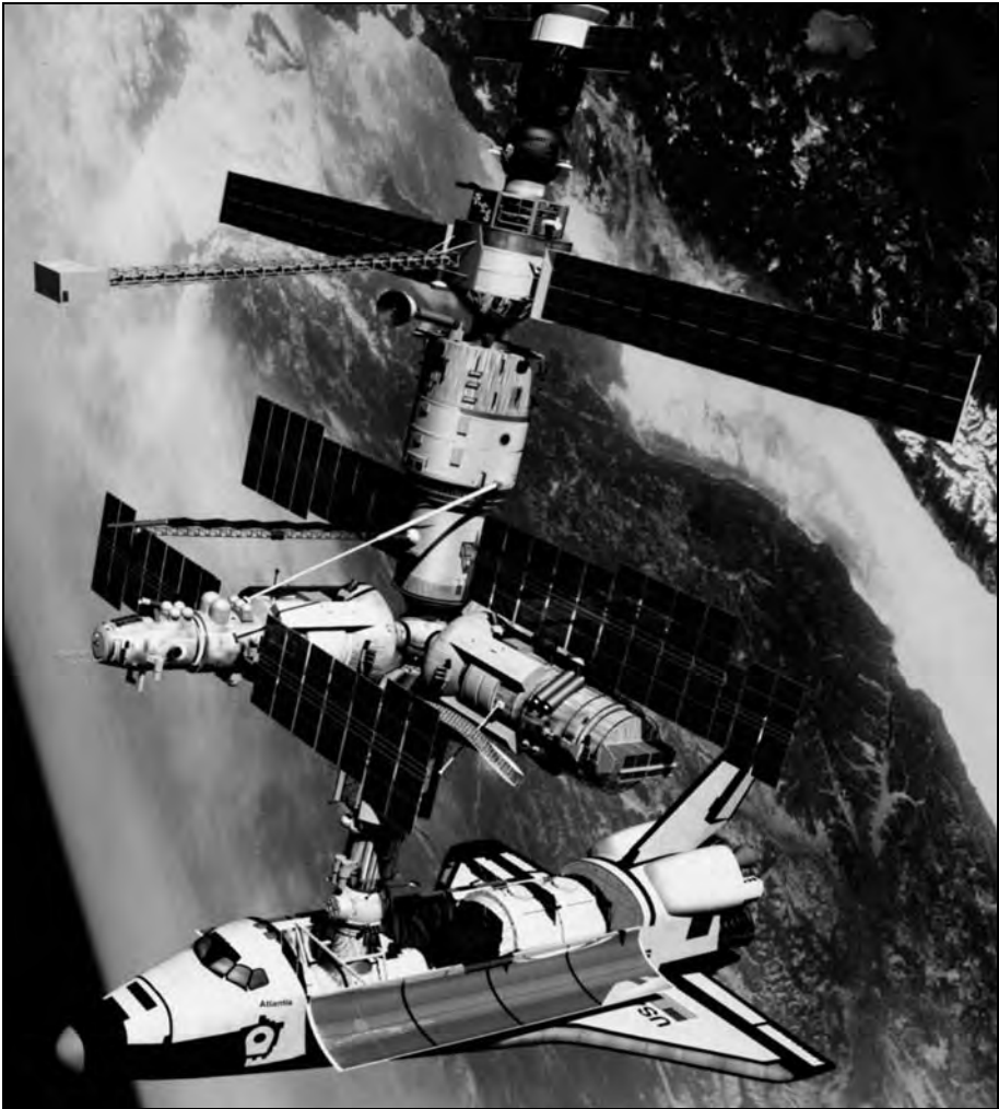
Figure 3–54. A technical rendition of the Space Shuttle Atlantis docked to the Kristall Module of Mir. This configuration shows the STS-71/Mir Expedition 18 completed in June 1995. The Russian-developed Androgynous Peripheral Docking System linked the orbiter to the Kristall Module. (NASA Photo No. S-93-46073)
