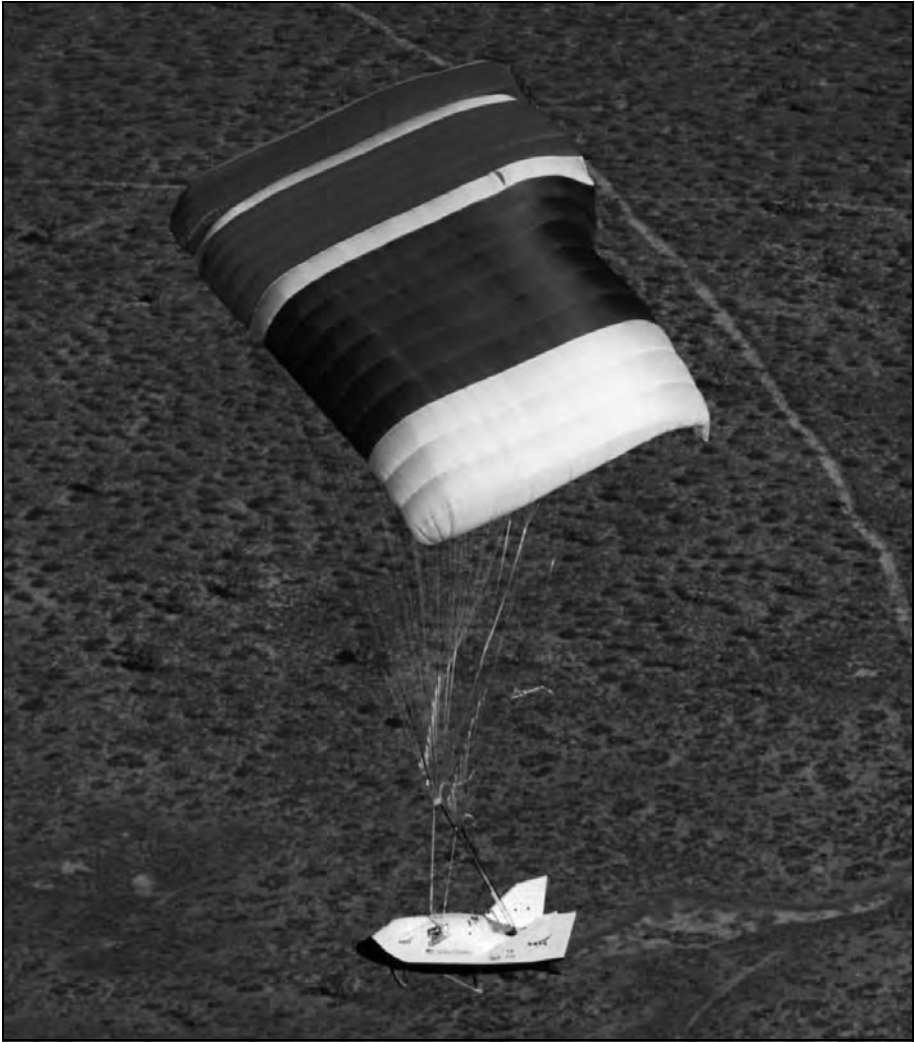
Figure 3-64. The X-38 descends under its steerable parafoil over the California desert during its first free flight at Dryden Research Center, March 12, 1998. (NASA-DFRC Photo No. EC98-44452-2)
