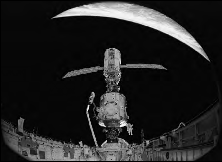
Figure 3–60. In December 1998, the crew of the STS-88 Mission began construction of the ISS, joining the U.S.-built Unity Node to the Russian-built Zarya Module. The crew used a large-format IMAX camera to take this photo, which shows astronauts Newman (left) and Ross maneuvering into position to continue work on Unity. (NASA Photo No. S99-03771)
