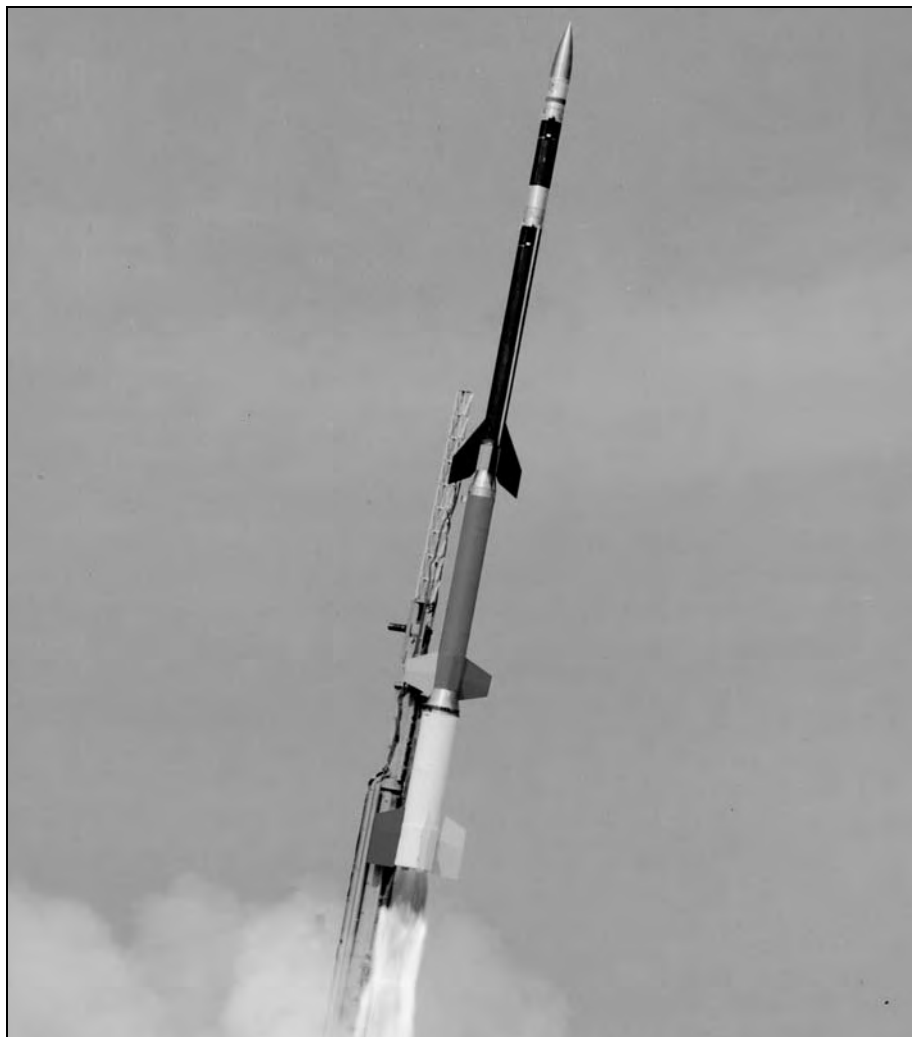
Figure 4-47. The four-stage Black Brant shown here blasting off from a launch pad at the Wallops Island Flight Facility in rural Virginia is at 66 feet (20 meters), the tallest of NASA's 13 sounding rockets. (NASA Photo No. WI-88-589-4)
