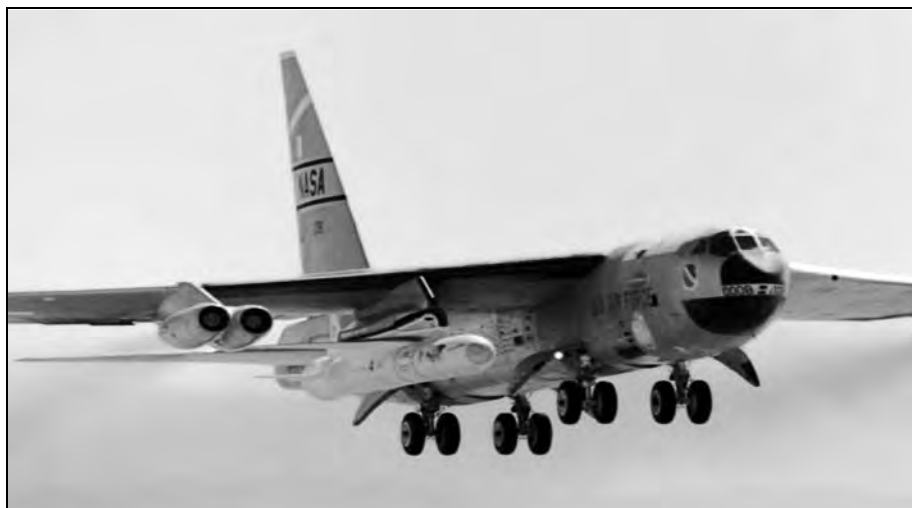
Figure 2-17. Pegasus Mounted Under B-52 Wing. (NASA-DFRC Photo No. EC91-348-3)
