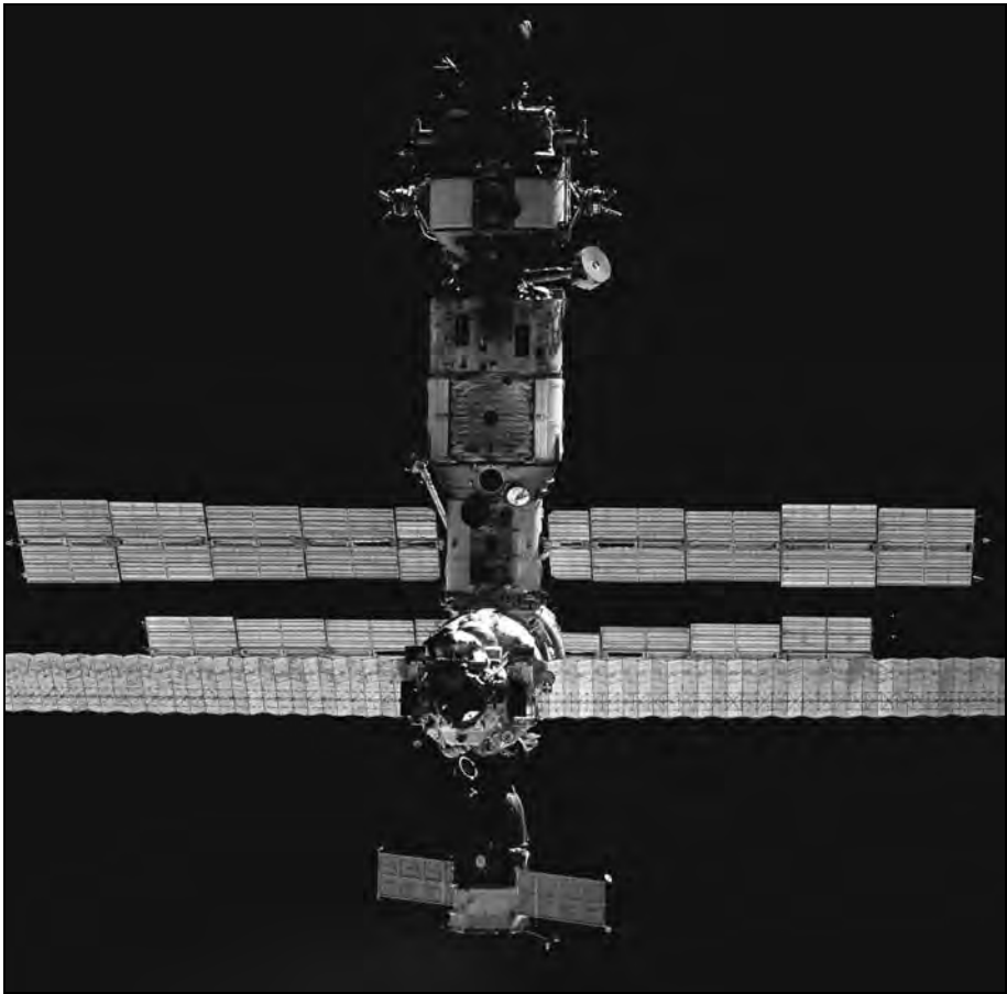
Figure 3–37. Russia's Mir Space Station during rendezvous operations with the Space Shuttle Discovery. Docked at the bottom of the Mir facility is a Soyuz vehicle. On STS-63, Discovery approached Mir, flew around the Russian Space Station, and then backed off. This provided practice for future docking missions. (NASA Photo STS063-712-017)
