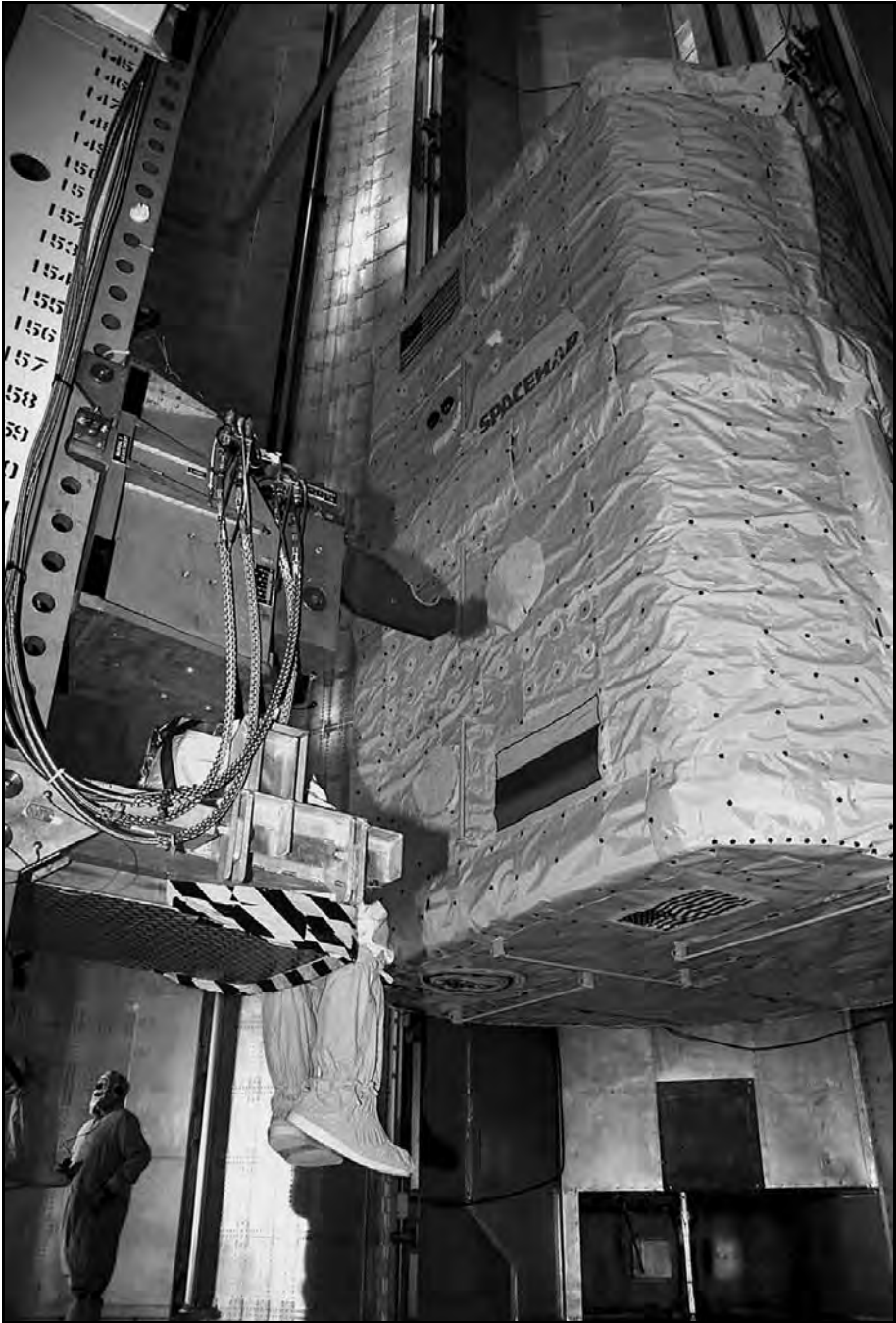
Figure 3-41. The SPACEHAB double module is lifted into the payload changeout room at Launch Pad 39-A for insertion into the payload bay of Atlantis. On STS-86, about 3-1/2 tons (3,175 kilograms) of science and logistical equipment and supplies were exchanged between Atlantis and Mir. (NASA Photo No. KSC-97PC-1340)
