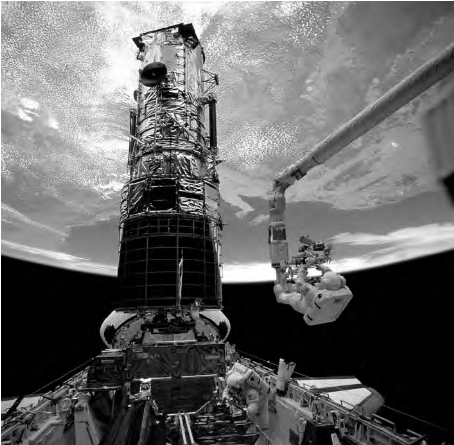
Figure 3–23. Astronaut F. Story Musgrave is seen anchored on the end of the Remote Manipulator System Arm as he prepares to be elevated to the top of the Hubble Space Telescope to install protective covers on the magnetometers, December 9, 1993. (NASA Photo No. GPN-2000-001085)
