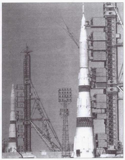
Two N1 Moon rockets appear on the pads at Tyura-Tam in early July 1969. In the foreground is booster number 5L with a functional payload for a lunar-orbiting mission. In the background is the 1M1 ground test mock-up of the N1 for rehearsing parallel launch operations. (files of Asif Siddiqi)
