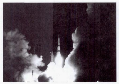
This photo captures the spectacular night launch of the third N1 rocket in June 1971. Although the booster cleared the tower, unanticipated rotations around the main vertical axis of the vehicle led to yet another catastrophic failure. (copyright Quest)
