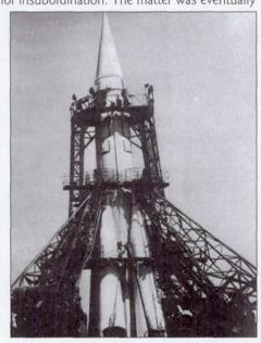
The first R-7 ICBM shown on the single launch pad at site 1 at Tyura-Tam in early 1957. Note the "tulip" launch structure around the base of the rocket. Later operational models of the rocket had a different payload fairing. (copyright Steven Zaloga)
