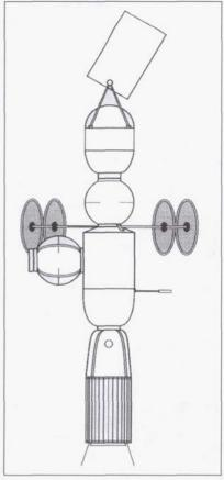
This is one conception of an early Earthorbital station dating from 1962. A visiting spacecraft called the Sever is shown docked to the station at the bottom of the drawing. The design of the Sever eventually evolved into the future Soyuz spacecraft. (copyright R. F. Gibbons, based on a drawing by Igor Afanasyev)
