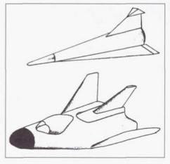
At top is a winged rocket-glider developed by the Tupolev design bureau in the early 1960s to carry out research at Mach 2–5 on the aerodynamic characteristics of a hypersonic winged vehicle. At bottom is the BOR-2 lifting body developed by the M. M. Gromov Flight-Research Institute in the late 1960s within the framework of the Spiral program. (copyright Asif Siddiqi)
