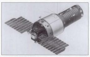
This drawing shows the flight variant of the Almaz space station with its unique docking node visible on the left. The viewport for the Agat-I reconnaissance camera was located on "the underside" of the vehicle, not visible in this image. (copyright VideoCosmos Co., via Dennis Newkirk)
