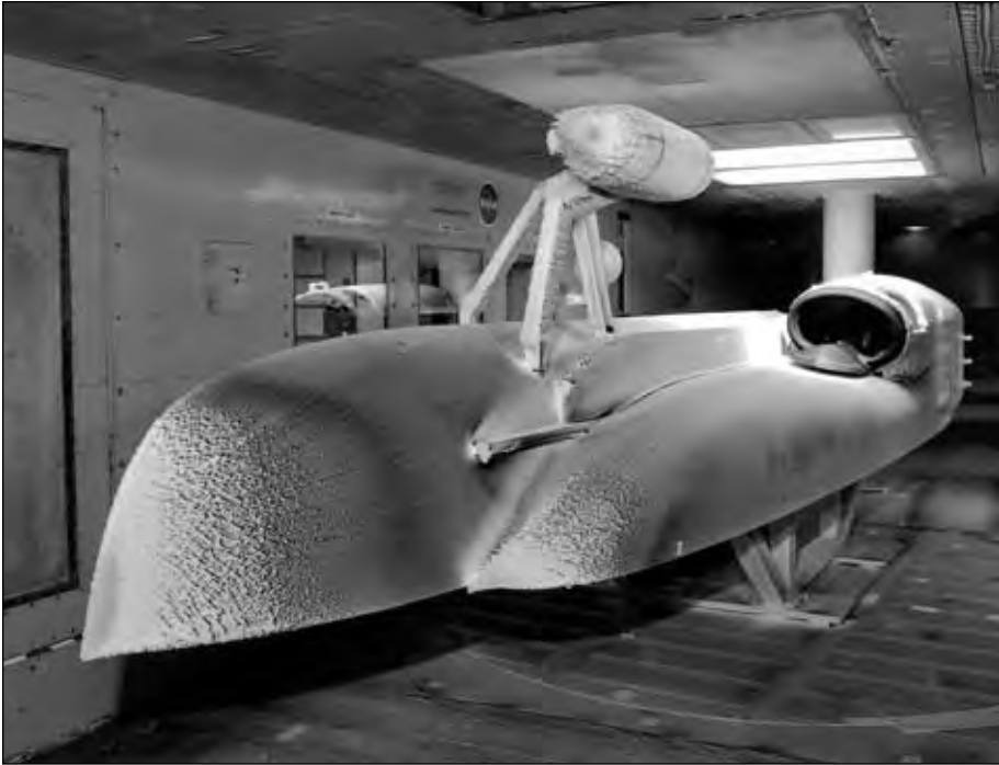
Figure 8–12. Icing tests of Sikorsky S-92 inlet in the IRT, 1998. (NASA C-98-1348)
