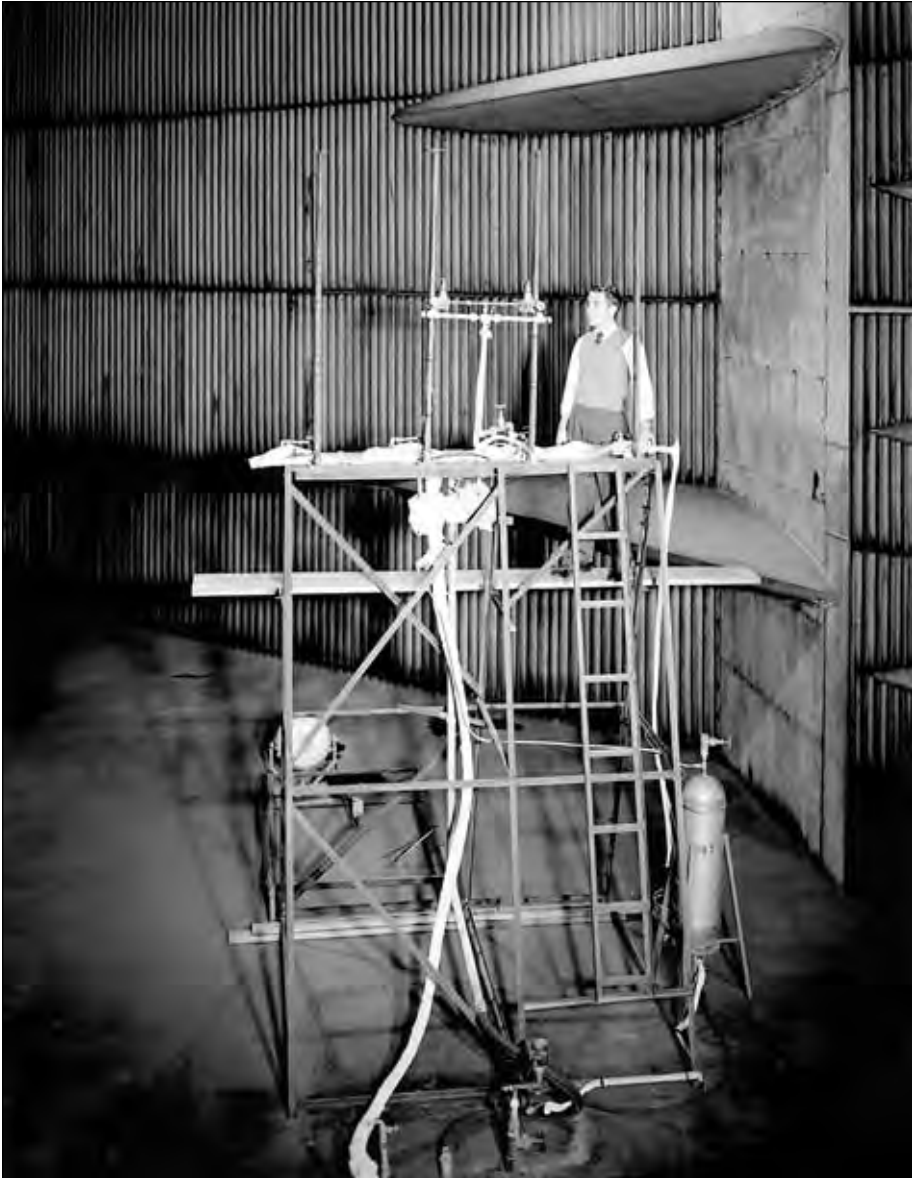
Figure 4-6. Researcher Thomas Gelder with spray system for dyed water impingement studies in IRT, 9 September 1949. (NACA C-49-24015)
