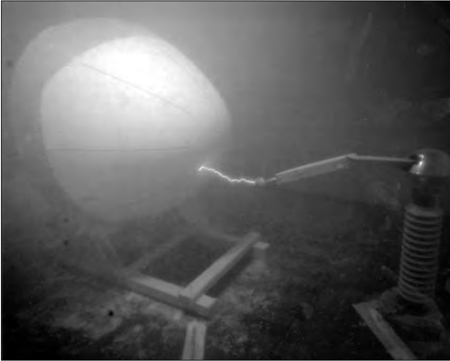
Figure 8-3. Lightning strikes on radome in IRT, 1995. (NASA C-1995-4457)
