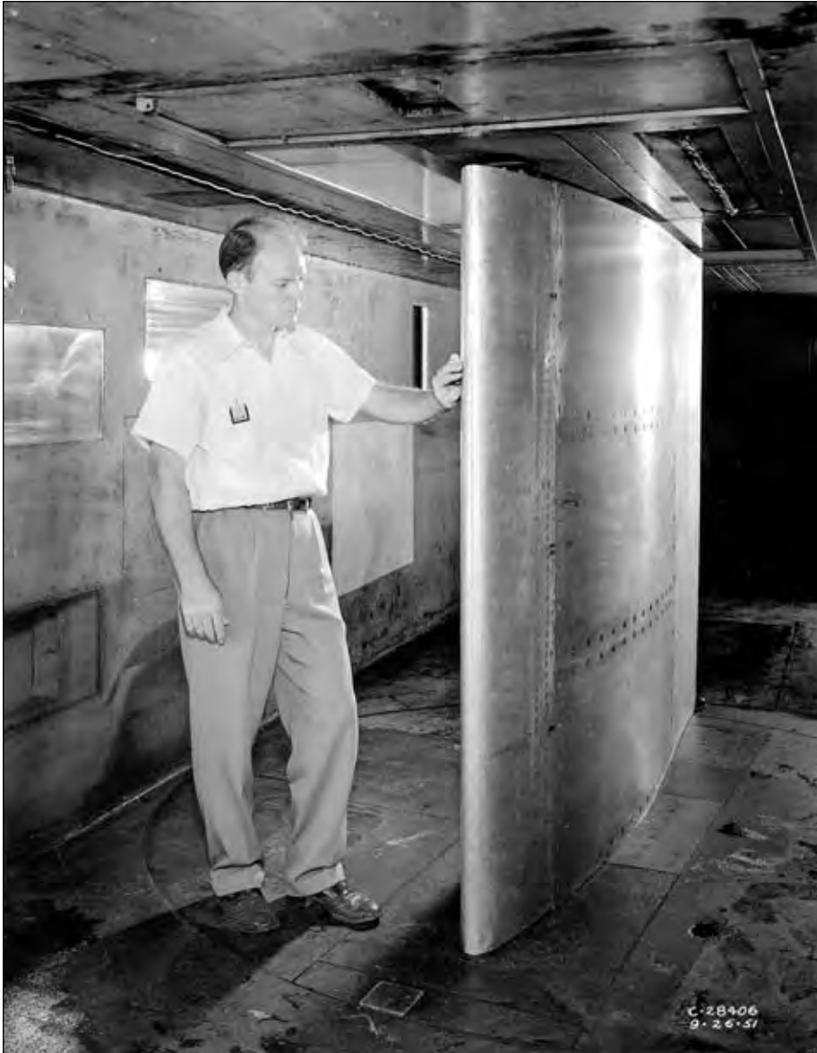
Figure 4-10. Vernon Gray inspects the airfoil model during cyclic gas de-icing experiments, 26 September 1951. (NACA C-28406)
