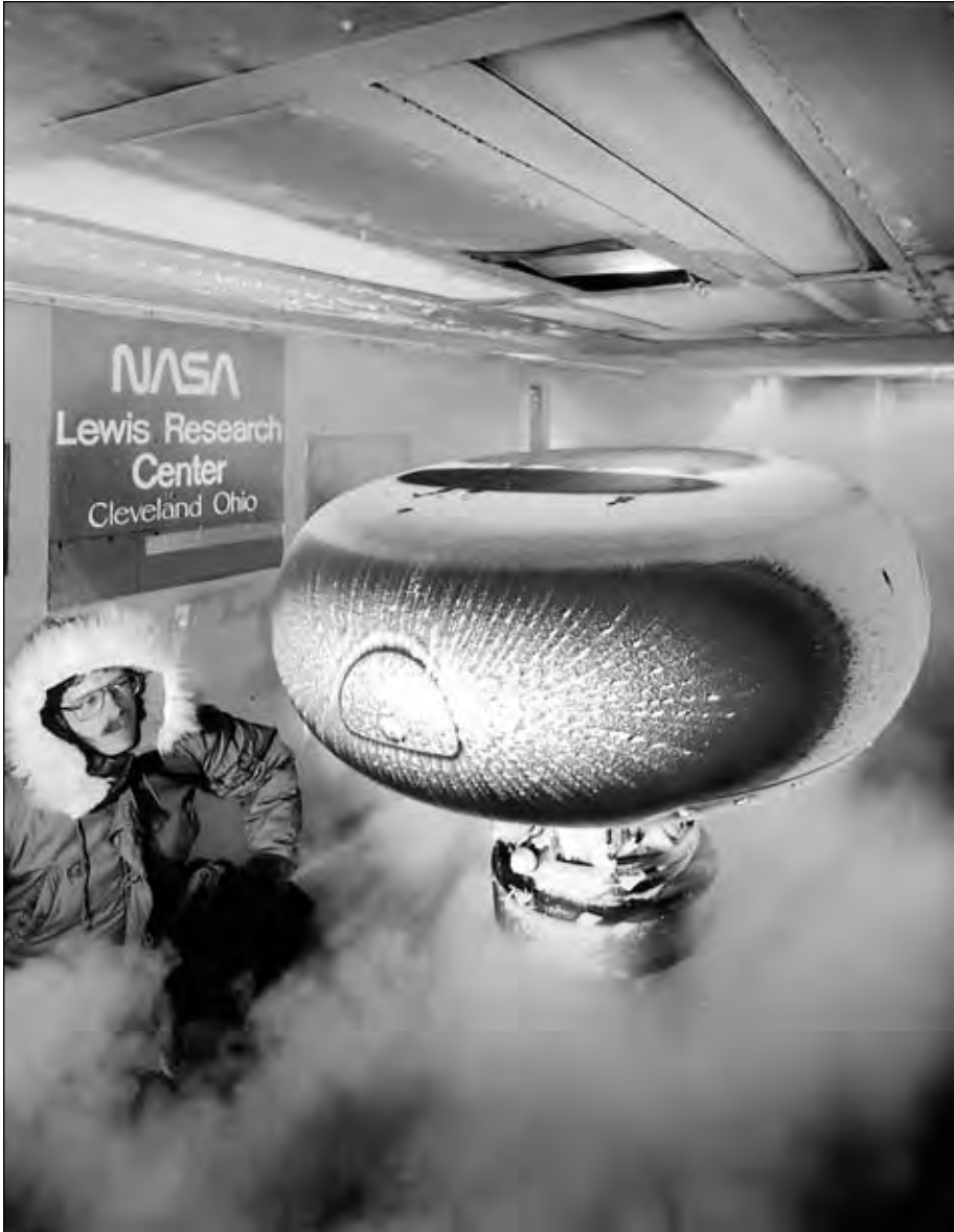
Figure 7-2. Technician Dan Gideon with AH-64 (Apache) Longbow fire control radar during icing tests, 1993. (NASA C-1993-4831)
