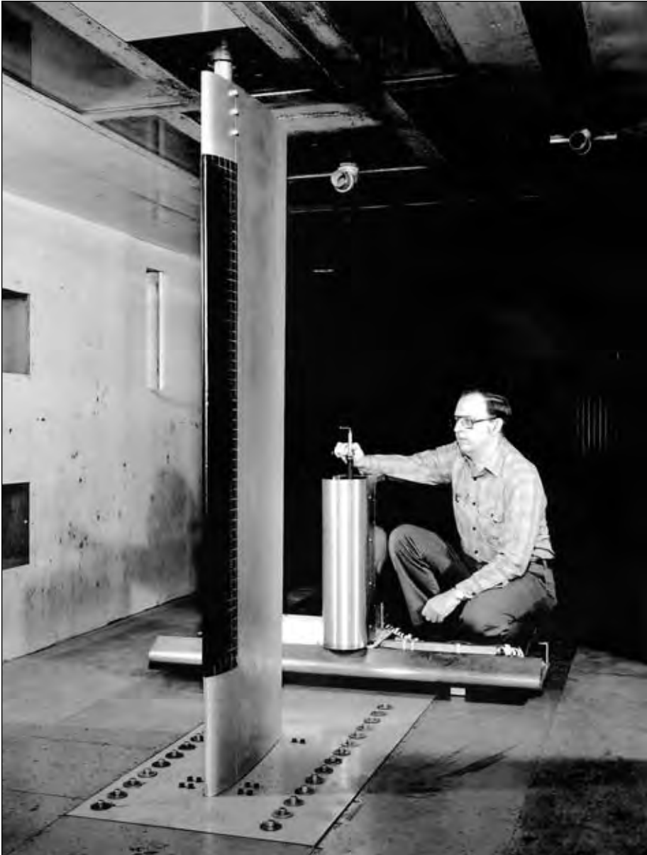
Figure 5-3. Technician Fred Murray with traverse rig in IRT, 1979. (NASA C-79-1686)
