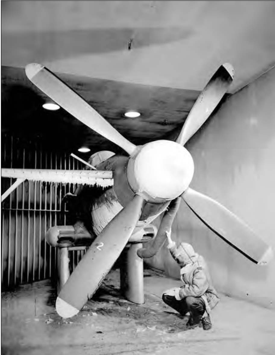
Figure 3-6. Rig for testing propellor ice-protection systems, 1946. (NACA C-15254)
