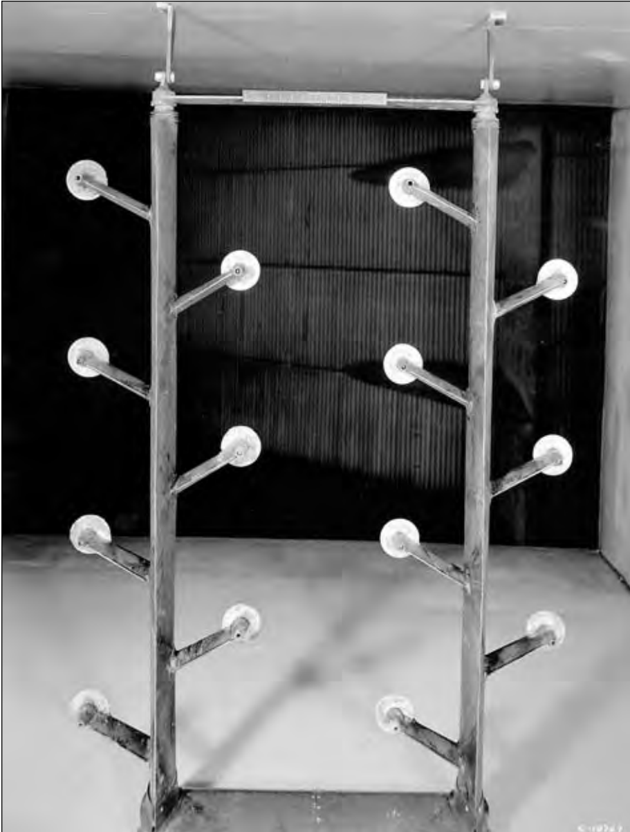
Figure 3-9. Water spray test in the IRT, 22 September 1947. (NACA C-19747)
