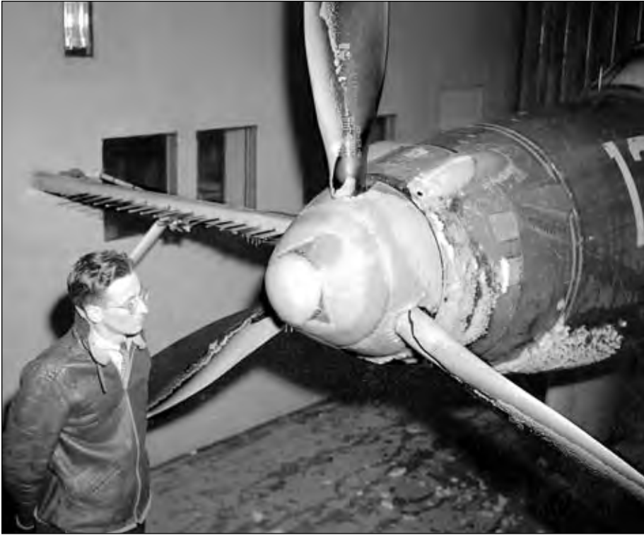
Figure 3-3. James P. Lewis inspects fuselage of a P-39 mounted in IRT for study of ice formation on propellers. (NACA C-10186)
