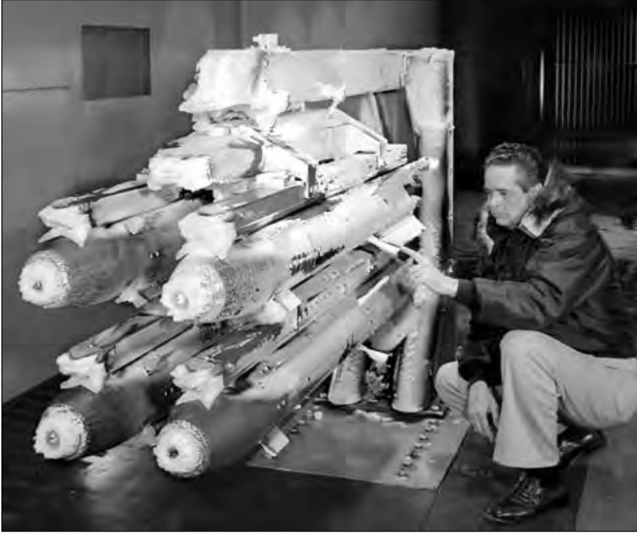
Figure 5-2. Rockwell factory representative inspects Hellfire missiles during IRT test, 1978. (NASA C-78-1039)
