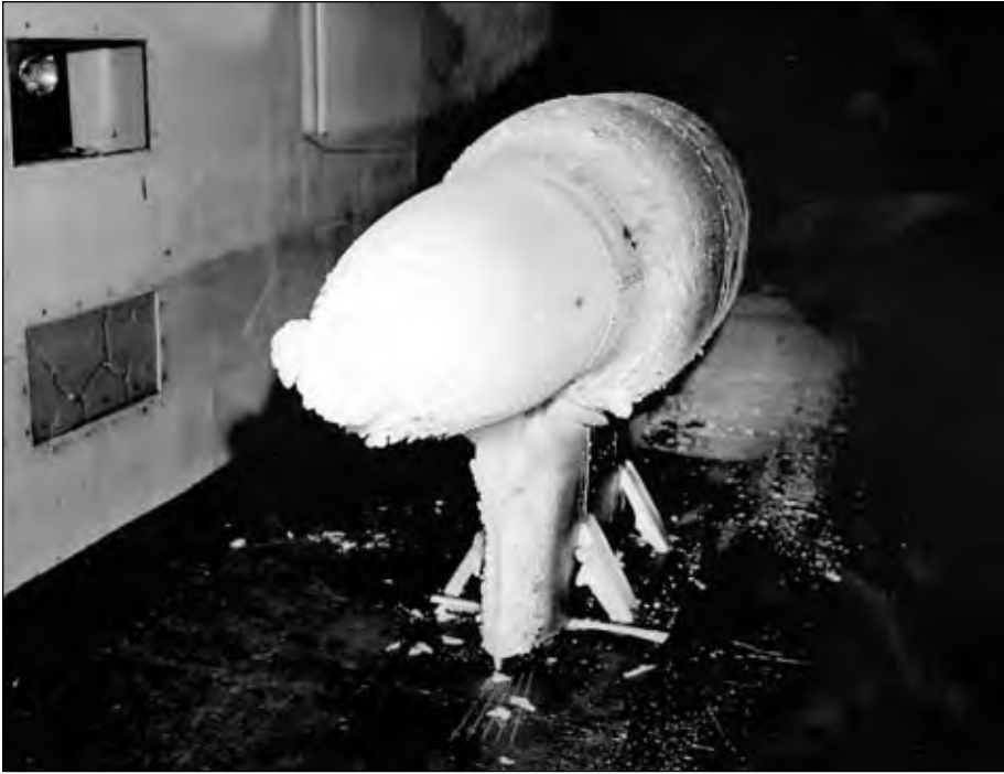
Figure 4-4. Unprotected propeller spinning after icing run, 1948. (NACA C-34635)
