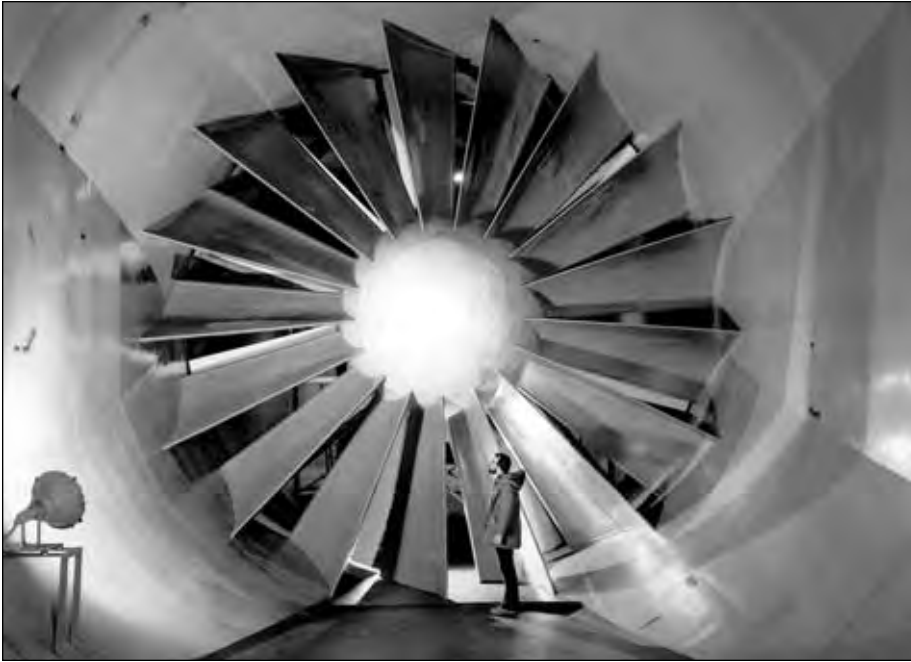
Figure 5-4. Inspecting IRT fan blades, 1979. (NASA C-79-324)
