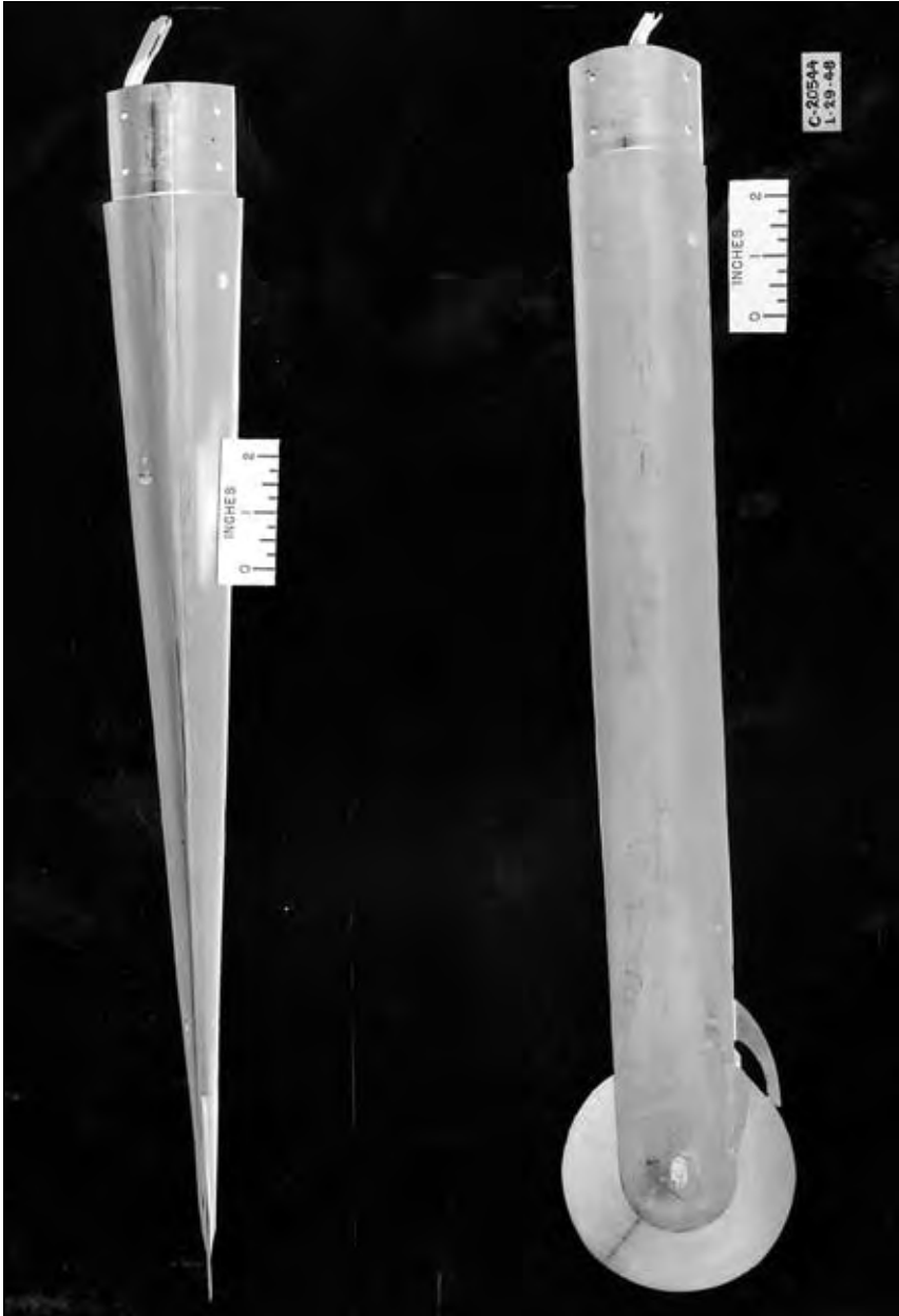
Figure 3-11. Rotating disk icing rate meter, 1948. (NACA C-20544)
