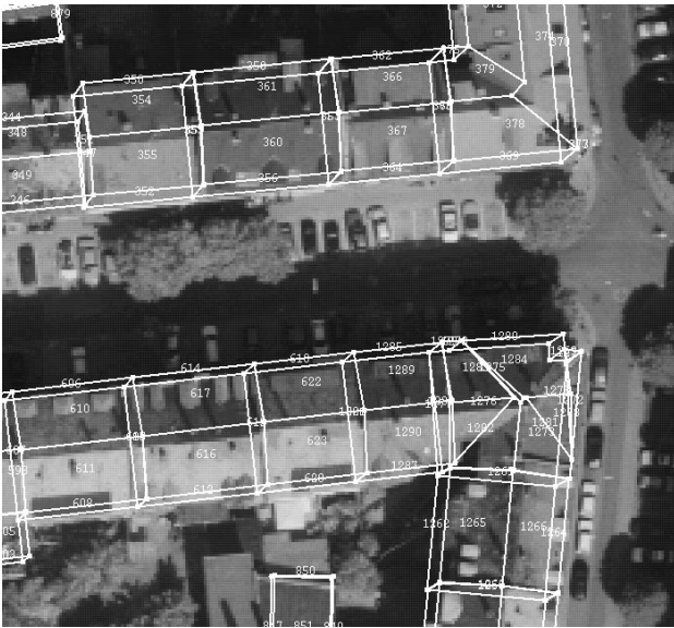
Figure 13: Reconstructed building projected into stereo image.
