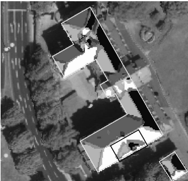
Figure 8: Segmented roof regions, original ground plan (white) and interactively added ground plan segment (black).
