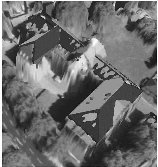
Figure 11: Reconstructed building and DSM surface.
