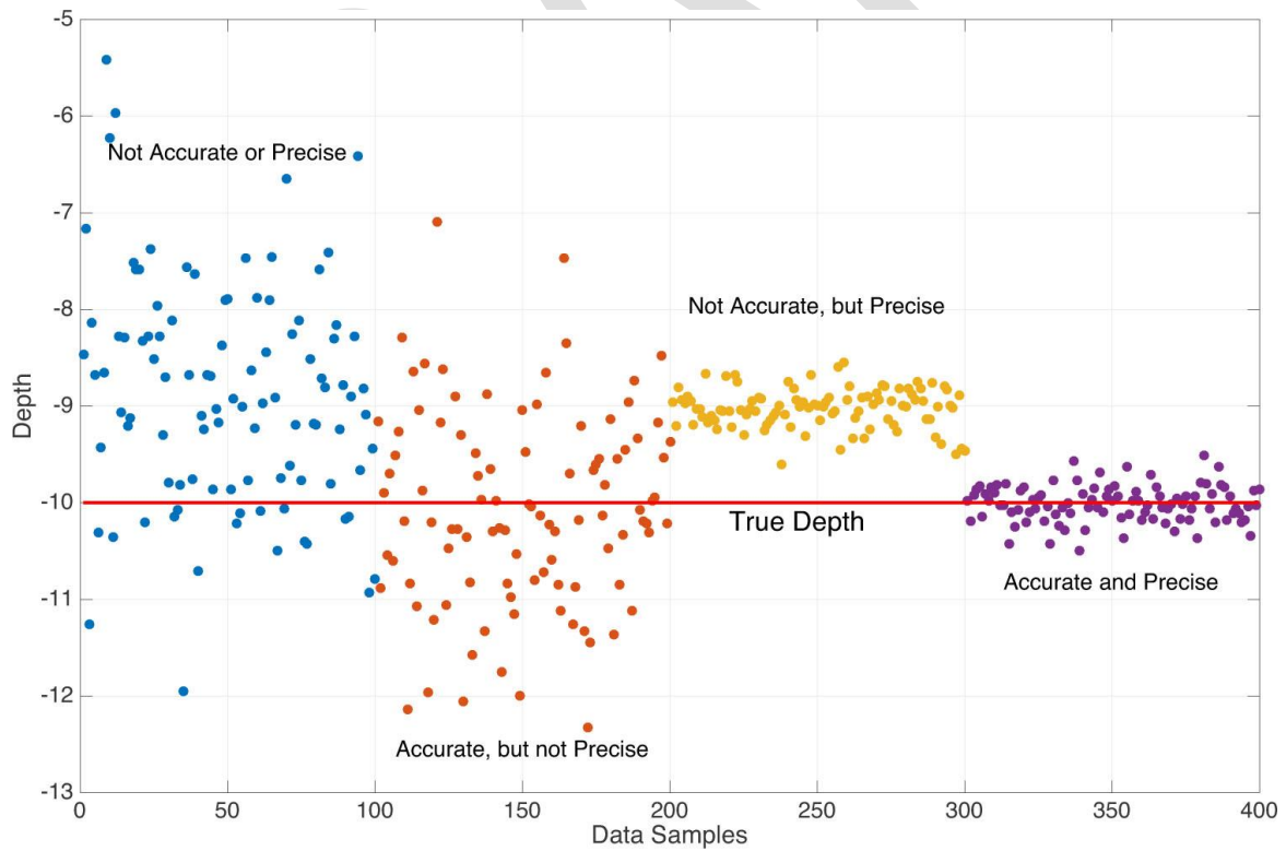
Figure 9. Example of depth measurements, from the four quadrants of Figure 8.
