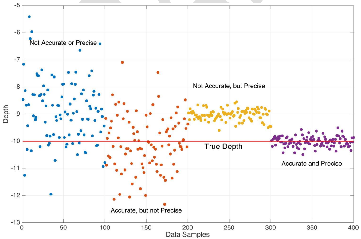
Figure 89. Example of depth measurements, from the four quadrants of Figure 78.
