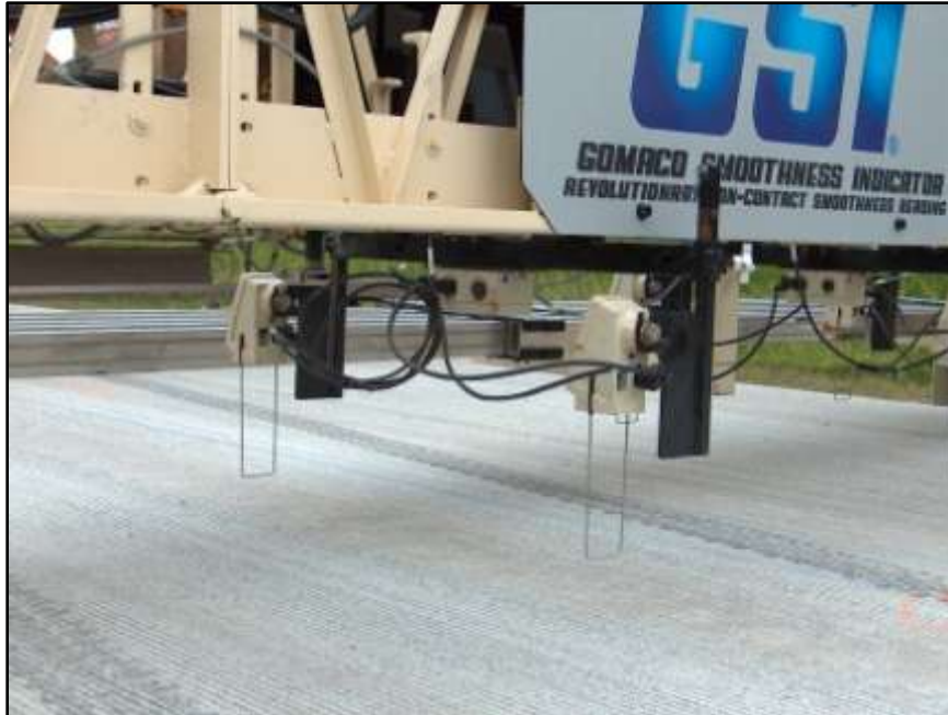
Figure 78 – Noncontact smoothness profile equipment (GOMACO)
