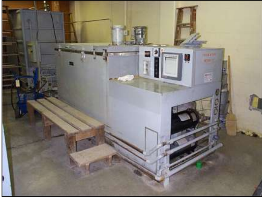
Figure 8 - Method "A" aggregate freeze-thaw equipment
