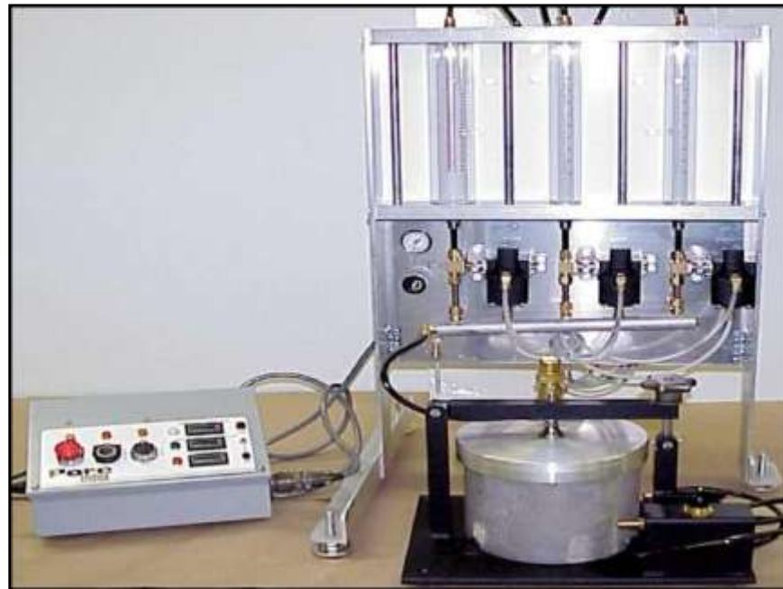
Figure 10 - Iowa Pore Index test equipment
