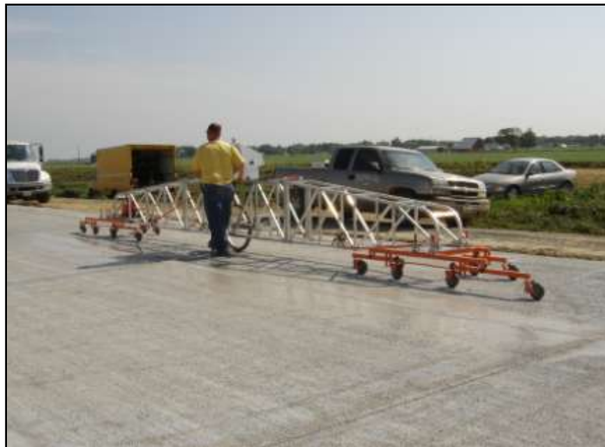
Figure 66 - 25 foot California type profilograph
