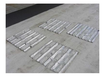
**Figure 8:** Solar Exposure of PETE Bottles: Bottles were exposed to sunlight on the roof of Kelley Engineering Center for 3 months. The bottles were place on corrugated PVC material wrapped in aluminum foil.
