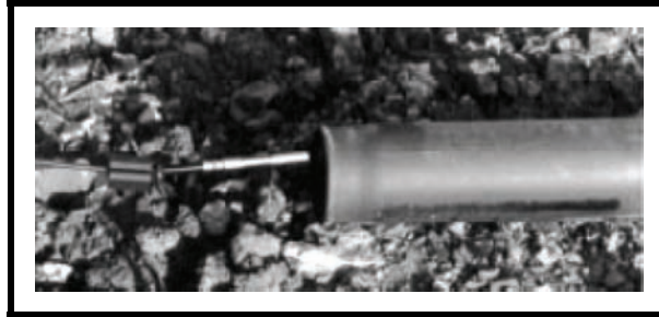
Figure 14-21. Priming of bangalore torpedo with MDI.
