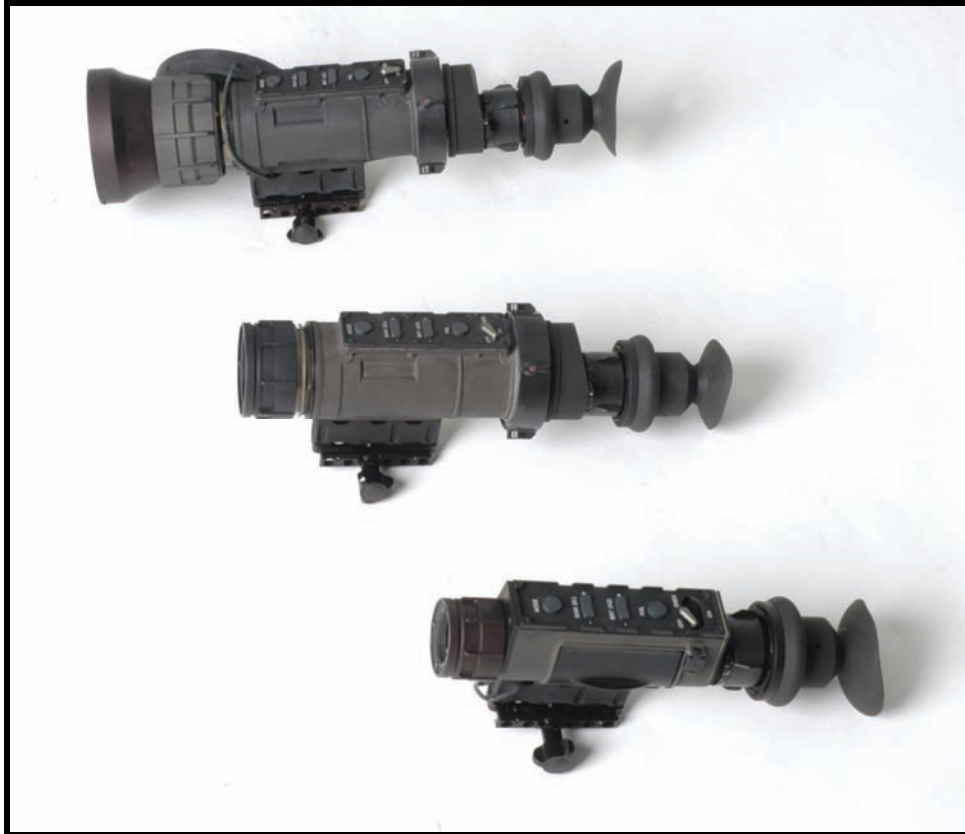
Figure 9-8. AN/PAS-13, V1, V2, and V3.
