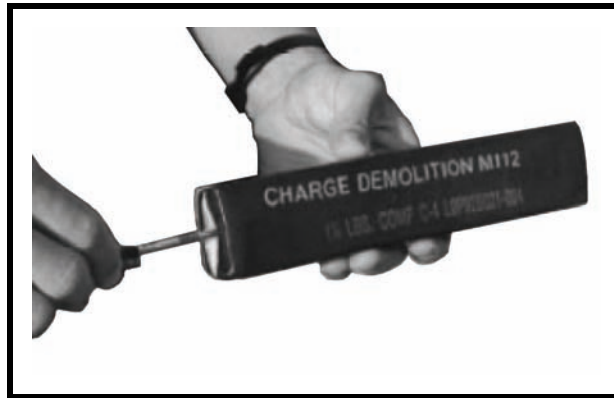
Figure 14-9. Priming of C4 demolition blocks with MDI.
