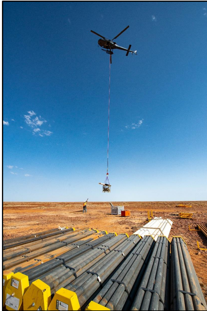
Figure 7 - Helicopter transporting heavy equipment from a laydown area on Andamooka Island to an 'offshore' drilling rig (courtesy of Applicant)
