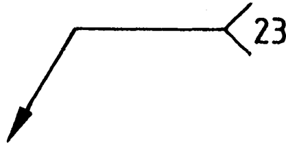
FIG. 18.11 INDICATION OF WELDING PROCESS
