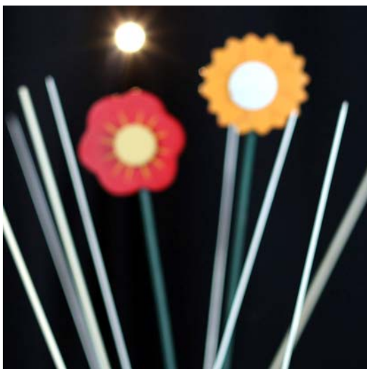
Test subject photographed slightly out of focus with the lens with 5 iris blades (see page 31)
