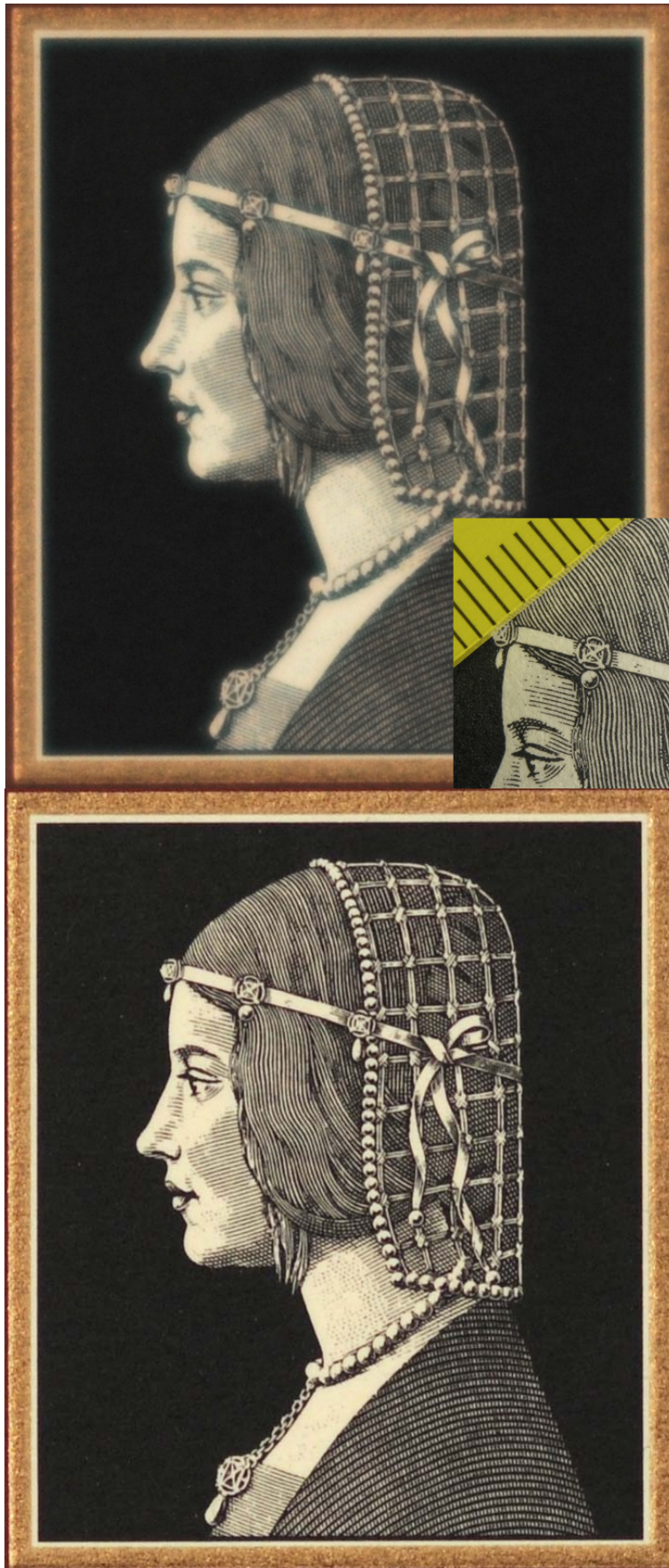
A 700x820 pixel crop from a 24MP-image, above with strong spherical aberration, below with good correction. The hatching in the hair is at about 40 Lp/mm on the sensor. Scale ratio was 1:10. These images are available as download files.
