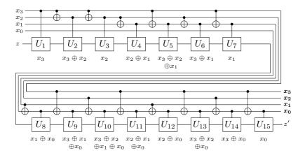
Figure 6.9. Extended Toffoli circuit with 4 mixed control units and without ancillary lines.
