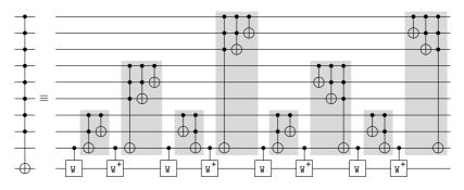
Figure 6.17. Application of the circuit from Figure 6.14 (b) to reduce quantum cost of the Toffoli gate with 8 control signals.
