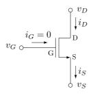
Figure 4.1. NMOS transistor with terminal labels, voltages, and currents.
