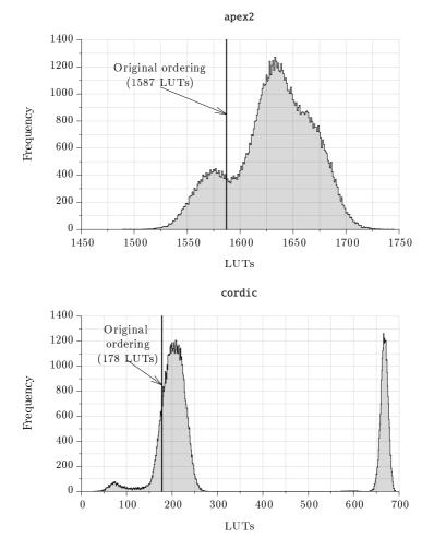
Figure 4.8. Distribution of solutions for the circuits apex2 and cordic.
