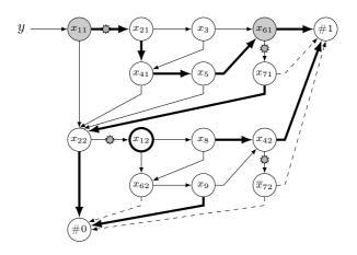
Figure 5.2. Structurally Synthesized BDD for the circuit in Figure 5.1.
