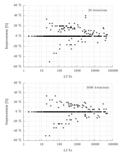
Figure 4.12. Delay improvements w.r.t the standard iterative process.
