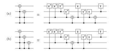
Figure 6.14. Reversible  $4 \times 4$  circuits mapped to optimal NCVW quantum circuits: (a) pair of 4-bit and 3-bit MCT gates, (b) additional CNOT gate.
