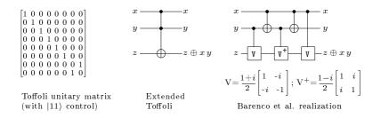
Figure 6.4. Unitary matrix, symbol, and quantum realization of the Toffoli gate.
