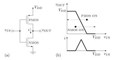
Figure 4.2. CMOS inverter: (a) circuit schematic, and (b) transfer characteristics.
