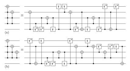
Figure 6.15. Optimal 5×5 NCV quantum circuits: (a) pair of 4-bit and 3-bit MCT gates, (b) Toffoli circuit from Figure 6.14 (b).
