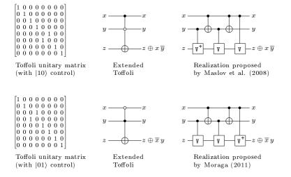
Figure 6.5. Toffoli gates with one negated control input.
