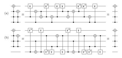
Figure 6.16. Best quantum circuits for the pair of 4-bit and 3-bit MCT gates: (a)  $4 \times 4$  NCVW, (b)  $5 \times 5$  NCV.
