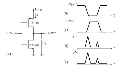
Figure 4.3. Power consumption waveforms: (a) CMOS inverter with load capacitance  $C_L$ , (b) input  $v_{IN}$ , (c) corresponding output  $v_{OUT}$ , (d) current *i* drawn from power supply, and (e) total instantaneous power.
