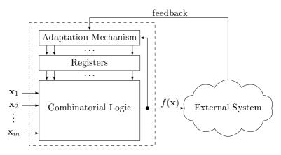
Figure 5.11. The architecture of a WbAH system.
